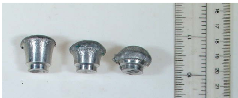
Deformed aluminum projectiles after plate perforation.
