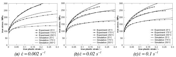
Figure 1: Experimental [5] and LS-Dyna simulation results of the uniaxial tension test
