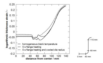
Figure 3: Thickness distribution results for different process layouts at 250  $^{\circ}$  flange temperature and 20 mm/s punch velocity
