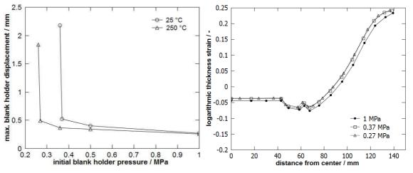
(a) Maximum blankholder displacement dependent on initial blank holder pressure
