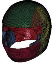
Figure 1: FE model of a commercial full-face helmet
