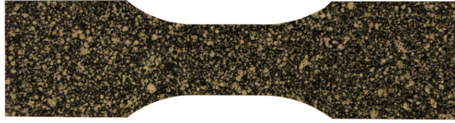
Figure 4: Tensile bar with grey scale pattern
