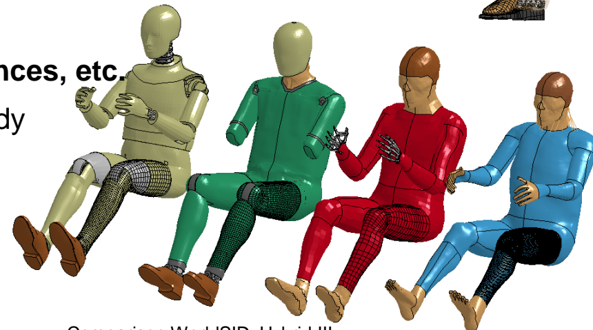
Comparison WorldSID, Hybrid III, THUMS V3, THUMS V4
