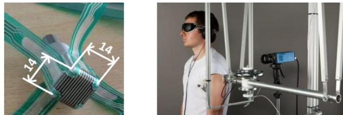
Fig. 1: Available impactor with impact surface 14mmx14mm (left) and the mechanical pendulum for examining verified limit values of dynamic contacts (right) [2].
