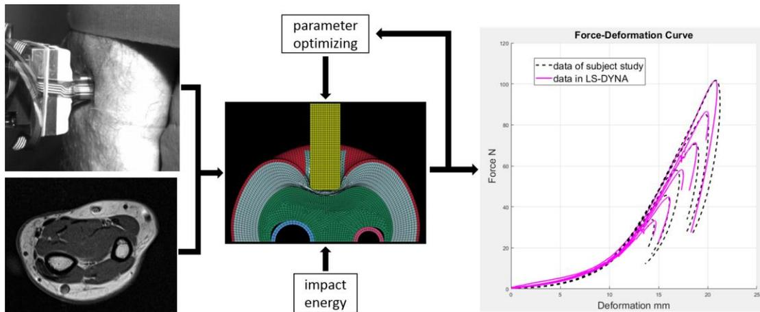
Fig. 3: Development of FE-simulation for the impact on tissue model in LS-DYNA, e.g. model for lower arm muscle with the impact energy from 0.23J to 0.48J and the impact mass 5.8kg.
