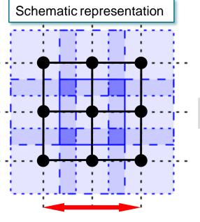
Reference length of the strain calculation
