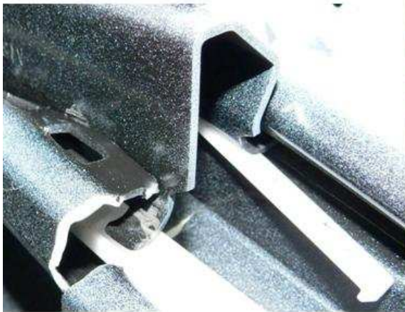
Design A : Rupture of the female profile
