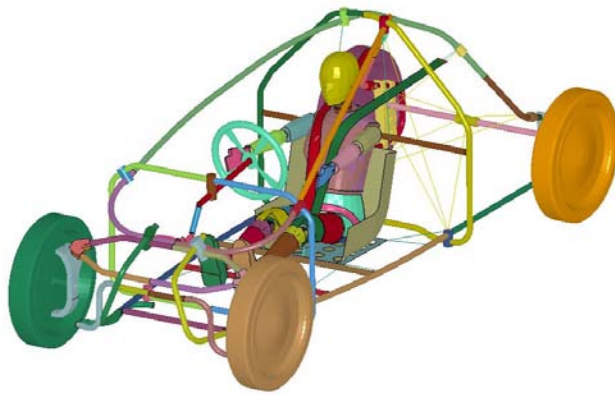
Figure 19: FE-Model of the Schluckspecht CityE2light
