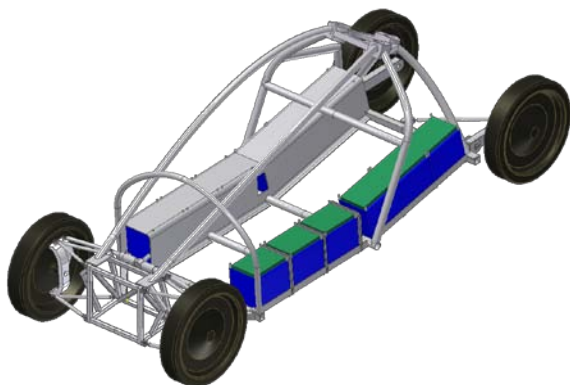
Figure 17: CAD-model of the Schluckspecht E structure with two battery packs
