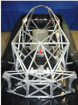
Figure 3: Schluckspecht City 2009 aluminum space frame
