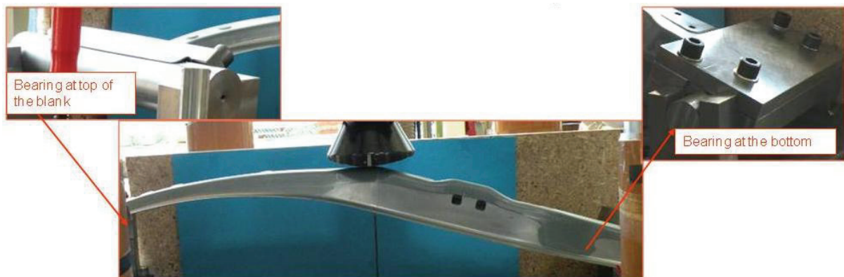
Figure 14: Experimental set-up of the tension-bending test on ZStE340 metal blank of a b-pillar.
