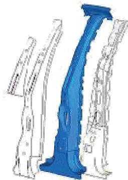
Figure 1: Part of the B-pillar considered for experiments and simulations: ZStE340 metal blank.
