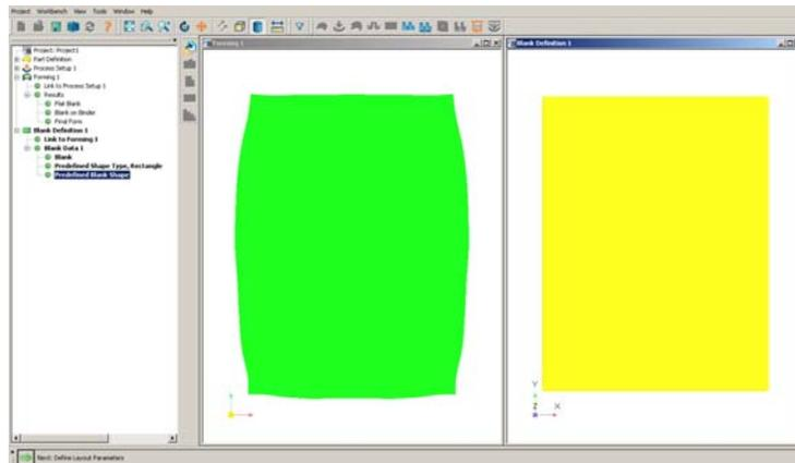
Figure 2: Nesting capabilities for definition of process blank
