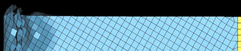
Fig 3a. Final deformed shape of square tube impacting the wall @ 5mph
