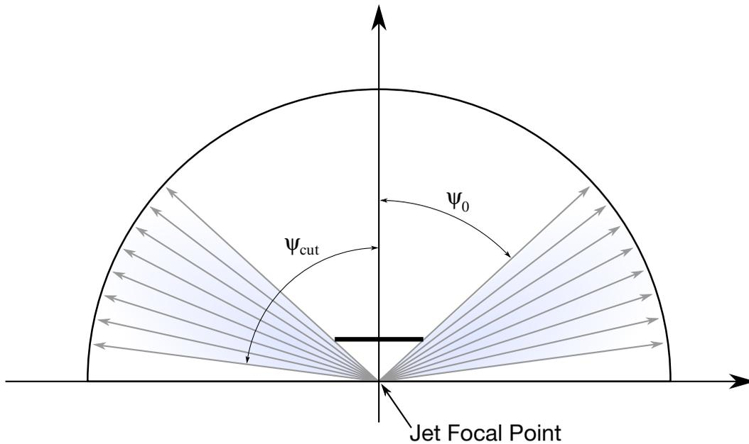
**Figure 3-4.** Multiple jet model for driver's side airbag. Typically,  $\psi_{\text{cut}}$  (see input ANGLE) is close to  $90^\circ$ . The angle  $\psi_0$  is included to indicate that there is some angle below which the jet is negligible; see [Figure 3-3](#).
