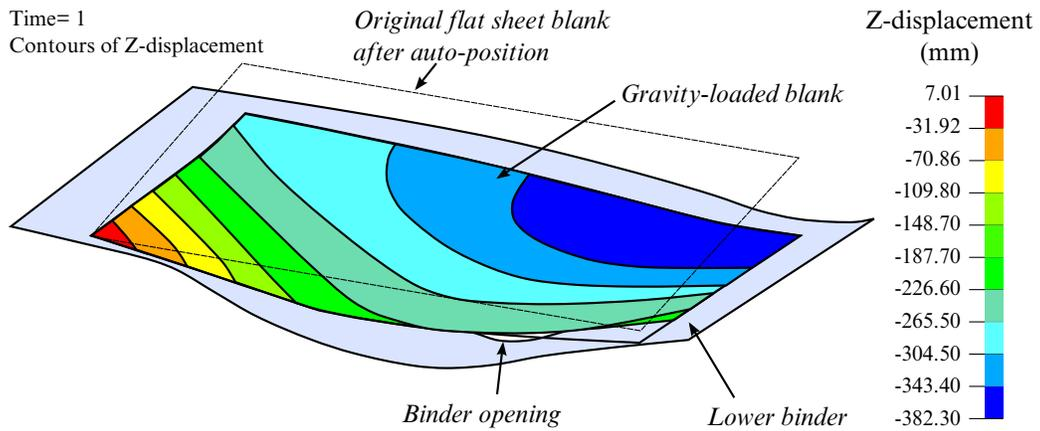
**Figure 12-54.** Gravity loading on a box side outer toggle die (courtesy of Autodie, LLC).
