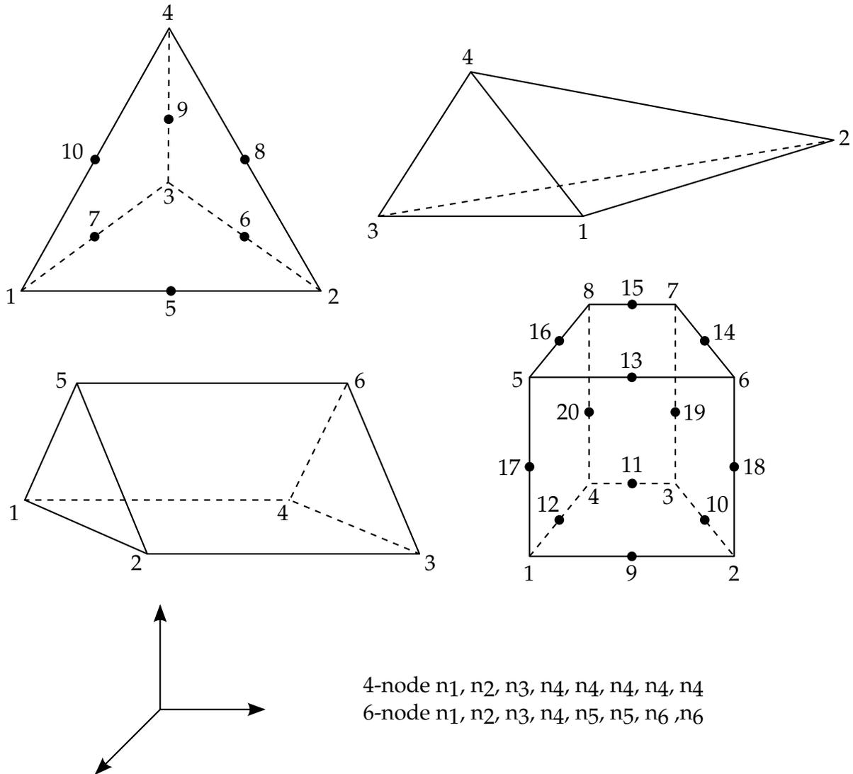
**Figure 18-28.** Four, six, and eight node solid elements. Nodes 1-4 are on the bottom surface.
