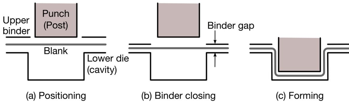
**Figure 12-43.** IDTEMP = 2: forming in 3-piece toggle draw.
