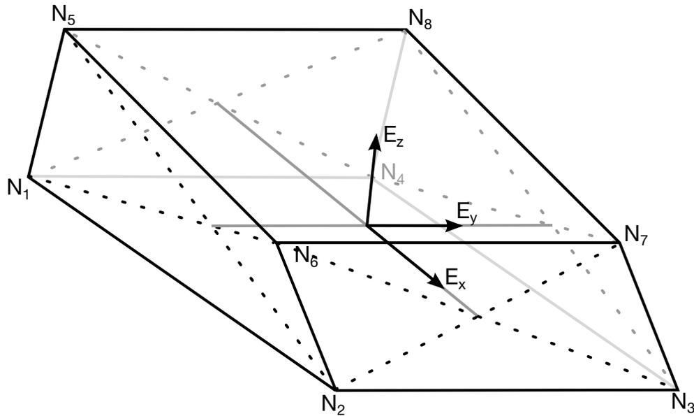
**Figure 10-32.** The  $E_x$  direction is aligned along the line segment connecting the centers of the 2-3-6-7 and the 1-4-8-5 faces. The  $E_y$  direction is orthogonal to the  $E_x$  direction and in the plane containing both  $E_x$  and containing the segment connecting the centers of the 1-2-6-5 and 3-4-8-7 faces. The  $E_z$  is normal to this plane.
