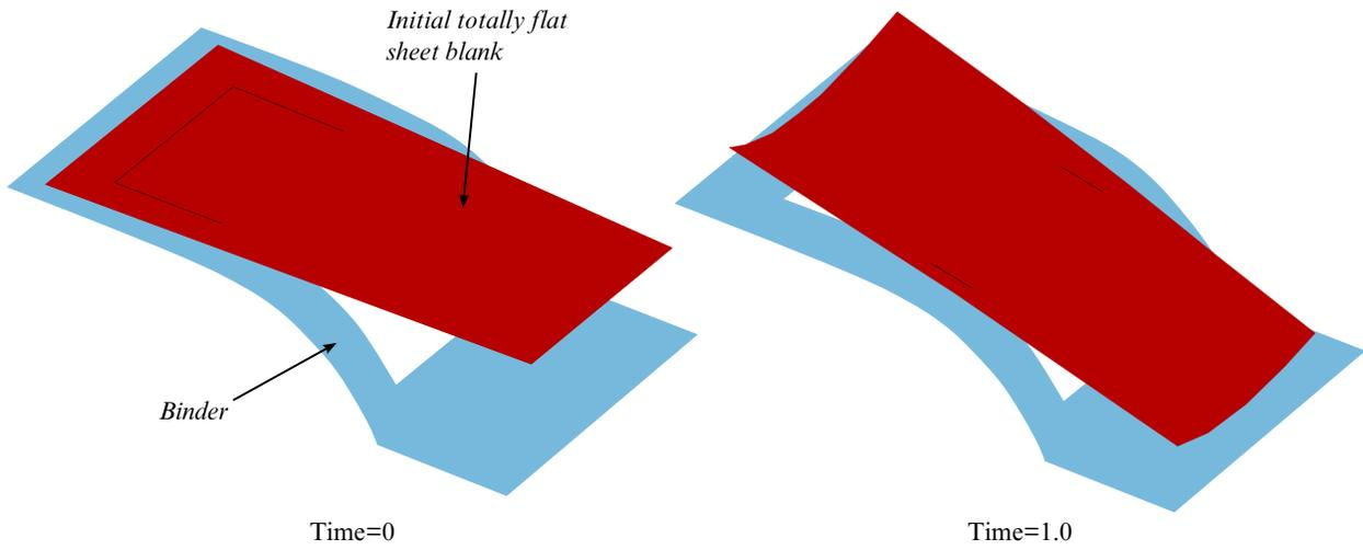
**Figure 12-66.** Test model (left) and gravity loaded blank (right) with switching from implicit dynamic to implicit static.
