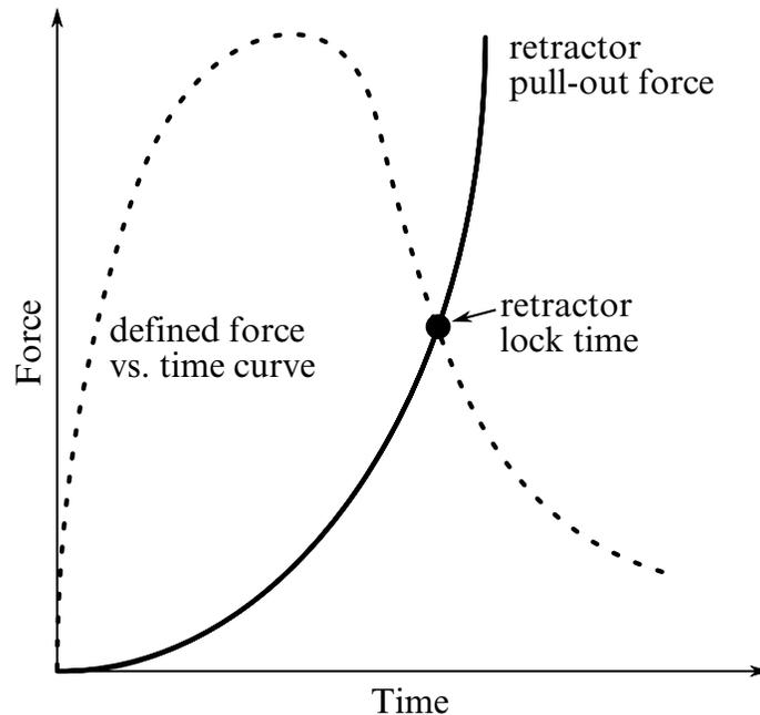
**Figure 18-15** Force versus time pretensioner. At the intersection, the retractor locks.
