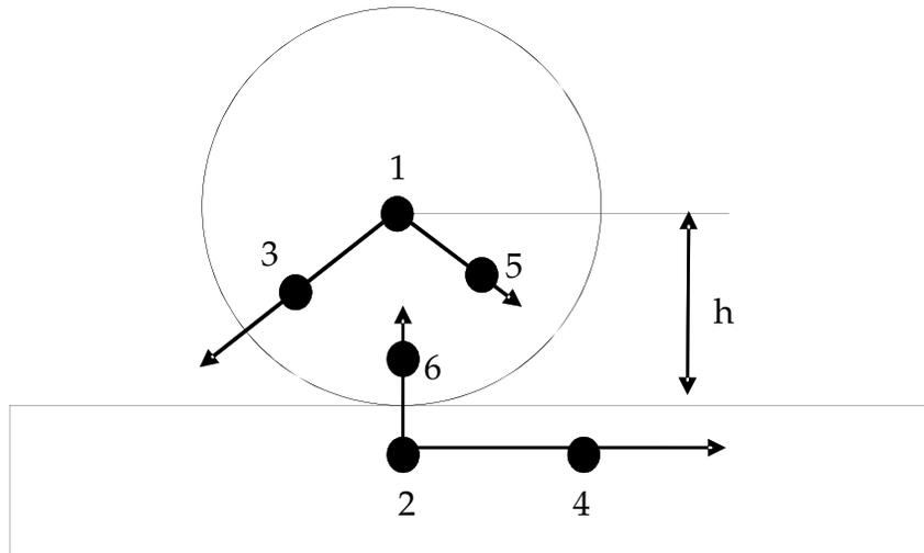
**Figure 10-23.** Rack and pinion joint. Nodal pair (1, 3) defines the axis of rotation of the first body (the pinion). Nodal pair (1, 5) is a vector in the plane of the pinion and is orthogonal to nodal pair (1, 3). Nodal pair (2, 4) defines the direction of travel for the second body (the rack). Nodal pair (2, 6) is parallel to the axis of the pinion and is thus parallel to nodal pair (1, 3). The value  $h$  is specified. The velocity of the rack is  $h\omega_{\text{pinion}}$ .
