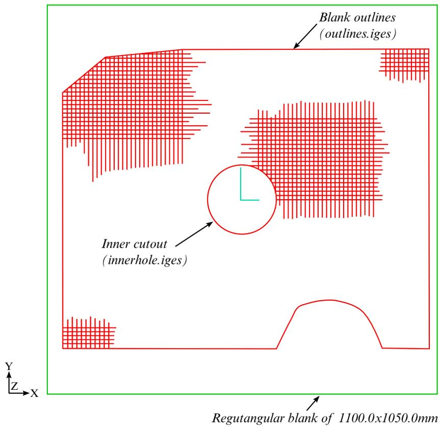
**Figure 15-33.** Initial input for a blank meshing.
