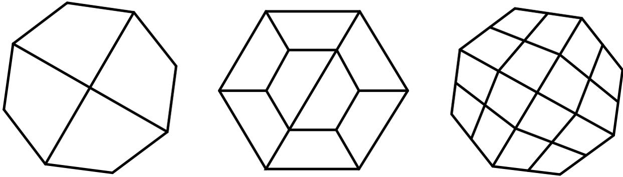
**Figure 15-42.** Sample four, eight, and sixteen element spot weld clusters comprised of solid hexahedron elements.
