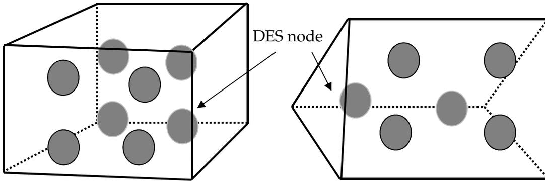
Example of discrete element sphere nodes for hexahedron element with  $NQ = 2$
