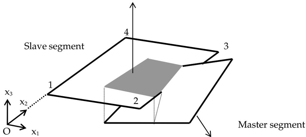
**Figure 11-16.** Illustration of Mortar segment to segment contact
