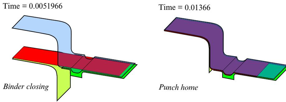
**Figure 12-24.** An air draw example with closing and drawing.
