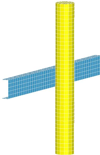
**Figure 45-3.** Impact between a user-defined shell and user-defined solid part.
