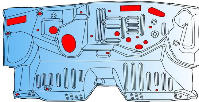
**Figure 12-14.** A trimmed dash panel (firewall) with holes auto-filled using LS-PrePost 4.0 (original model courtesy of NCAC Taurus crash model).
