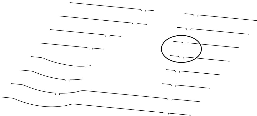
**Figure 25-35.** Multiple sections cut on the lower binder.
