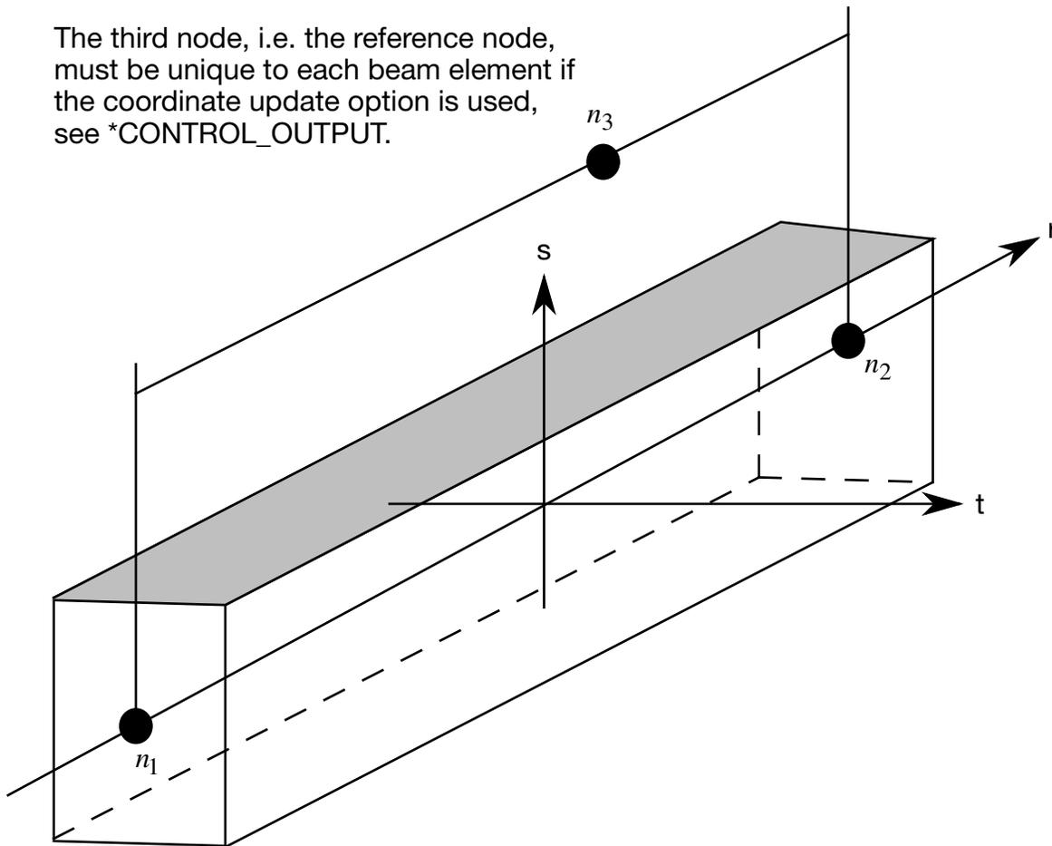
**Figure 18-1.** LS-DYNA beam elements. Node  $n_3$  determines the initial orientation of the cross section.
