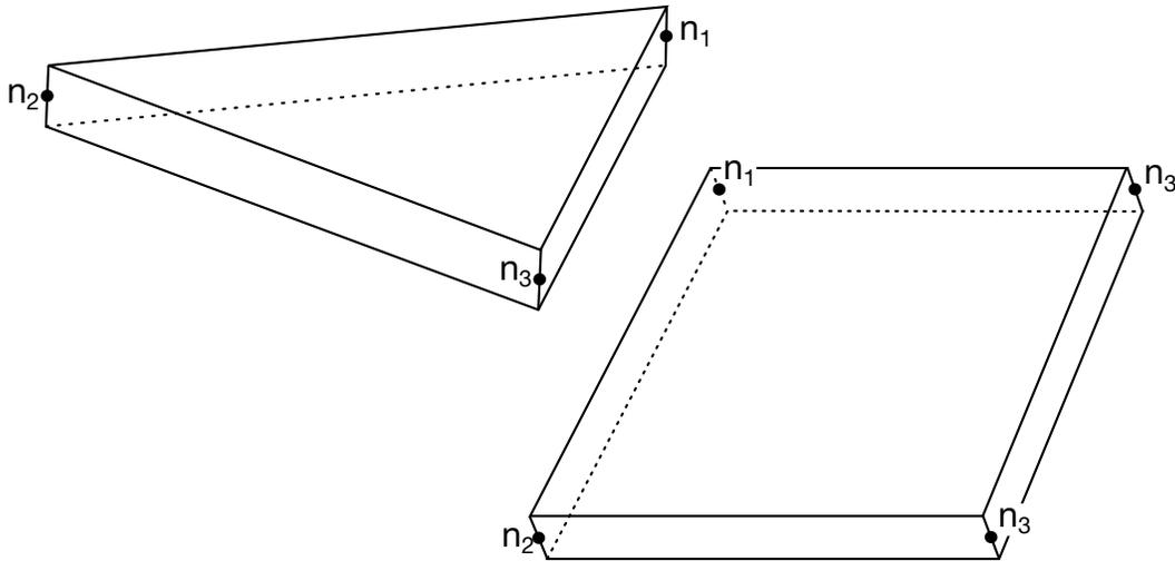
**Figure 18-23.** LS-DYNA shell elements. Counterclockwise node numbering determines the top surface.
