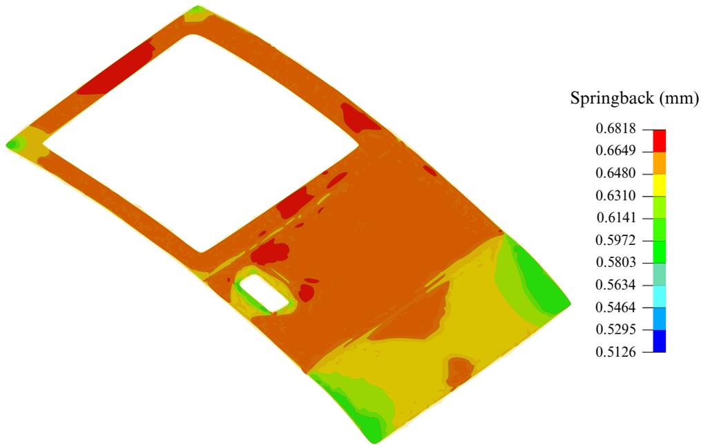
Figure 12-39. Springback amount (mm).
