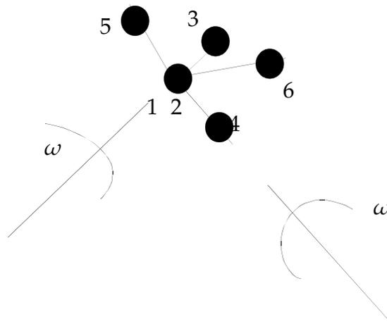
**Figure 10-24.** Constant velocity joint. Nodal pairs (1, 3) and (2, 4) define an axes for the constant angular velocity, and nodal pairs (1, 5) are orthogonal vectors. Here nodal points 1 and 2 must be coincident.
