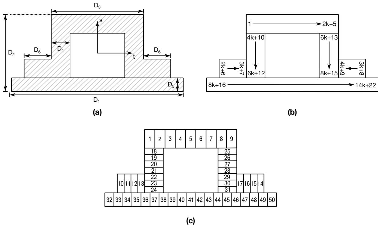
**Figure 24-24.** Type 22: Hat-Shaped 2. (a) Cross section geometry. (b) Integration point numbering. (c) Example for  $k = 2$ .
