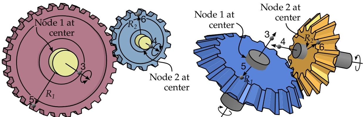
**Figure 10-22.** Gear joints. Nodal pairs (1, 3) and (2, 4) define axes that are orthogonal to the gears. Nodal pairs (1, 5) and (2, 6) define vectors in the plane of the gears. The ratio  $R_2/R_1$  is specified but need not necessarily correspond to the geometry, if for instance the gear consists of spiral grooves. Note that the gear joint in itself does not maintain the contact point but this requires additional treatment, such as accompanying it with other joints.
