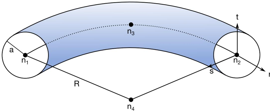
**Figure 18-2.** LS-DYNA Elbow element. Node n4 is the control node and is given as the beam center of curvature.
