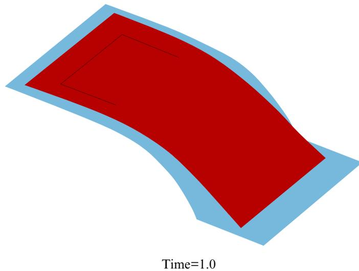
**Figure 12-67.** Gravity loaded blank without the “switching”.
