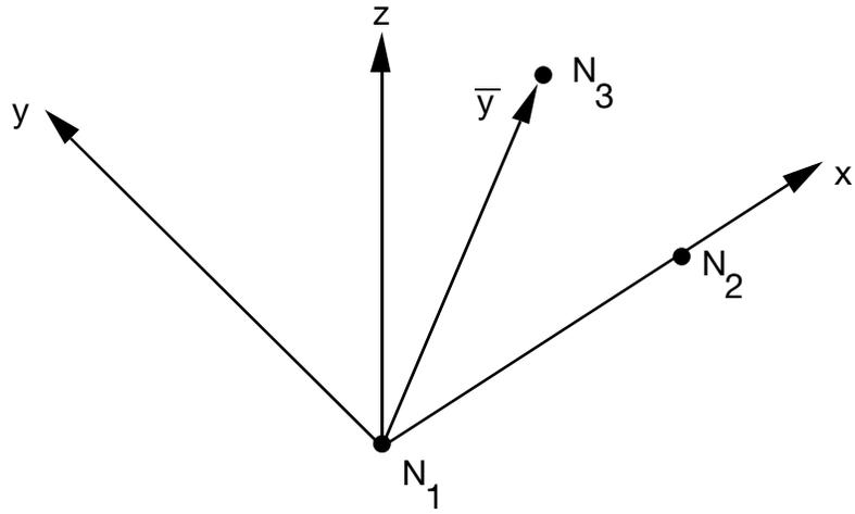
**Figure 15-1.** Definition of local coordinate system using three nodes when the node N2 lies along the x-axis.
