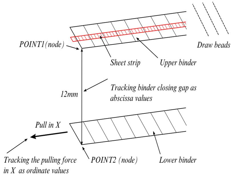
**Figure 11-7.** Tracking the closing gap and pulling distance.
