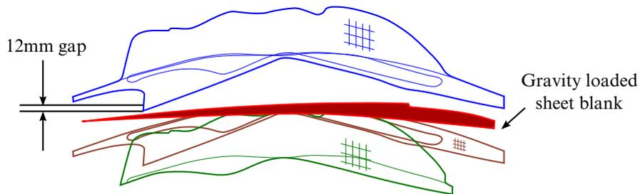
**Figure 11-19.** Gravity loading on blank at  $t = 0.2$ .
