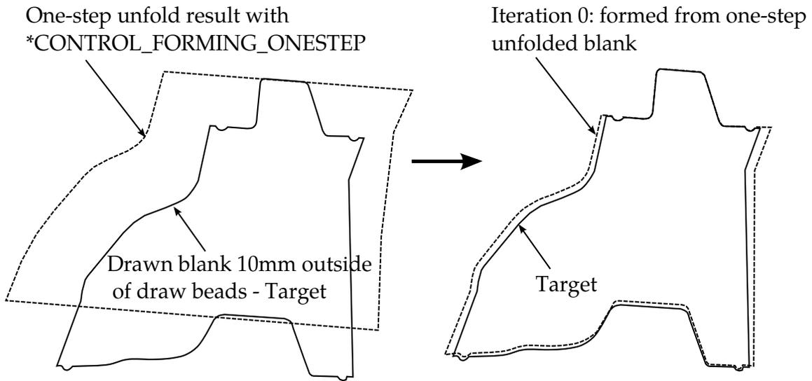
**Figure 25-12.** Initial blank calculation and baseline formed blank.
