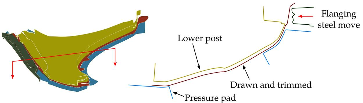
Figure 25-18. The flanging process on NUMISHEET 2002 fender outer.
