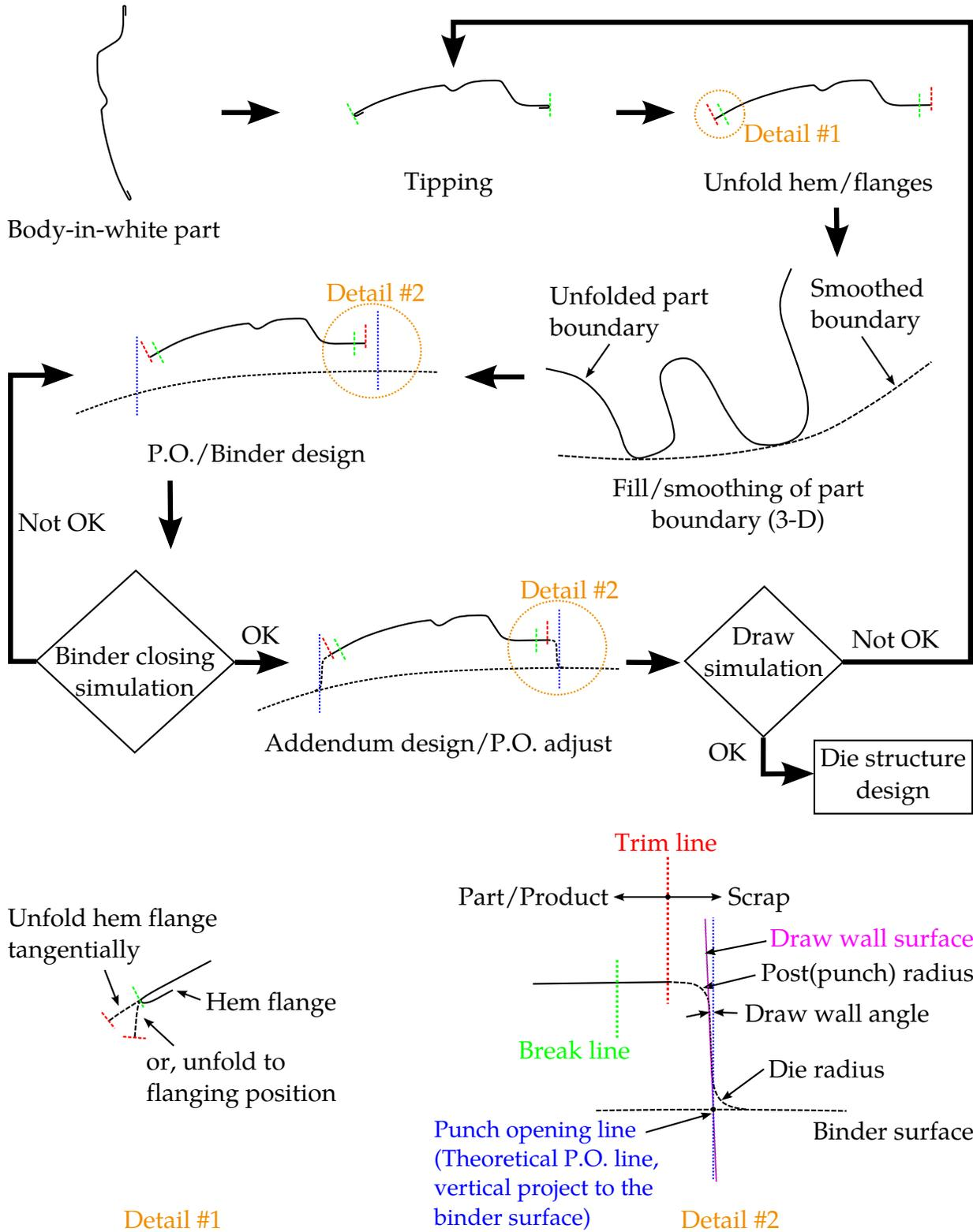
**Figure 62-1.** A typical draw die engineering process
