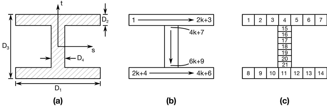
**Figure 24-3.** Type 1: I-Shape. (a) Cross section geometry. (b) Integration point numbering. (c) Example for  $k = 2$ .
