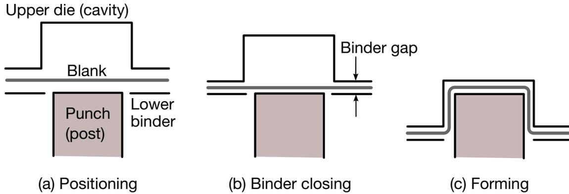
**Figure 12-42.** IDTEMP = 1: forming in 3-piece air draw.
