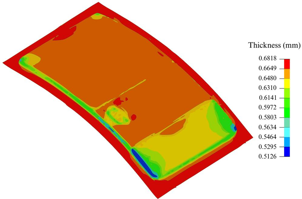
Figure 12-37. Thickness contour of the panel after draw simulation.
