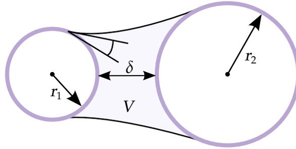
Figure 12-5. Schematic representation of capillary force model.
