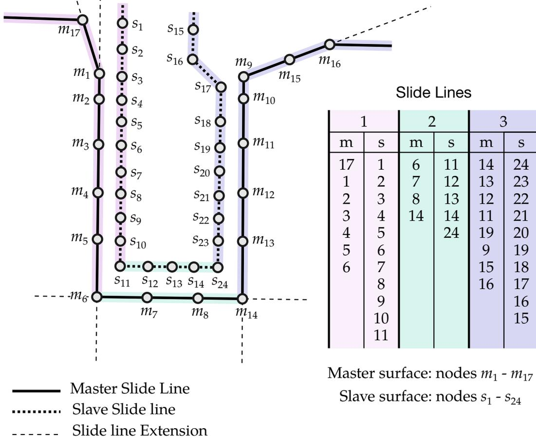
**Figure 11-26. Slide line Example.** Note: (1) as recommend, for 90° angles each facet is assigned a distinct slide line; (2) the master slide line is more coarsely meshed; (3) the slave is to the left of the master (following the node ordering, see inset table); (4) as shown for slave nodes 1 and 2 it is important the slide line extension does not spuriously come into contact.
