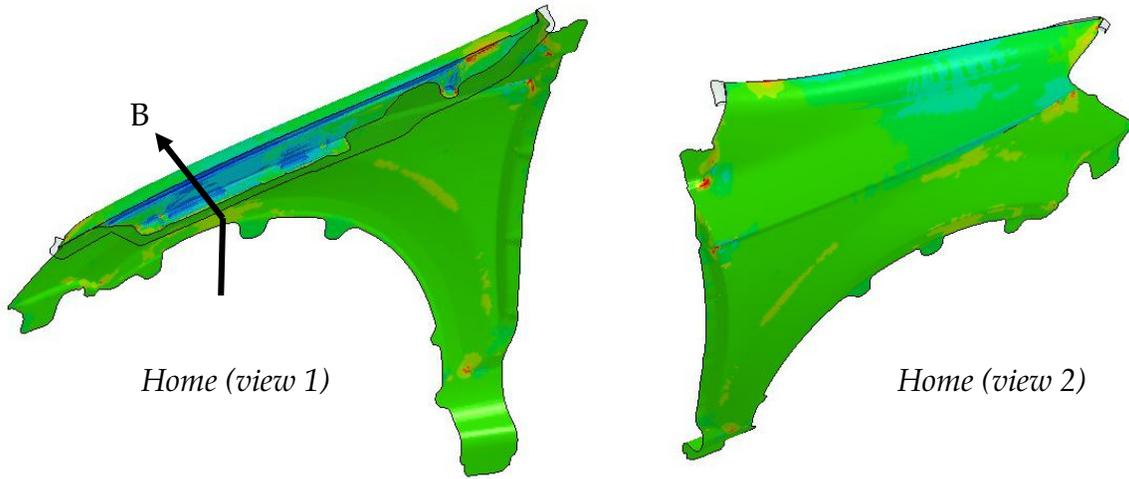
Figure 12-62. Mean stress at flanging home (compression/surface lows in red).
