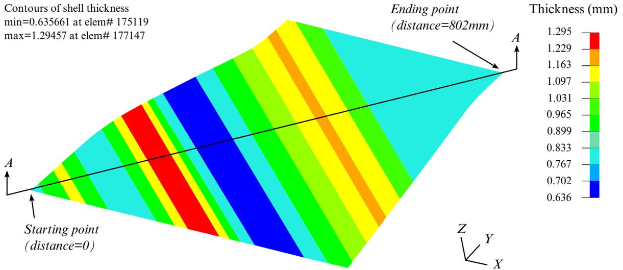
Figure 12-12. Define a varying thickness field across the sheet blank.
