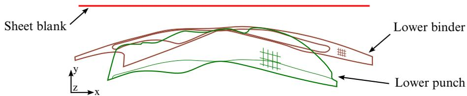
**Figure 12-28.** Initial model before auto-positioning.
