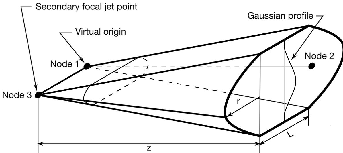
**Figure 3-2.** Jetting configuration for the passenger's side bag.
