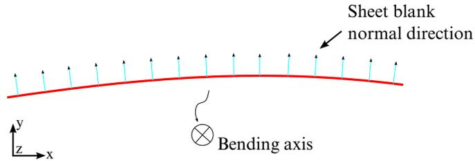
**Figure 12-27.** Negative "R" puts center of bending on the opposite side of the positive blank normal.
