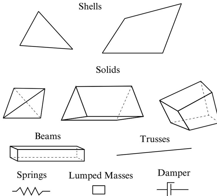
**Figure 1-1.** Elements in LS-DYNA. Three-dimensional plane stress constitutive subroutines are implemented for the shell elements which iteratively update the stress tensor such that the stress component normal to the shell midsurface is zero. An iterative update is necessary to accurately determine the normal strain component which is necessary to predict thinning. One constitutive evaluation is made for each integration point through the shell thickness.
