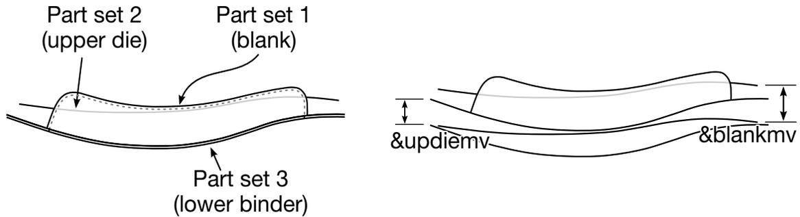
Figure 12-11. An example of binder closing in air draw
