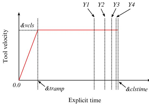
**Figure 12-23.** Specifying d3plot/intfor output at specific distances to punch home.
