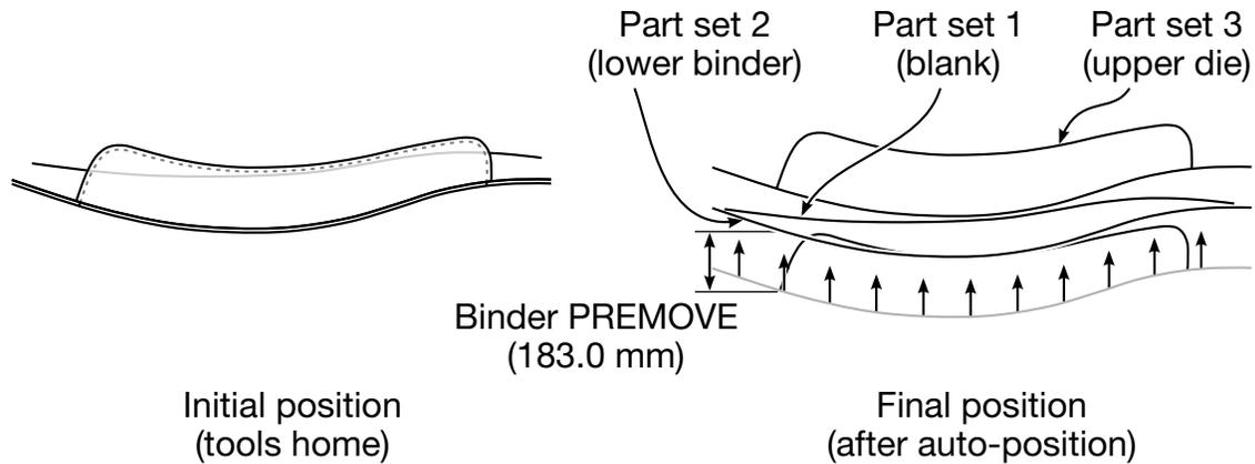
**Figure 12-10.** An example of using the variable PREMOVE
