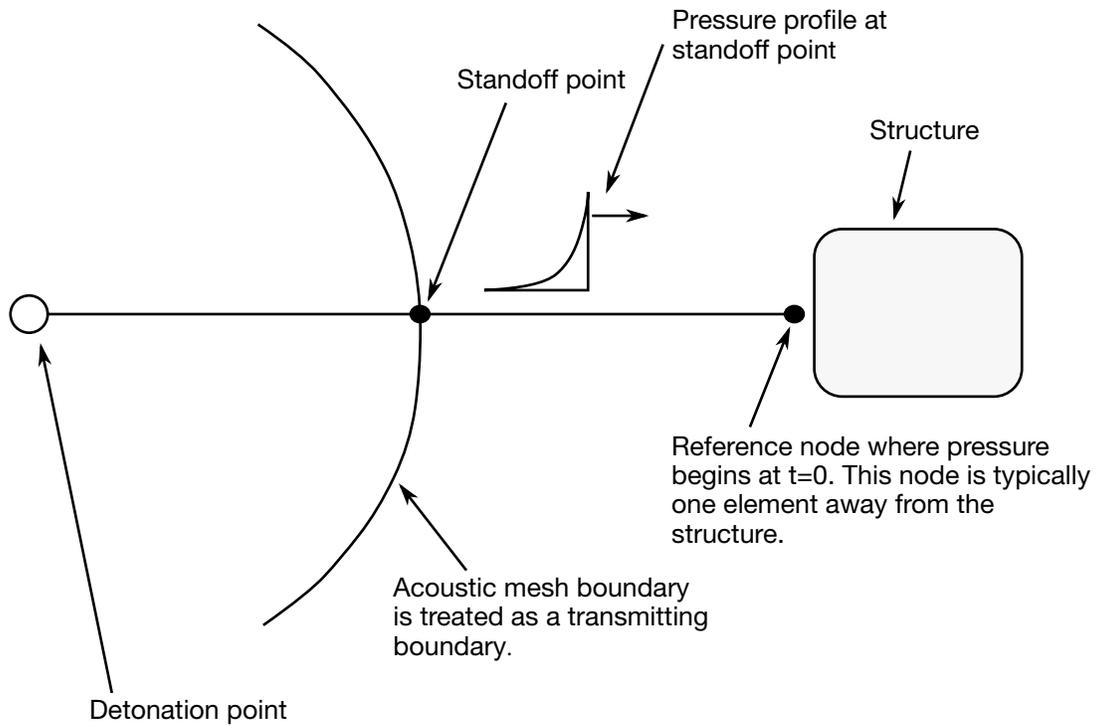
**Figure 23-1.** Initialization of the initial pressures due to an explosive disturbance is performed in the acoustic media. LS-DYNA automatically determines the acoustic mesh boundary and applies the pressure time history to the boundary. This option is only applicable to the acoustic element formulation, see \*SECTION\_SOLID.
