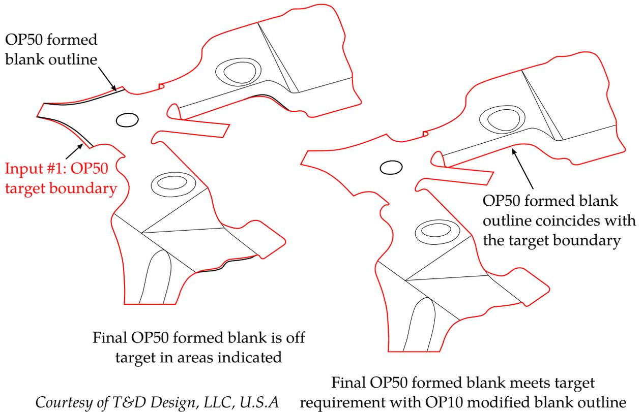
**Figure 25-24.** Verification simulation on the progressive die process.
