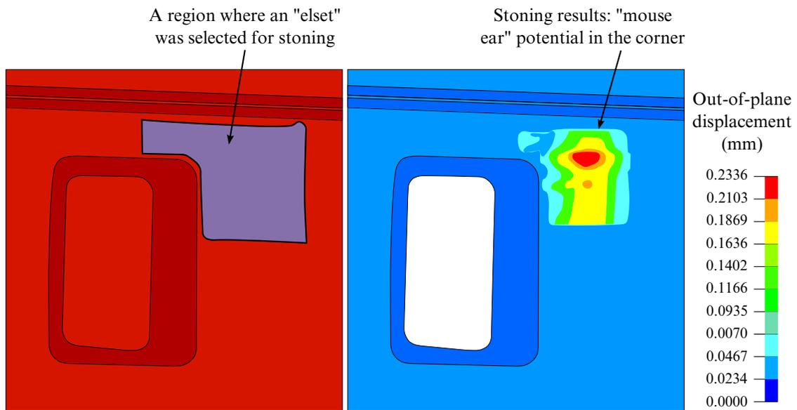
Figure 12-40. Stoning simulation for the upper right door corner.
