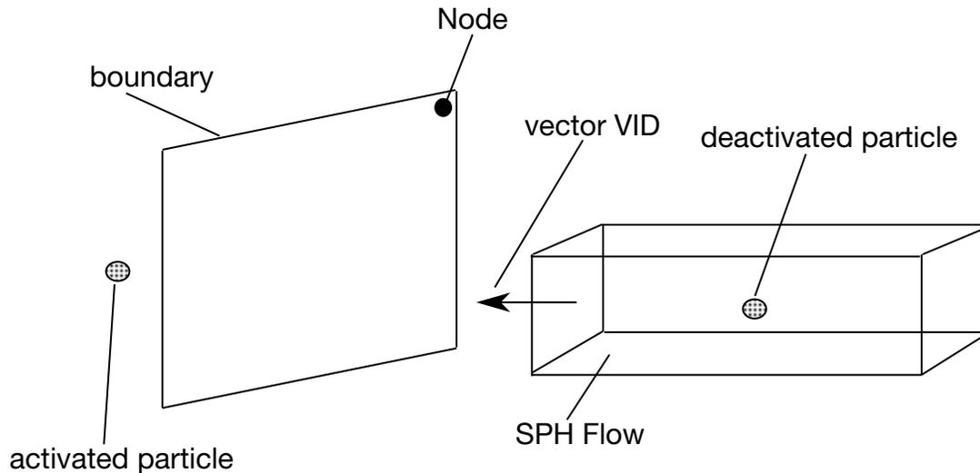
**Figure 5-5.** Vector VID determines the orientation of the SPH flow
