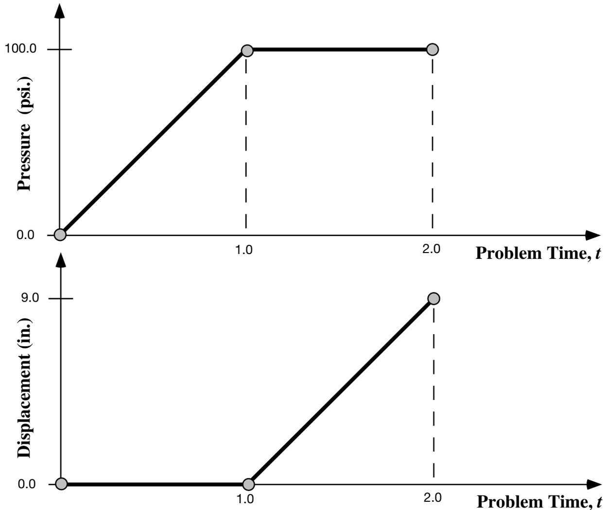
Load curves for a static simulation with two loading events. For convenience in this static simulation, the pressure loading is specified to begin at time 0.0 and end at time 1.0, and the displacement begins at time 1.0 and ends at time 2.0.
