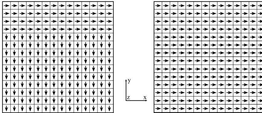
**Figure 15-39.** Element directions (N1-N2) of an incoming sheet blank (left) and directions after re-orientation.
