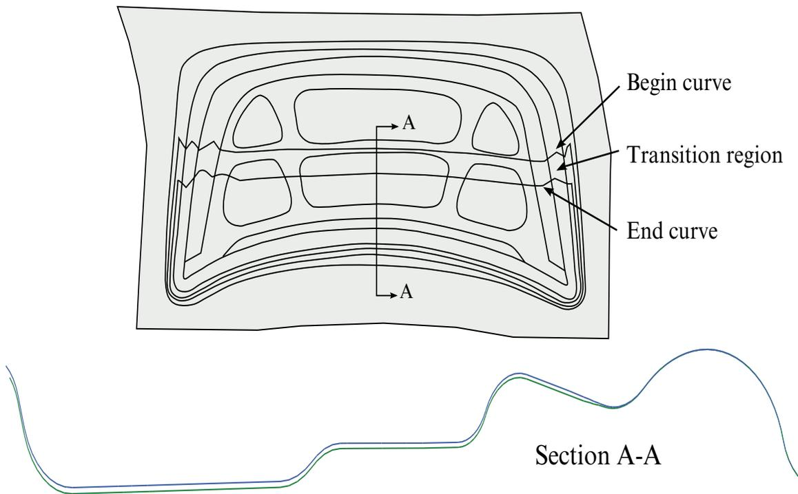
Figure 25-30. Two curves defining a localized area of a decklid inner.
