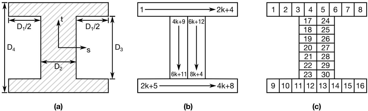
**Figure 24-17.** Type 15: I-Shape 2. (a) Cross section geometry. (b) Integration point numbering. (c) Example for  $k = 2$ .
