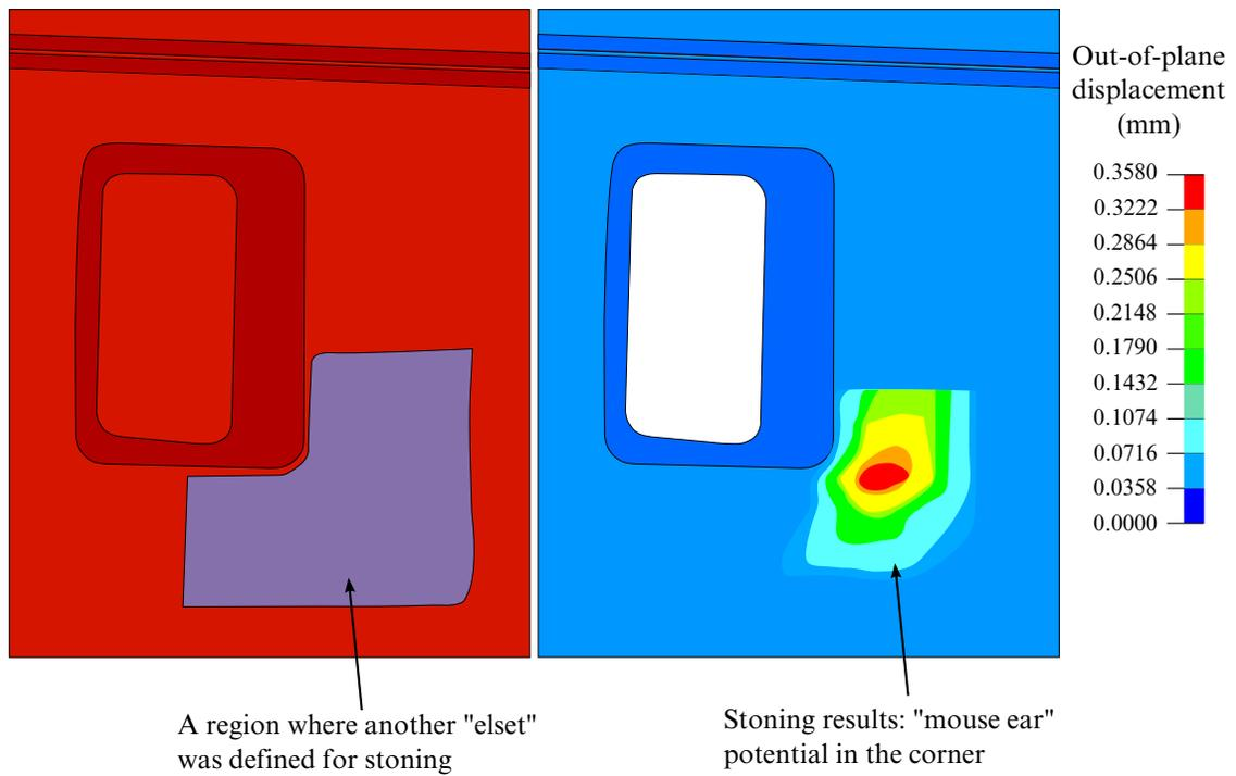
**Figure 12-41.** Stoning simulation for the lower right door corner.
