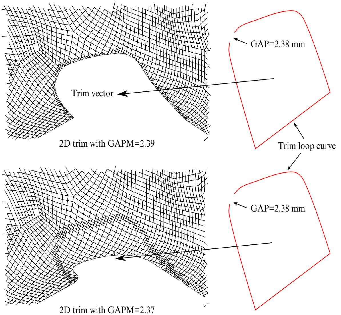
Figure 12-46. A 2D trimming with different GAPM values.
