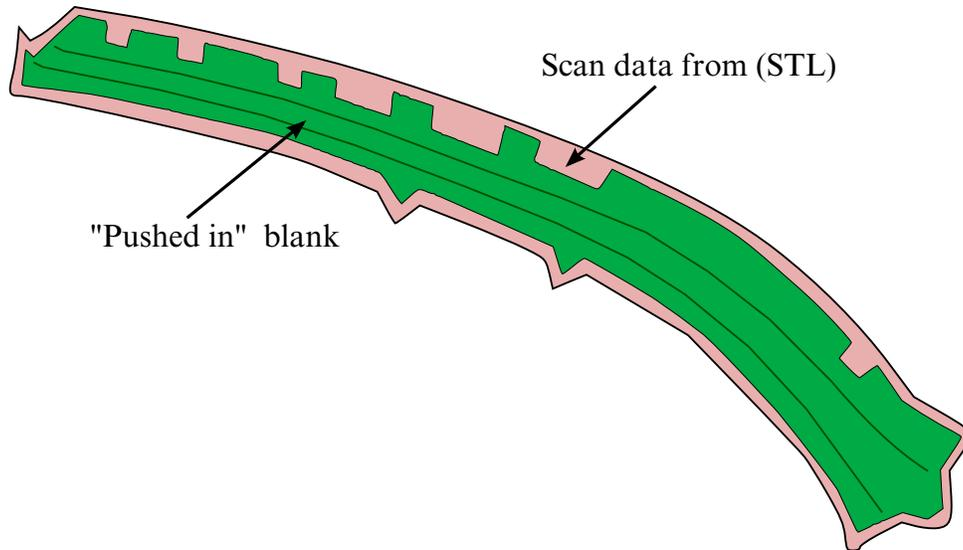
**Figure 25-28.** A trimmed panel “pushed” onto the scan data (rigid body).
