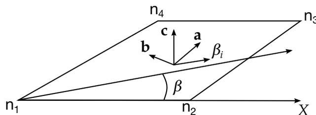
**Figure 18-25.** Orientation of material directions (shown relative to the 1-2 side as when AOPT = 0 in \*MAT).
