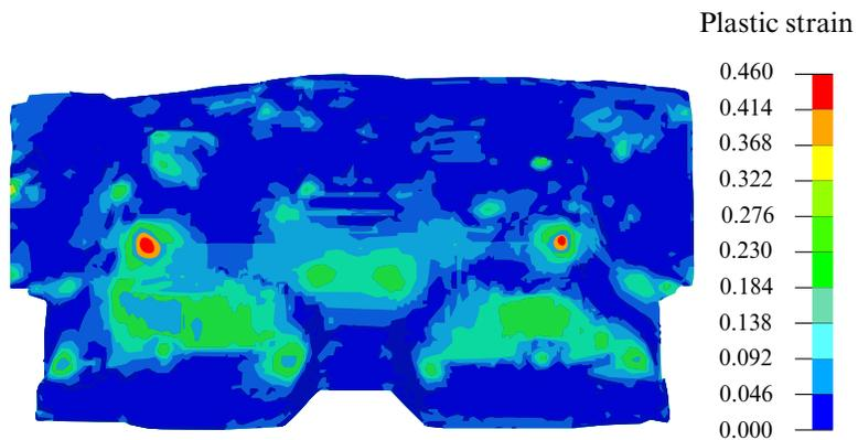
**Figure 12-16.** Effective plastic strain Prediction.
