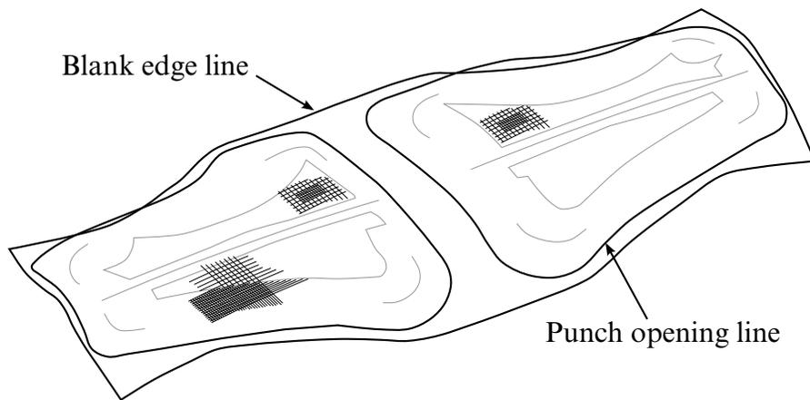
**Figure 15-19.** The fender outer (draw complete) in wireframe mode.
