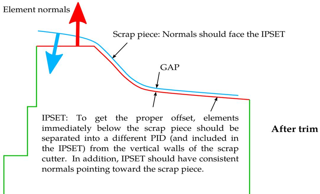
**Figure 12-36.** Element normal of the IPSET in the scrap trimming method. *Model courtesy of the Ford Motor Company.*
