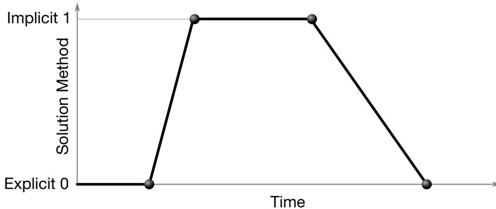
**Figure 12-69.** Solution method, implicit or explicit, controlled by a load curve.
