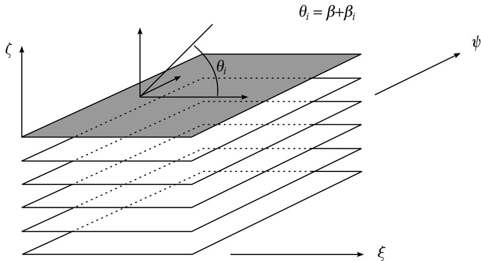
**Figure 18-24.** A multi-layer laminate can be defined. The angle  $\beta_i$  is defined for the  $i$ 'th lamina (integration point), see \*SECTION\_SHELL.
