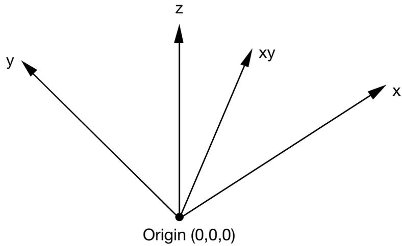
**Figure 15-5.** Definition of the coordinate system with two vectors.
