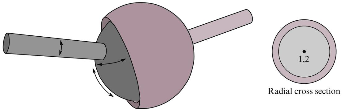
**Figure 10-13.** *Spherical joint.* The relative motion of the rigid bodies is constrained so that nodes which are initially coincident remain coincident. In the above figure the socket's node is not interior to the socket—LS-DYNA does not require that a rigid body's nodes be interior to the body.
