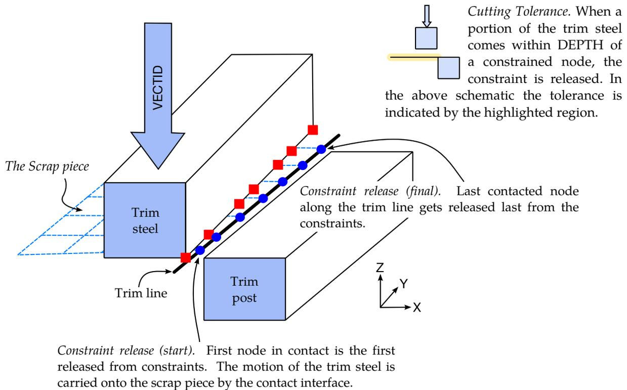
**Figure 12-33.** Contact-based separation and contact-driven kinematics and dynamics in the constraint release method. *Drawing modified from the original sketches courtesy of the Ford Motor Company.*
