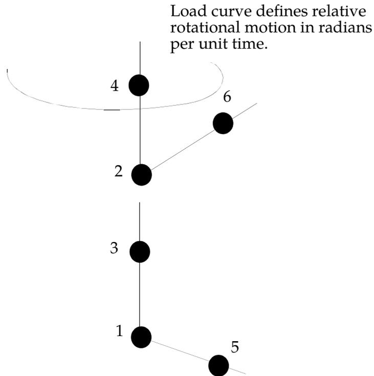
**Figure 10-21.** Rotational motor joint. This joint can be used in combination with other joints such as the revolute or cylindrical joints.
