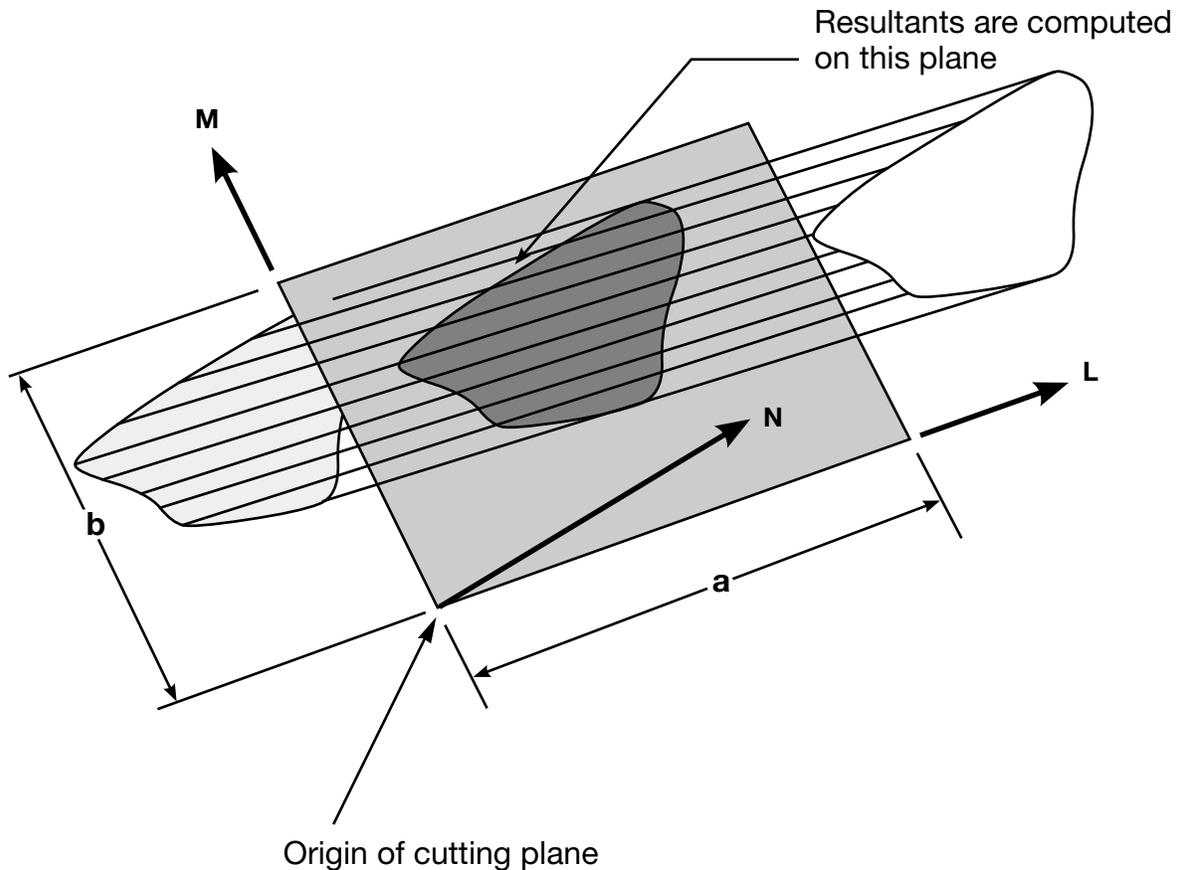
**Figure 14-1.** Definition of cutting plane for automatic definition of interface for cross-sectional forces. The automatic definition does not check for springs and dampers in the section. For best results the cutting plane should cleanly pass through the middle of the elements, distributing them equally on either side. Elements that intersect the edges of the cutting plane are deleted from the cross-section.
