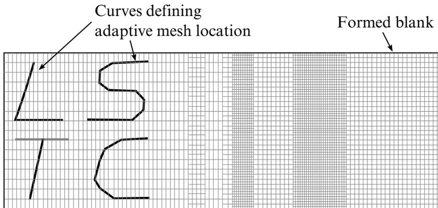
**Figure 15-23.** Curves can be discontinuous and in one IGES file.
