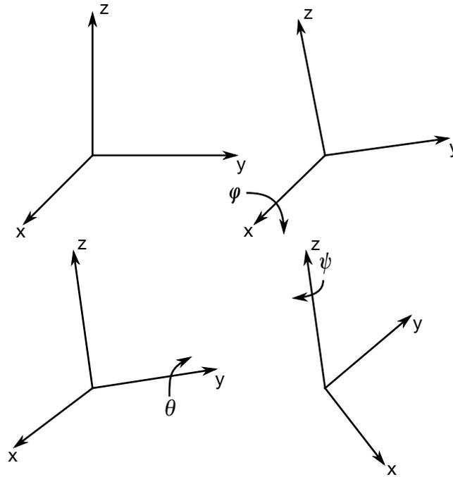
**Figure 10-29.** Definition of angles for the GENERALIZED joint stiffness.
