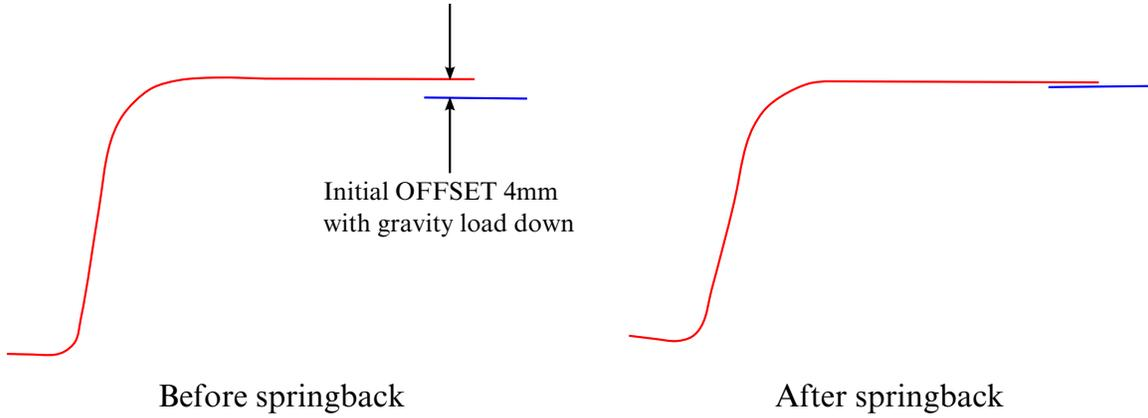
**Figure 12-8.** Springback and contact with nets - gravity down.
