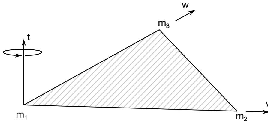
**Figure 27-3.** Follower force and moment acting on a plane defined by nodes  $m_1$ ,  $m_2$ , and  $m_3$ . In this case, the load is applied to node  $m_1$ ; i.e.,  $m = m_1$ . A positive force acts in the positive  $t$ -direction, and a positive moment puts a counterclockwise torque about the normal vector. The positive  $t$ -direction is found by the cross product  $\mathbf{t} = \mathbf{v} \times \mathbf{w}$  where  $\mathbf{v}$  and  $\mathbf{w}$  are vectors as shown.
