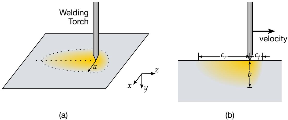
**Figure 5-6.** Schematic illustration of welding with moving torch. The left figure (a) shows the surface of the material from above, while the right figure (b) shows a slice along the dotted line in the  $y$ - $z$  plane.
