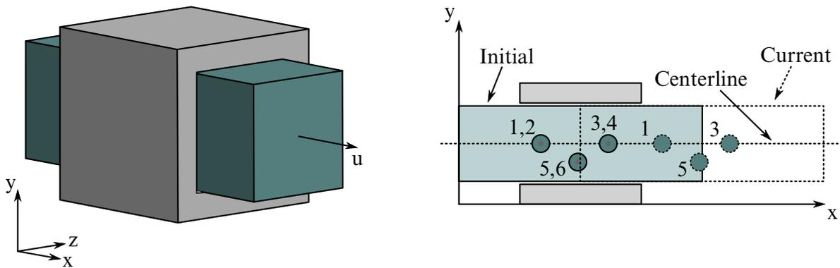
**Figure 10-16. Translational joint.** This is a cylindrical joint with a third pair of off-centerline nodes which restrict rotation. Aside from translation along the centerline, the two rigid bodies are stuck together.
