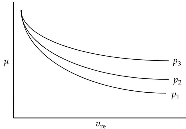
**Figure 11-1.** See variables FS and FD. Friction coefficient,  $\mu$ , can be a function of relative velocity and pressure. Specify a flag for the static coefficient of friction, FS, and a table ID for the dynamic coefficient. This option only works with ONE\_WAY\_SURFACE\_TO\_SURFACE with thickness offsets.
