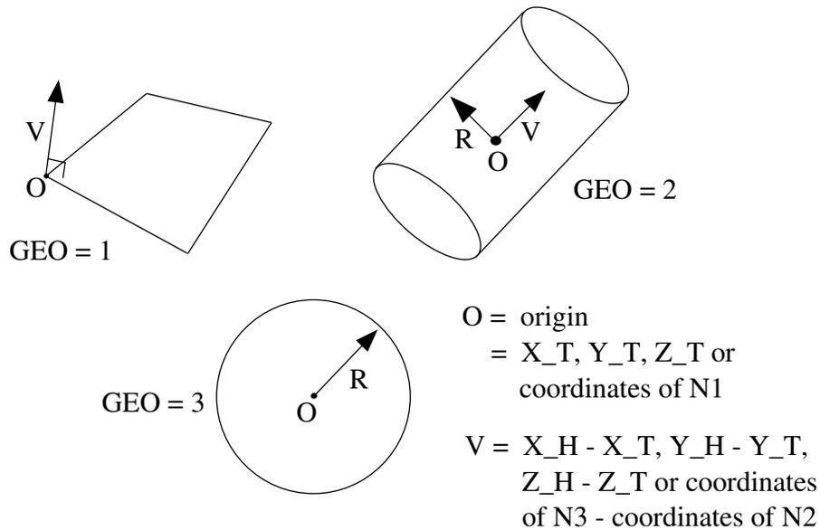
**Figure 15-30.** Geometry types.
