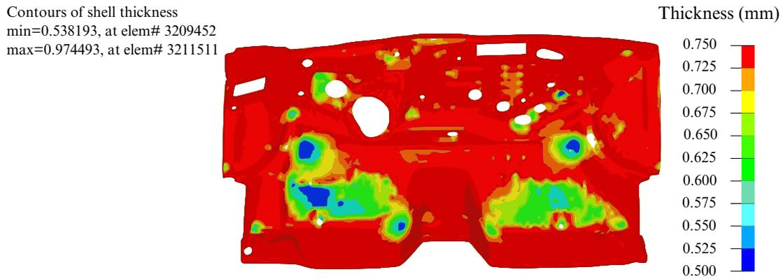
Figure 12-20. Blank thickness with trimmed holes ( $t_0 = 0.75\text{mm}$ ).
