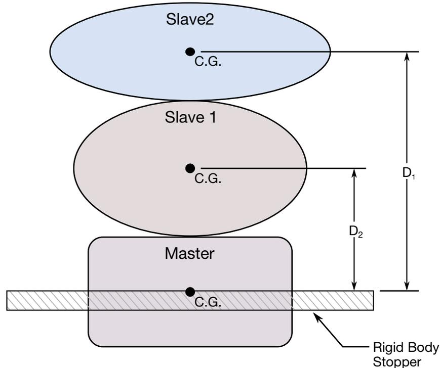
**Figure 10-36.** When the master rigid body reaches the rigid body stopper, the velocity component into the stopper is set to zero. Slave rigid bodies 1 and 2 also stop if the distance between their mass centers and the master rigid body is less than or equal to the input values  $D_1$  and  $D_2$ , respectively.
