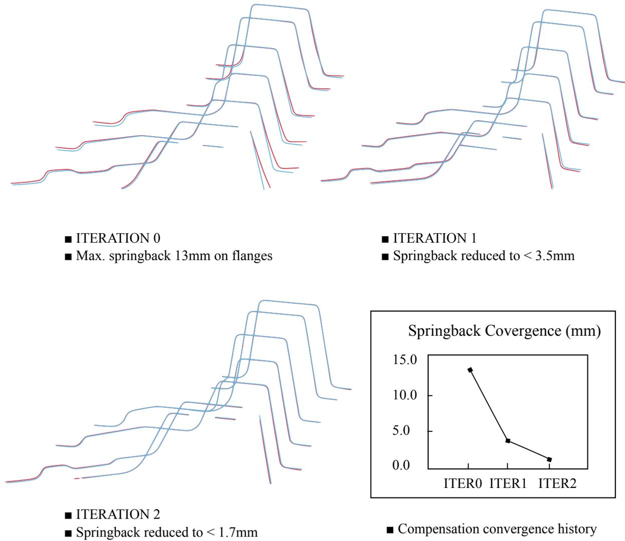
**Figure 25-27.** Iterative springback compensation on NUMISHEET'05 Xnbr(red – springback, blue – design intent)
