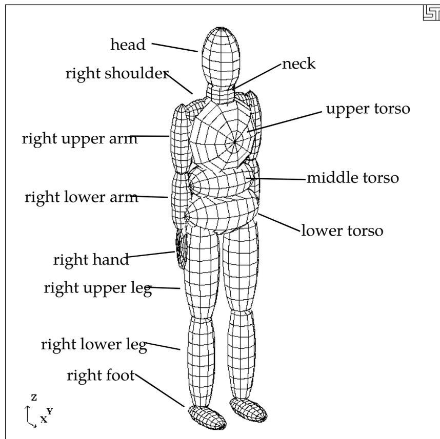
**Figure 56-1.** 50th percentile male dummy in the nominal position.
