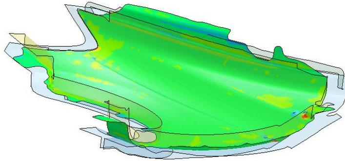
**Figure 12-60.** Mean stress at pad closing.
