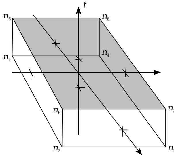
**Figure 18-31.** 8-node Thick Shell Element.
