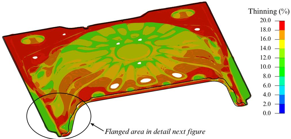
Figure 12-64. Flanging simulation of a rear floor pan using IOPTION 1 (Courtesy of Chrysler, LLC).
