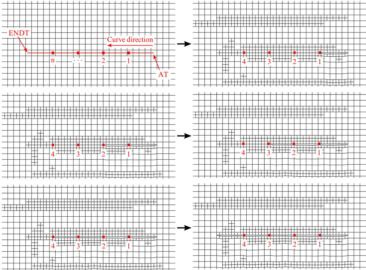
**Figure 18-10.** Progressive lancing - defining AT, ENDT, NTIMES, curve direction; mesh separation progression during progressive lancing.
