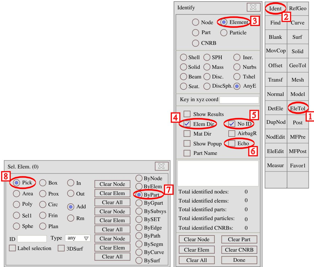
**Figure 15-40.** Checking element directions (N1-N2) by part using LS-PrePost4.0.
