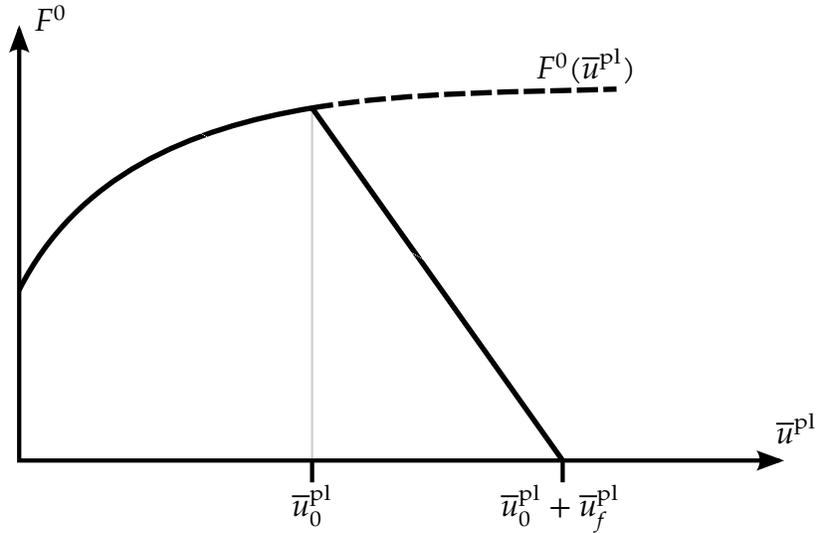
**Figure 10-12.** Force-displacement curve: plasticity and linear damage
