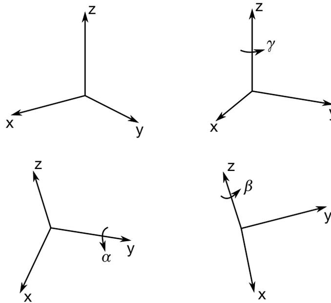
**Figure 10-27.** The angles  $\alpha$ ,  $\beta$ ,  $\gamma$  align rigid body one with rigid body two for the FLEXION-TORSION option.
