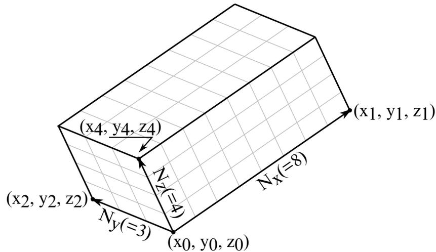
**Figure 3-5.** Illustration of automatic mesh generation for the ALE mesh in a hexahedral region
