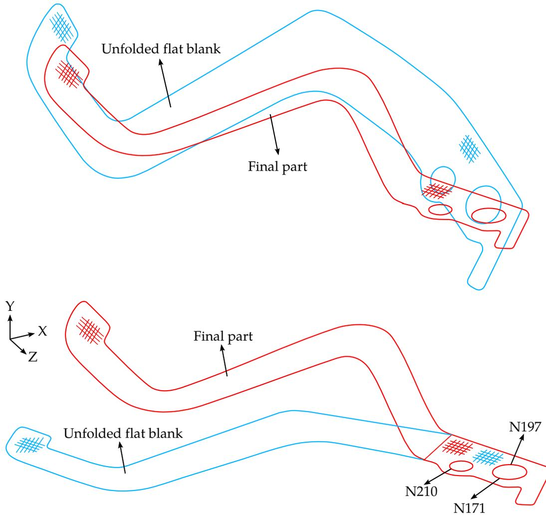
**Figure 12-21.** An example of the results when using the NODE1, NODE2, and NODE3 feature (bottom) and without using the feature (top), courtesy of Kaizenet Technologies Pvt Ltd, India.
