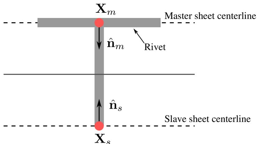
**Figure 10-39.** Single-sheet rivet system.
