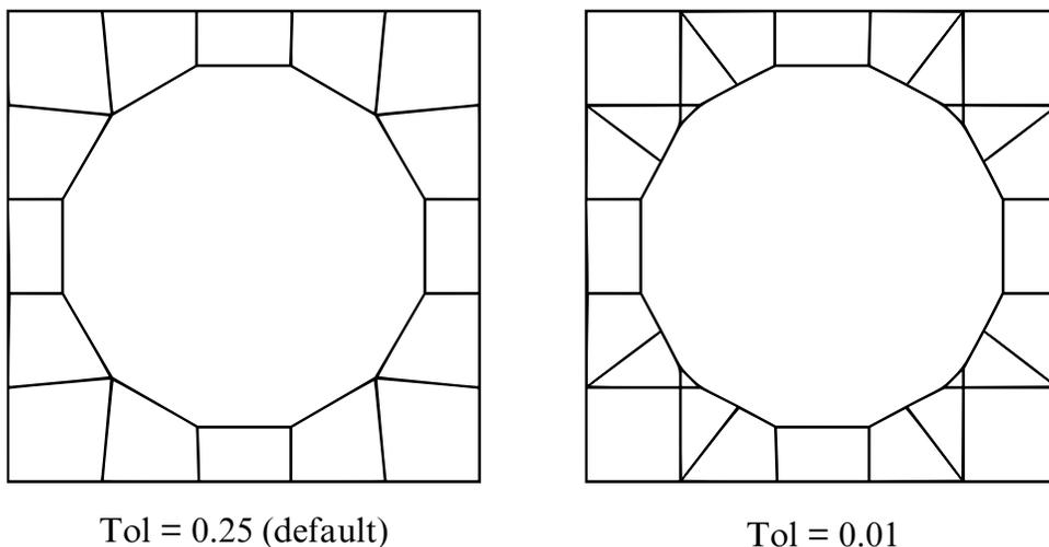
**Figure 15-17.** Trimming Tolerance. The tolerance limits the size of the small elements generated during trimming. The default tolerance (left) produces large elements. Using a tolerance of 0.01 (right) allows smaller elements, and more detail in the trim line.
