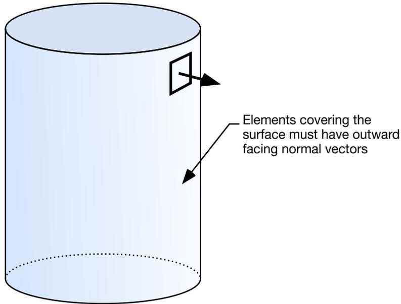
**Figure 27-5.** The shell elements interacting with the fluid must be numbered such that their outward normal vector points into the fluid media.
