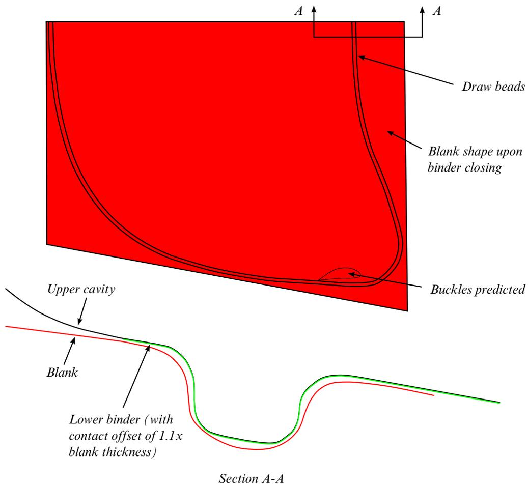
Figure 12-59. Binder closing with beads on a hood outer.
