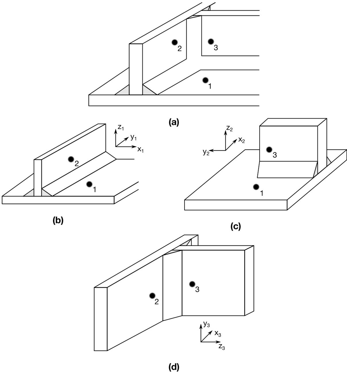
**Figure 10-8.** A simple cross fillet weld illustrates the required input. Here  $NPR = 3$  with nodal pairs  $(A = 2, B = 1)$ ,  $(A = 3, B = 1)$ , and  $(A = 3, B = 2)$ . The local coordinate axes are shown. These axes are fixed in the rigid body and are referenced to the local rigid body coordinate system which tracks the rigid body rotation.
