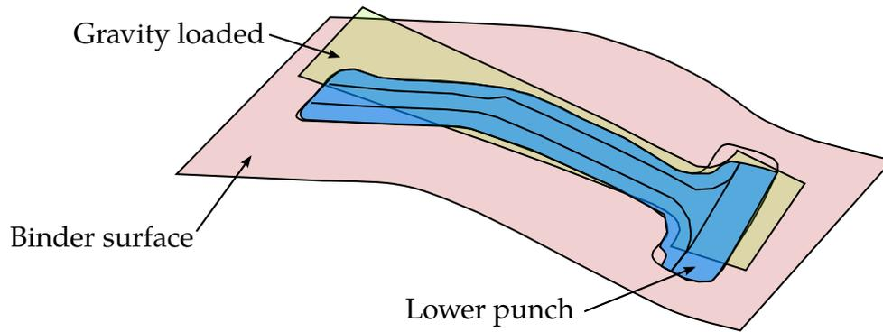
**Figure 25-8.** NUMISHEET 2008 B-pillar; Gravity loaded blank.
