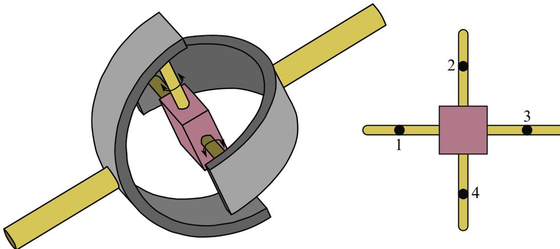
**Figure 10-18.** *Universal Joint.* In contrast with the preceding joints, nodal pairs (1, 2) and (3, 4) are not initially coincident. Rather, the segments formed by (1, 3) and (2, 4) must be orthogonal; and they serve as axes about which the two bodies may undergo relative rotation. The universal joint excludes all other relative motion and the axes remain orthogonal at all time.
