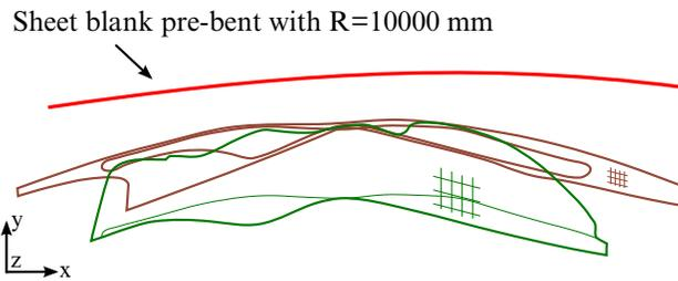
Figure 12-30. Pre-bending using this keyword (1<sup>st</sup> state of D3plots).
