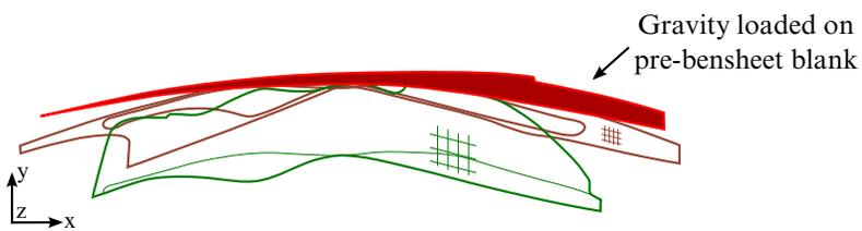
Figure 12-31. Gravity loaded shape (last state of D3plots) with convex shape.
