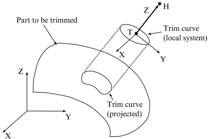
**Figure 15-16.** Trimming Orientation Vector. The tail (T) and head (H) points define a local coordinate system (x,y,z). The global coordinate system is named (X,Y,Z). The local x-direction is constructed in the Xz plane. If X and z nearly coincide ( $|X \cdot z| > 0.95$ ), then the local x-direction is instead constructed in the Yz plane. Trim curve data is input in the x-y plane, and projected in the z-direction onto the deformed mesh to obtain the trim line.
