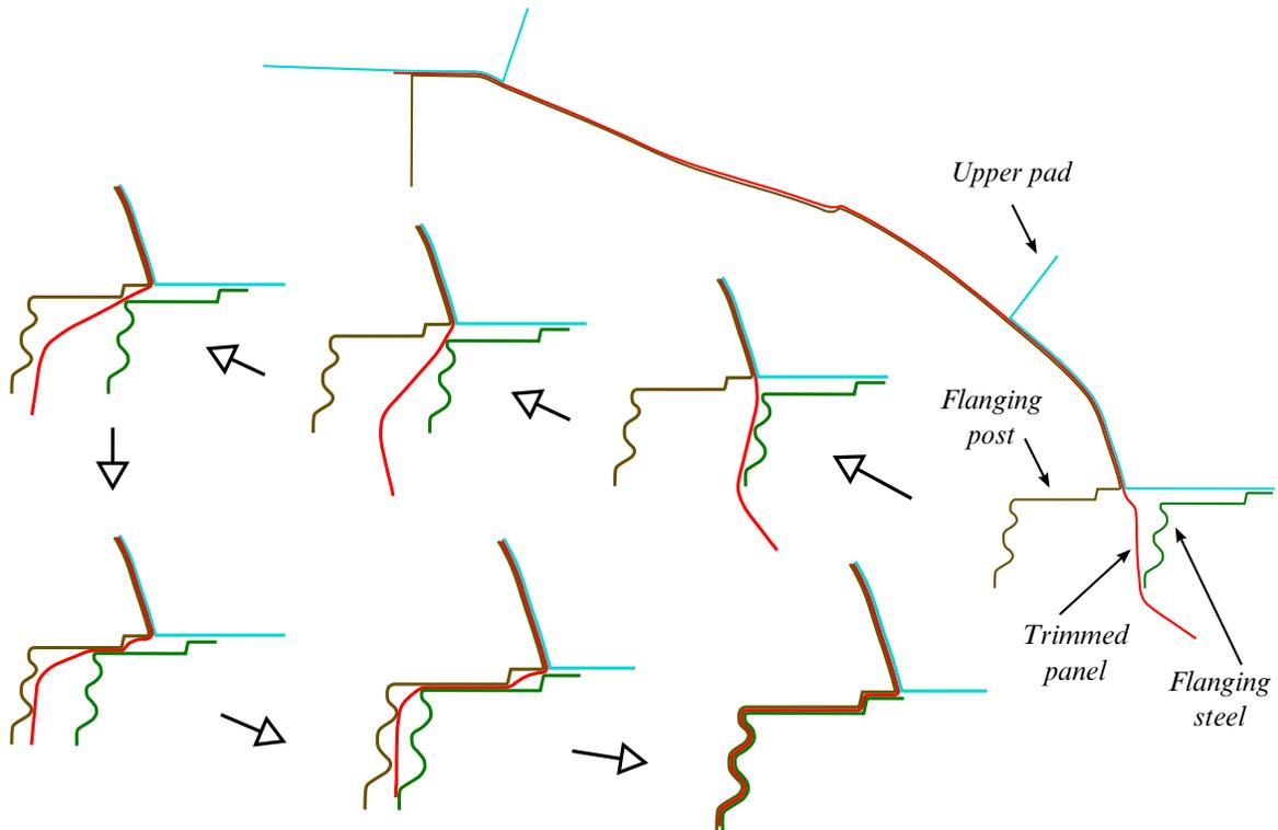
Figure 12-63. Flanging progression along section B (flanging post stationary).
