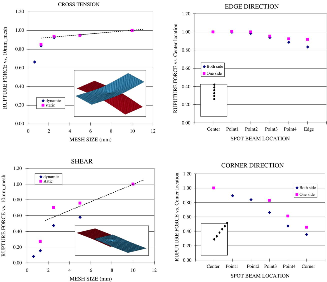
**Figure 12-73** The failure force resultants can depend both on mesh size and the location of weld relative to the center of the contact segment
