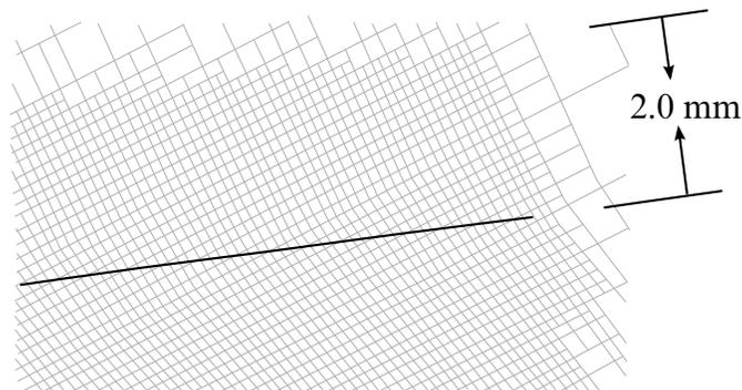
Figure 15-29. Mesh refinement with TCTOL = 2.0.
