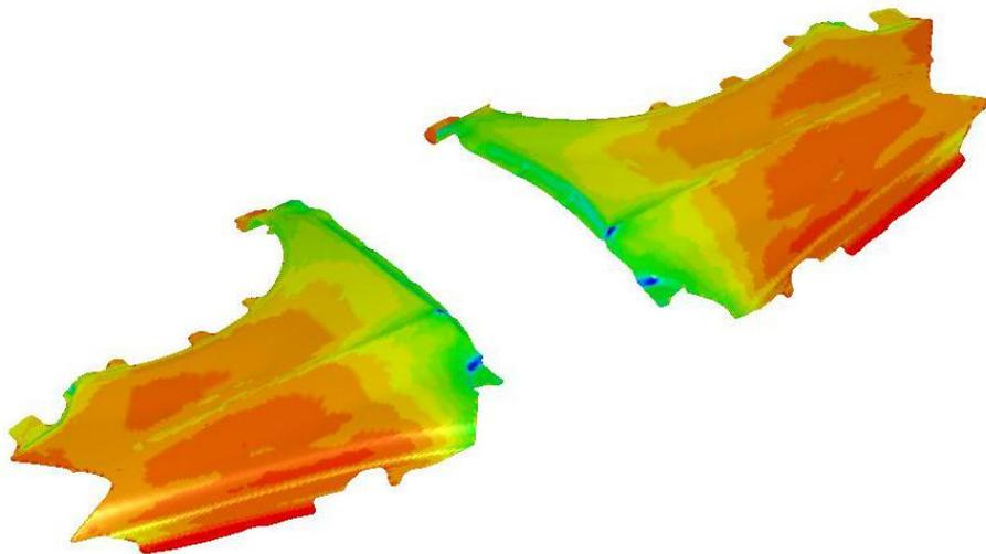
**Figure 15-21.** The fender outer trim complete using the NSEED1/NSEED2 feature.
