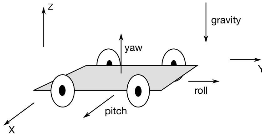
**Figure 23-3.** The vehicle pictured is to be oriented with a successive rotation sequence about the yaw, pitch, and roll axes, respectively. Accordingly, AAXIS = 3, BAXIS = 1, and CAXIS = 2. The direction of gravity is given by GRAV = -3.
