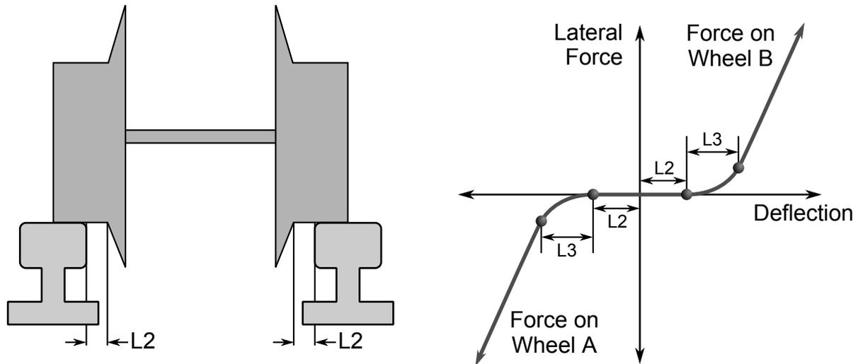
**Figure 33-2.** Illustration of lateral drift parameters L2 and L3 from \*RAIL\_TRACK.
