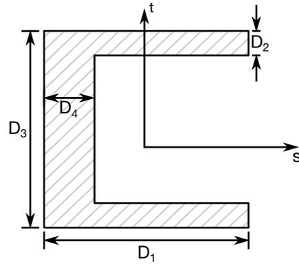
Figure 35-2. SECTION\_02 ⇒ Channel
