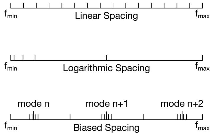
**Figure 20-2.** Spacing options of the frequency points.
