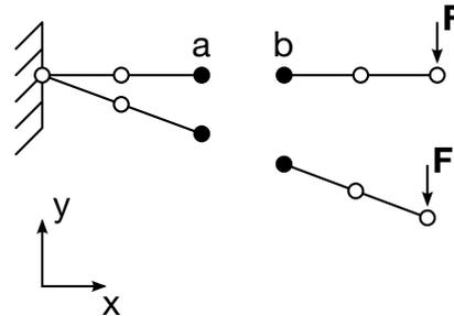
**Figure 10-35.** Two different ways to constrain node *a* and *b*. For rigid-body type situations this card, \*CONSTRAINED\_NODE\_SET may lead to un-physical results.
