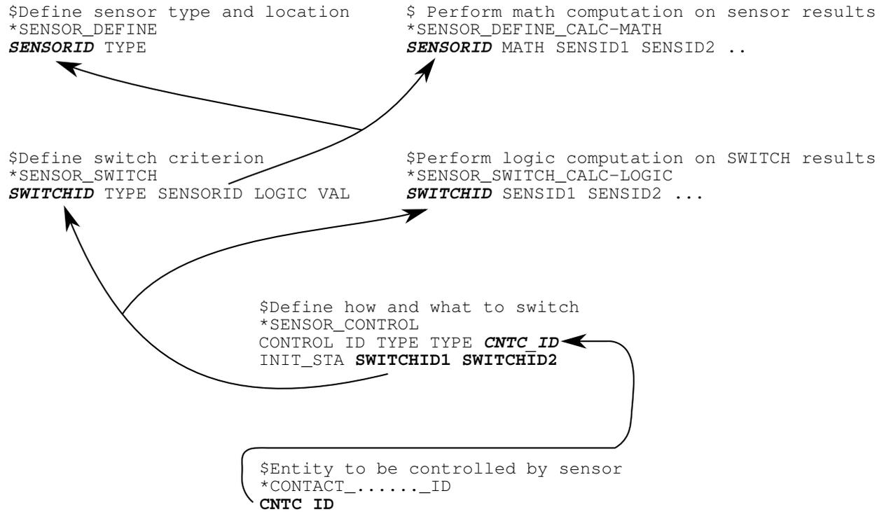
**Figure 36-1.** Relationship between sensor keyword definitions.
