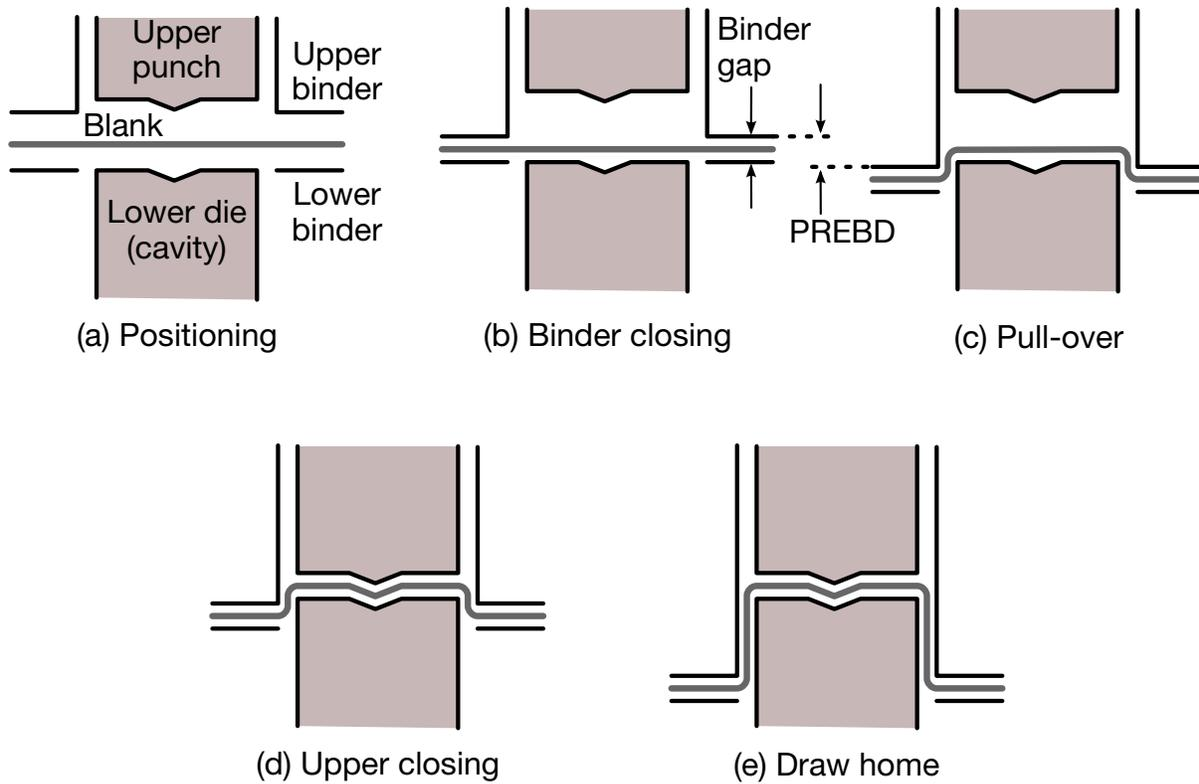
Figure 12-44. IDTEMP = 3: forming in 4-piece stretch draw.
