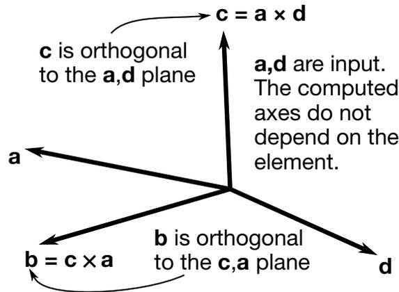
**Figure 18-29.** Two vectors  $\mathbf{a}$  and  $\mathbf{d}$  are defined and the triad is computed and stored.
