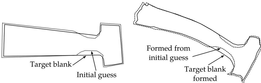
Figure 25-15. Iteration 0 results comparison with target.
