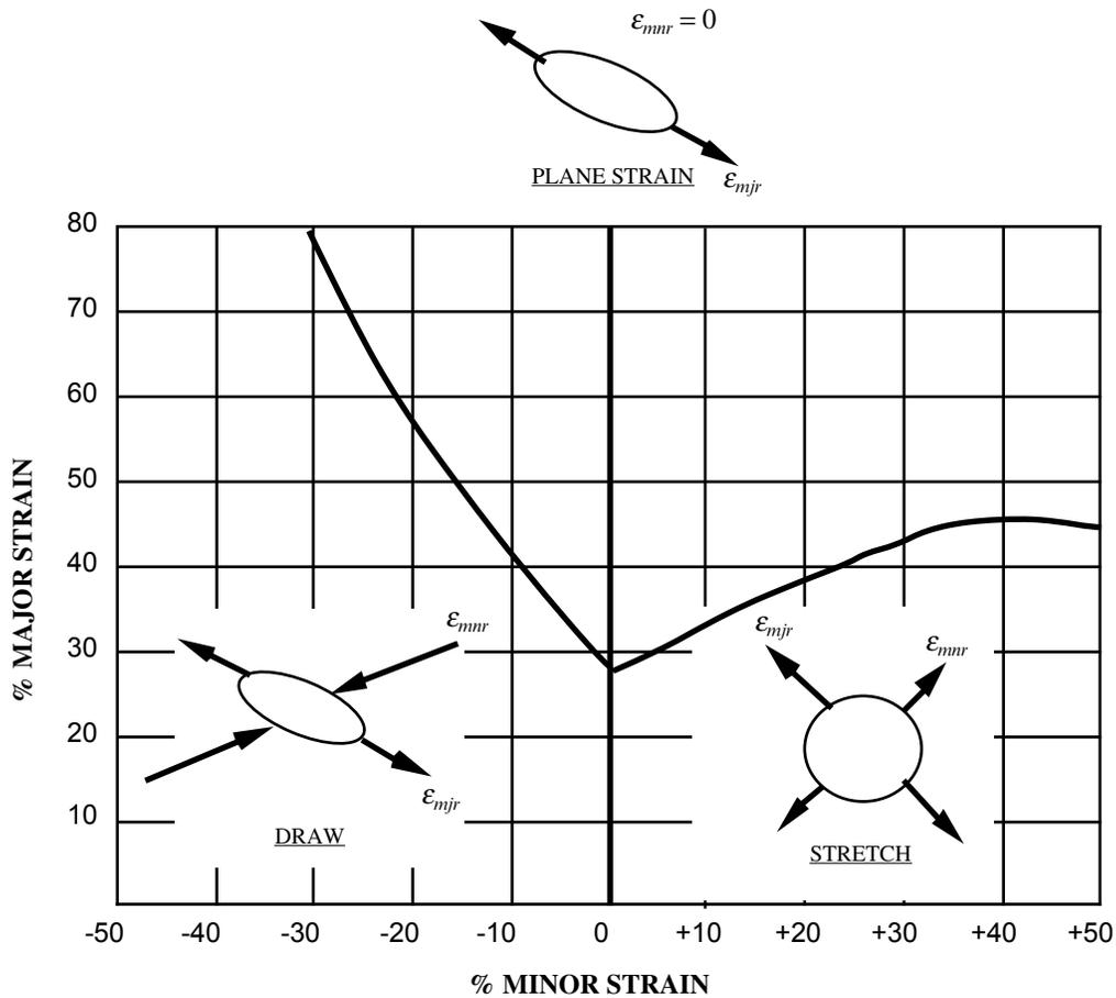
**Figure 15-12.** Flow limit diagram.
