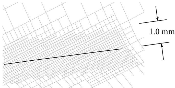
Figure 15-28. Mesh refinement with TCTOL = 1.0.
