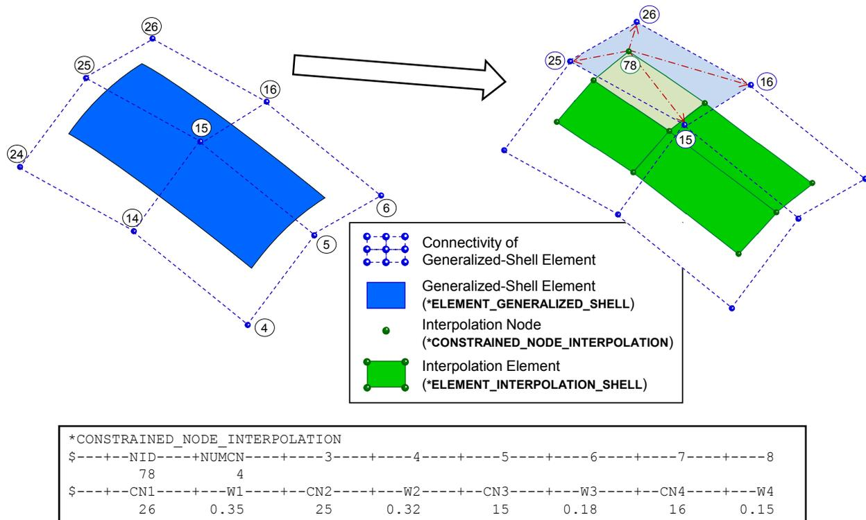
Figure 10-34. Example of a \*CONSTRAINED\_NODE\_INTERPOLATION card
