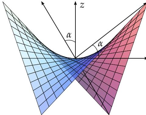
**Figure 12-71.** Illustration of an element in a *W-Mode*. One pair of opposite corners go up, and the other pair goes down. The angle,  $\alpha$ , is formed by the plane of the flat element and by the vector connecting the center to the corner. See [Remark 4](#).
