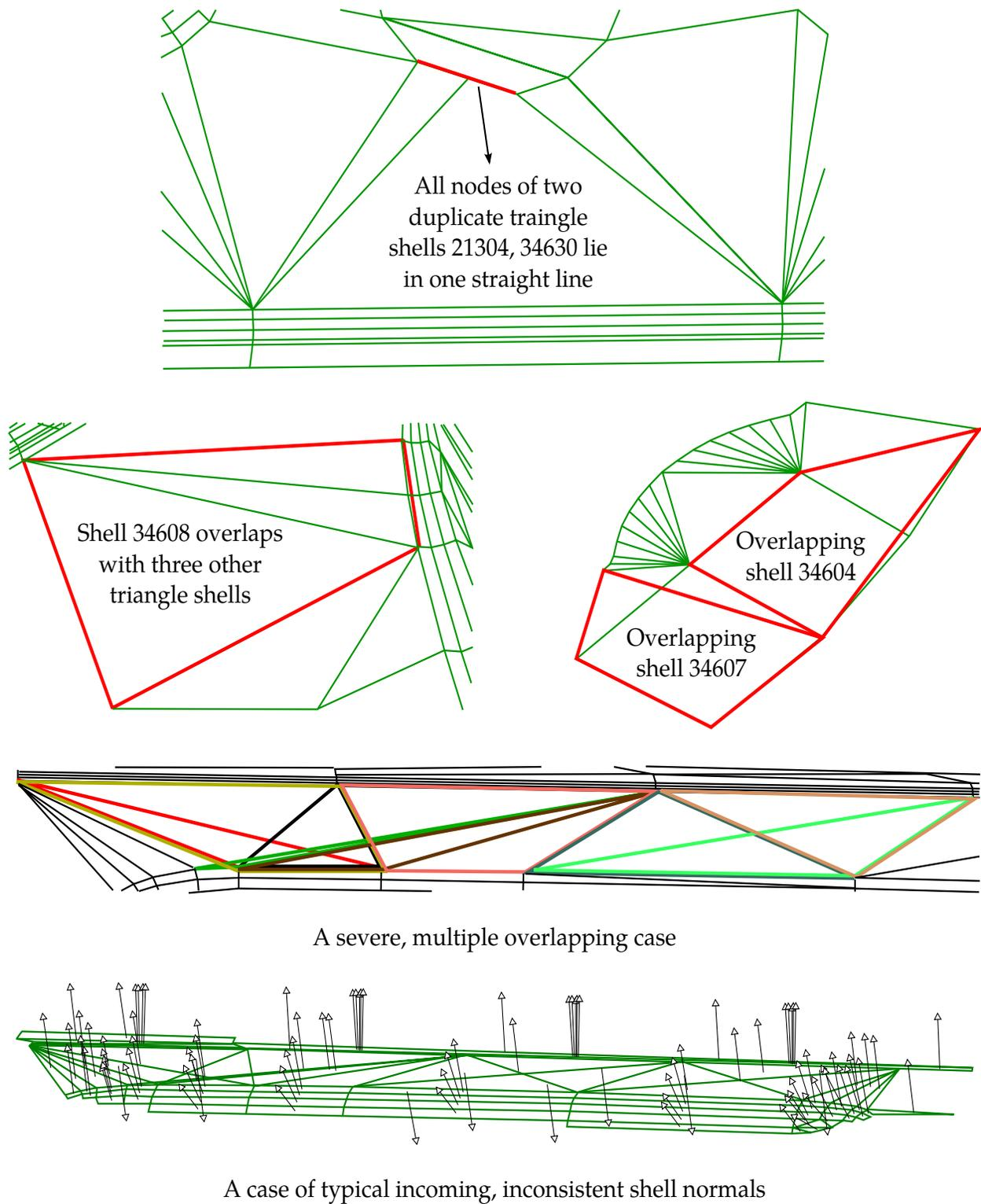
**Figure 12-6.** A few cases of the tooling mesh problems handled by this keyword.
