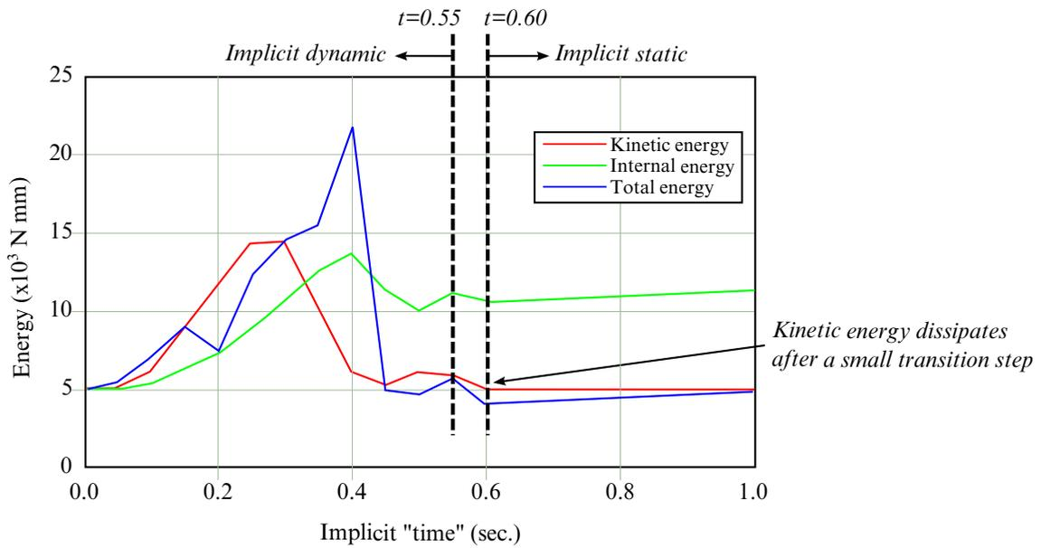
Figure 12-68. Switching between implicit dynamic and implicit static.
