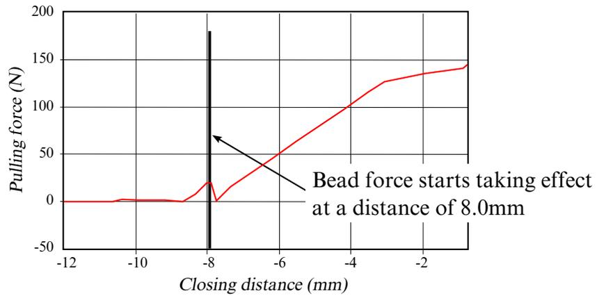
**Figure 11-8.** Pulling force (NODFOR) vs. closure distance.
