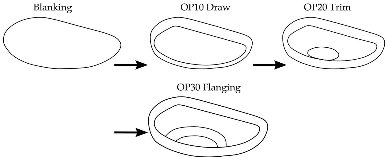
**Figure 25-2.** A stamping process consists of draw, trim and flanging (*Courtesy of Metal Forming Analysis Corporation*). The labels *OP10*, *OP20*, and *OP30* are used extensively in the ensuing discussion.
