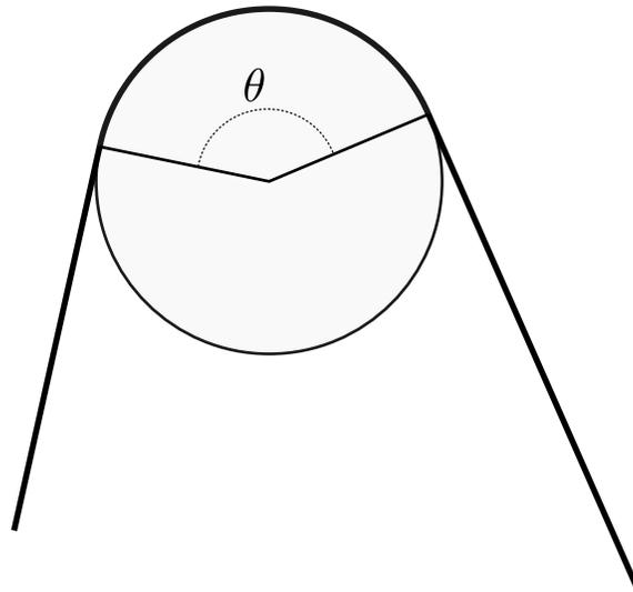
Figure 18-21. Front view showing wrap angle.
