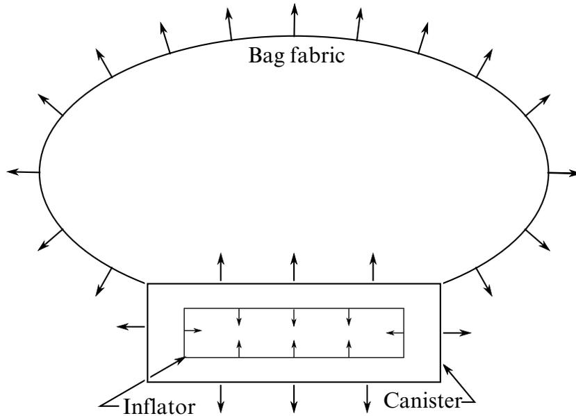
**Figure 3-6.** Arrows indicate “outward” normal
