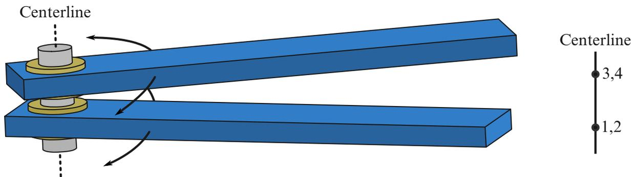
**Figure 10-14.** *Revolute Joint.* Both nodal pairs (1, 2) and (3, 4) are constrained to remain coincident. Consequently, the relative motion of these rigid bodies is restricted to rotations about the line segment formed by the two pairs of coincident nodes. This segment is labeled the "centerline".
