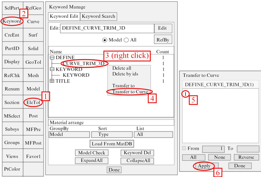
Figure 25-10. Converting trimcurves.ibo to IGES format in LSPP4.0.
