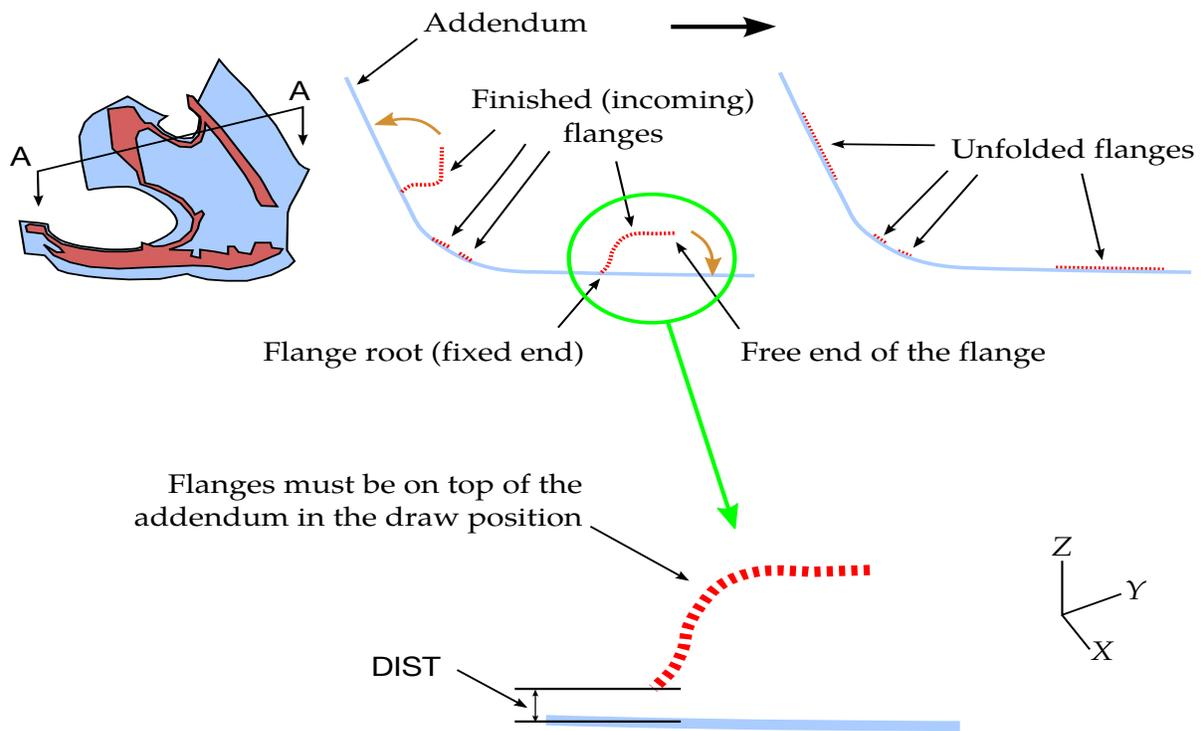
**Figure 12-48.** A section view showing flange unfolding before and after.
