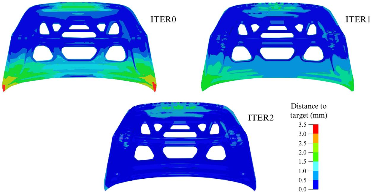
Figure 25-31. Iterative compensation for a localized (backlite) region.
