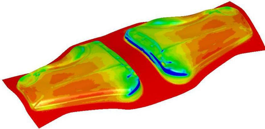
**Figure 15-20.** The fender outer - thickness/thinning plot on the drawn panel.
