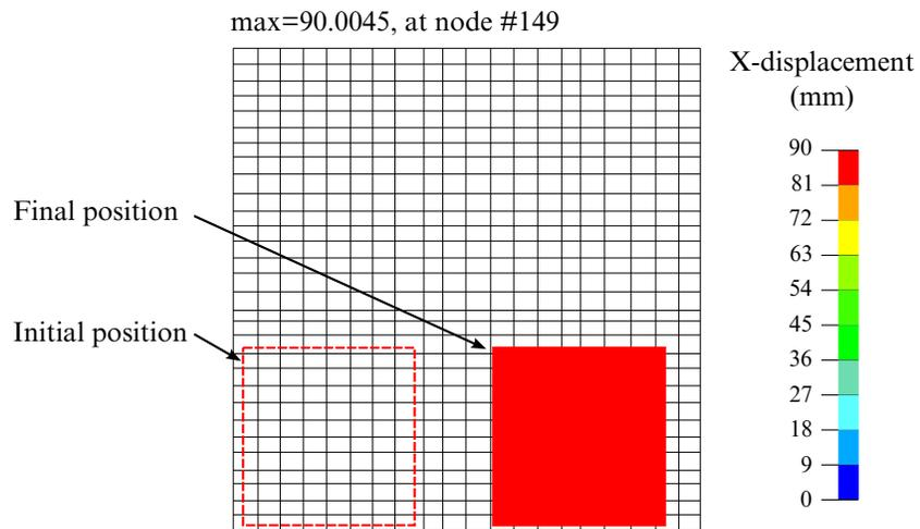
**Figure 15-36.** Initial and final position of the blank.
