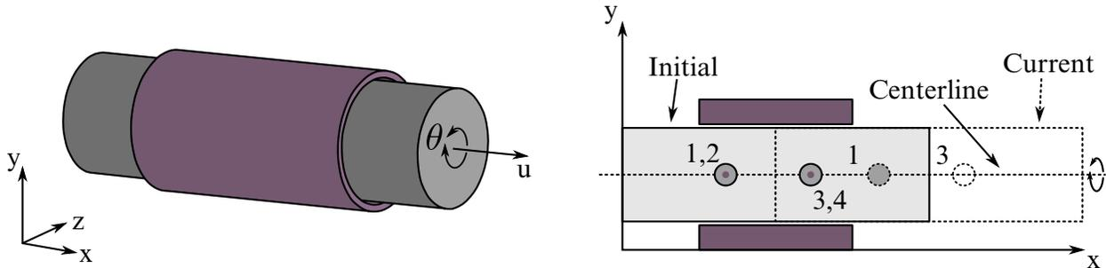
**Figure 10-15. Cylindrical Joint.** This joint is derived from the rotational joint by relaxing the constraints along the centerline. This joint admits relative rotation and translation along the centerline.
