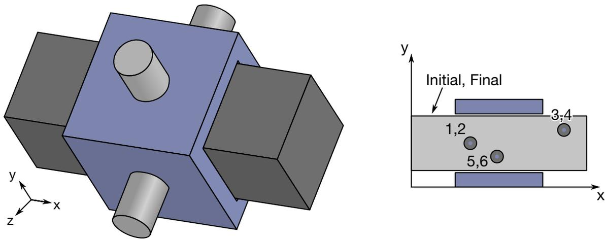
**Figure 10-19. Locking Joint.** A locking joint couples two rigid bodies in all six degrees-of-freedom. The forces and moments required to form this coupling are written to the jntforc file (\*DATABASE\_JNTFORC). As stated in the Remarks, forces and moments in jntforc are calculated halfway between N1 and N3. Nodal pairs (1, 2), (3, 4) and (5, 6) must be coincident. The three spatial points corresponding to three nodal pairs must be neither collocated nor collinear.
