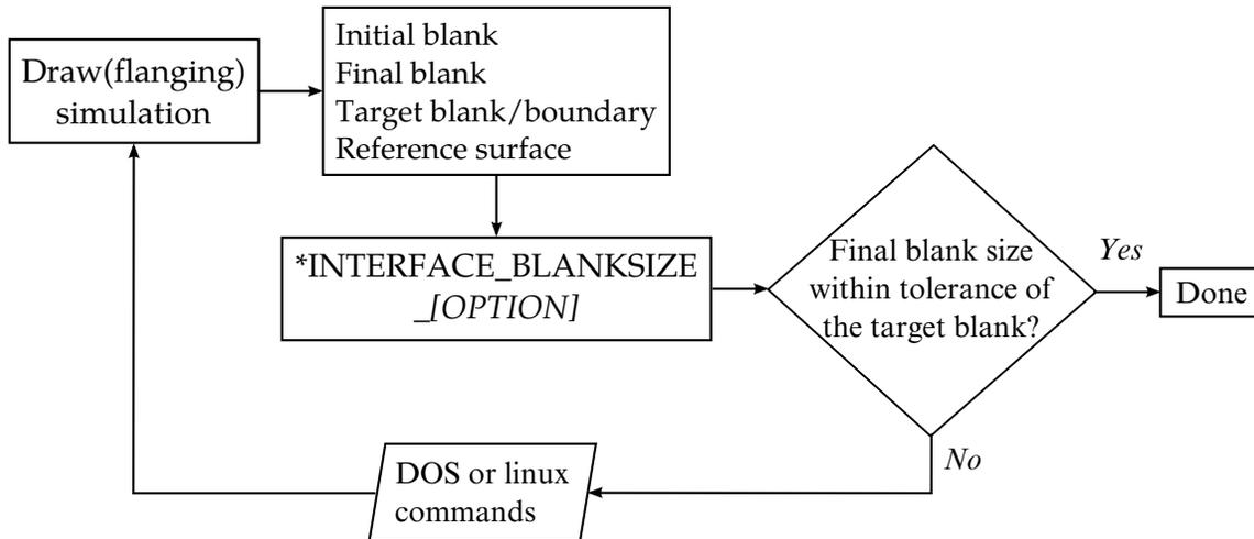
Figure 25-5. An iterative blank size development process.
