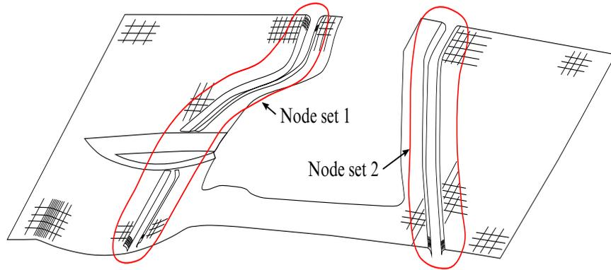
**Figure 25-36.** Local smoothing - two node sets defined including some nodes on the relatively flat binder area for both left and right draw beads.
