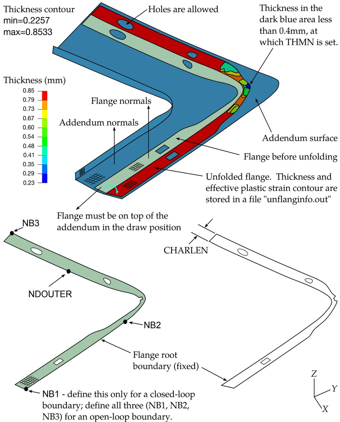
Original flange is modified based on THMN=0.4 and the mesh is stored in a file "mdfiedflangedpart.k". Boundary curves can be created using LSPP4.0 under Curve/Spline/From mesh/by part.
