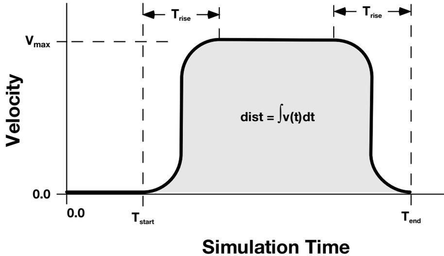
**Figure 15-15.** Smooth curve created automatically using \*DEFINE\_CURVE\_SMOOTH. This shape is commonly used to control velocity of tools in metal forming applications as shown in the above graph, but can be used for other applications in place of any standard load curve.
