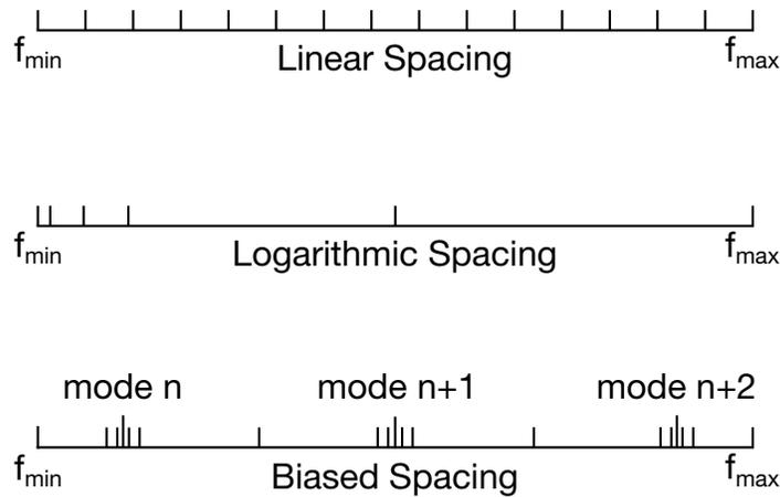
**Figure 14-6.** Spacing options of the frequency points.
