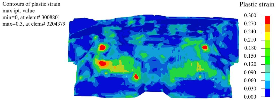
Figure 12-19. Effective plastic strain with EPSMAX = 0.3.
