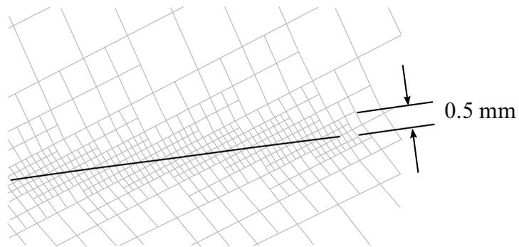
Figure 15-27. Mesh refinement with TCTOL = 0.5.
