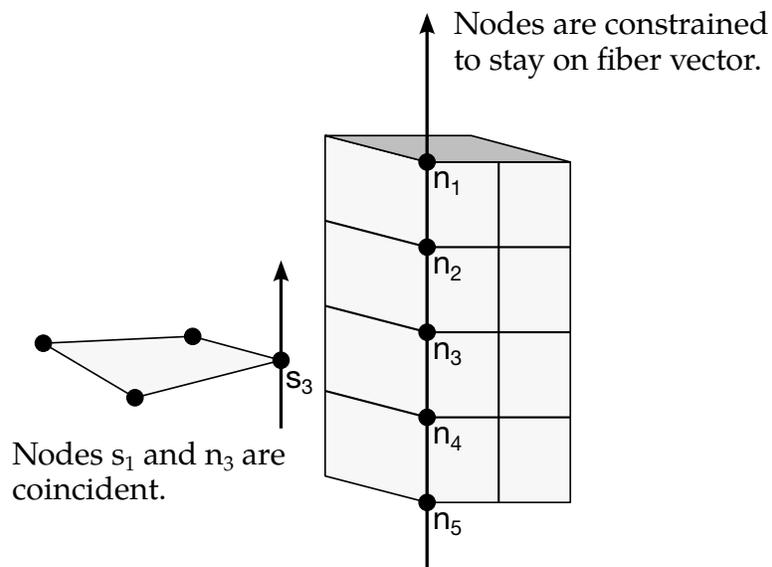
**Figure 10-37.** The interface between shell elements and solids ties shell node  $s_1$  to a line of nodes on the solid elements  $n_1$ - $n_5$ . It is very important for the nodes to be aligned.
