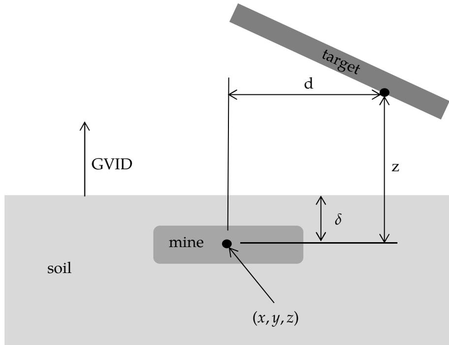
**Figure 23-2.** Schematic of the buried mine parameters.
