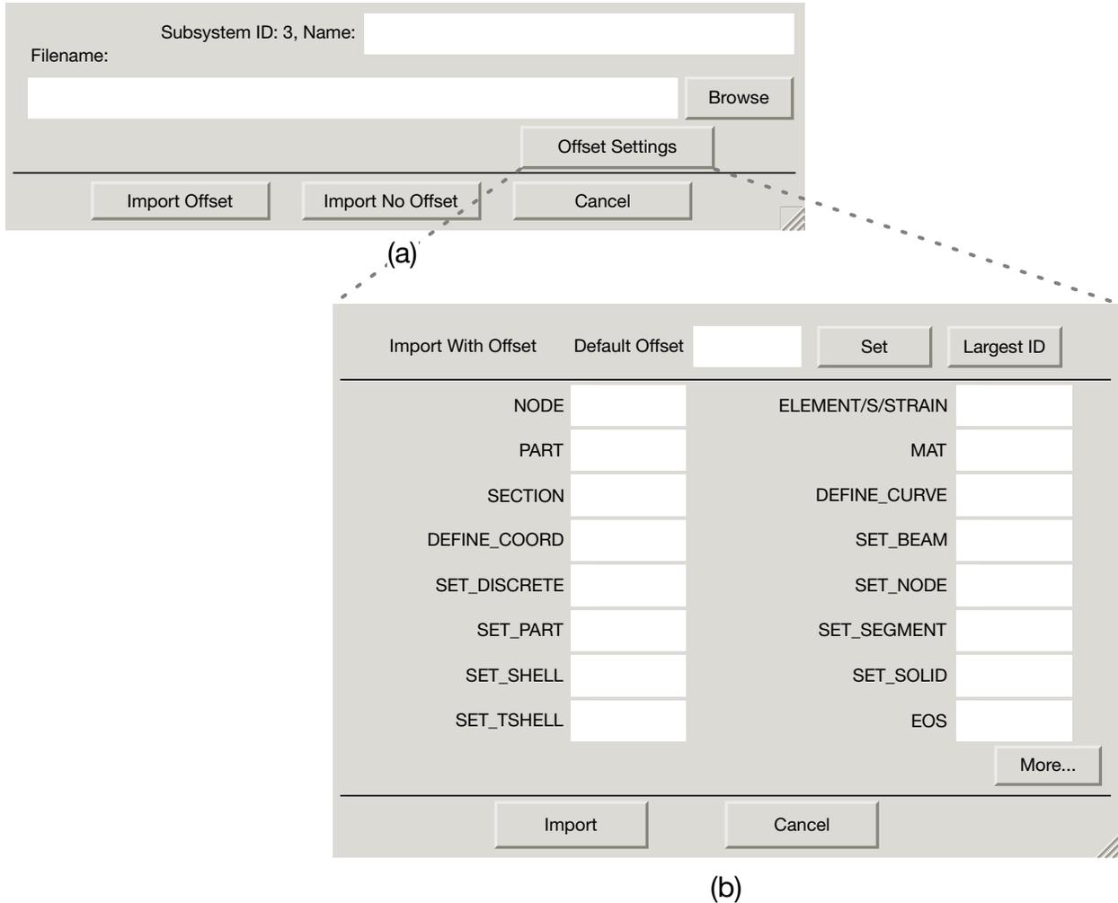
**Figure 29-1.** (a) the file → import → keyword dialog box; (b) the LS-PrePost dialog that takes the offset as a function of ID type.
