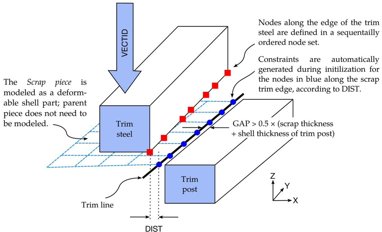
**Figure 12-32.** Modeling details of the constraint release method. *Drawing modified from the original sketches courtesy of the Ford Motor Company.*
