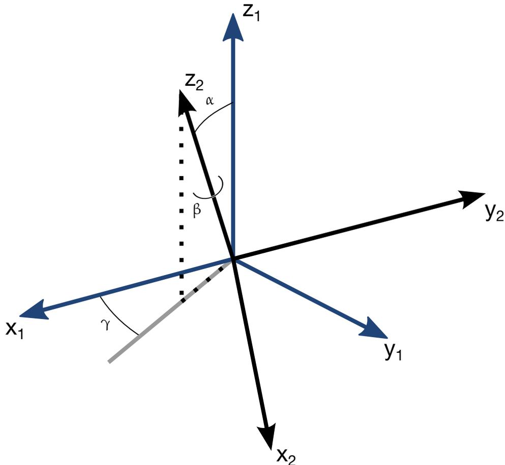
**Figure 10-28.** Flexion-torsion joint angles. If the initial positions of the local coordinate axes of the two rigid bodies connected by the joint do not coincide, the angles,  $\alpha$  and  $\gamma$ , are initialized and torques will develop instantaneously based on the defined load curves. The angle  $\beta$  is also initialized but no torque will develop about the local axis on which  $\beta$  is measured. Rather,  $\beta$  will be measured relative to the computed offset.
