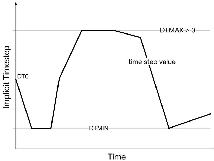
**Figure 12-51.** The implicit time step size changes continuously as a function of convergence within the bounds set by DTMIN and DTMAX
