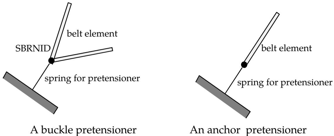
**Figure 18-16.** Buckle and anchor pretensioner.
