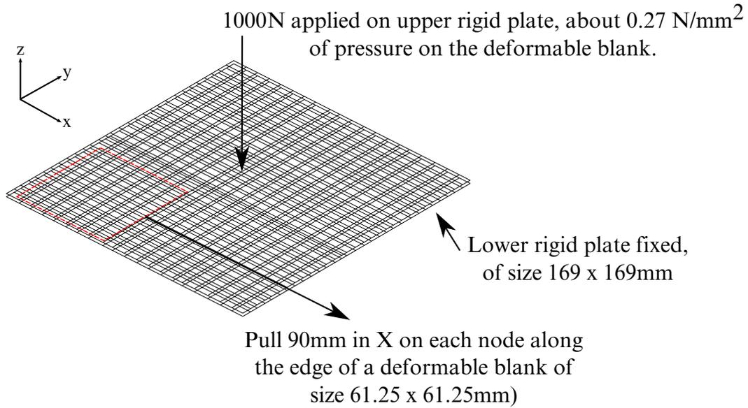
**Figure 15-35.** Boundary and loading conditions of a small test model.
