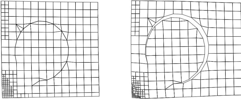
**Figure 18-9.** Instant lancing – open-loop hole. The left mesh is immediately after AT while the right one is at punch home.
