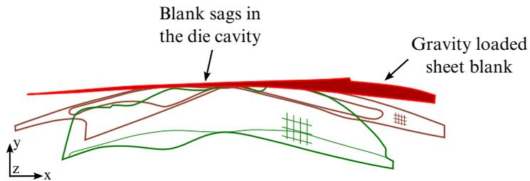
**Figure 12-29.** Gravity loaded blank without using this keyword.
