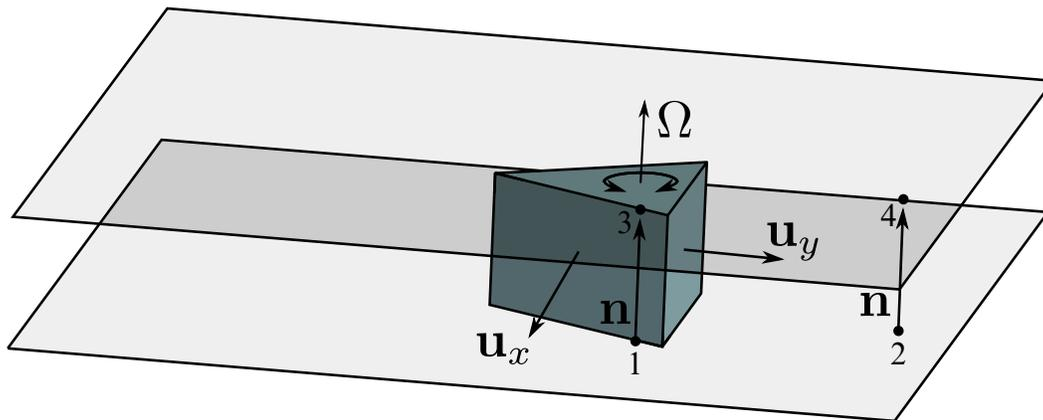
**Figure 10-17.** *Planar joint.* This joint is derived from the rotational joint by relaxing the constraints normal to the centerline. Relative displacements along the direction of the centerline are excluded.
