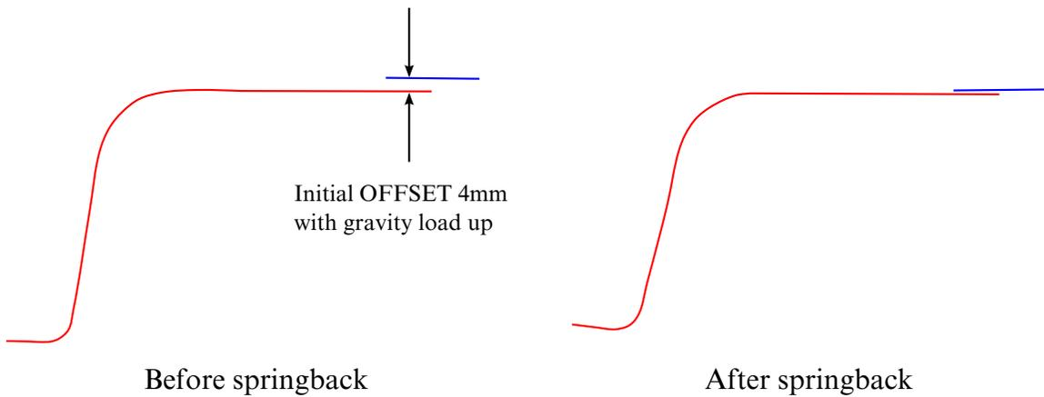
**Figure 12-9.** Springback and contact with nets – gravity up.
