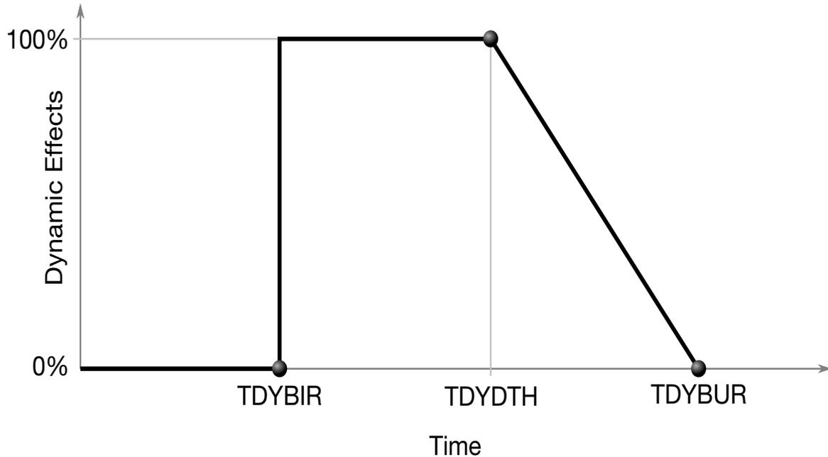
**Figure 12-53.** Birth, death, and burial time for implicit dynamics. The terms involving  $M$  and  $D$  are scaled by a factor between ranging between 1 and 0 to include or exclude dynamical effects, respectively.
