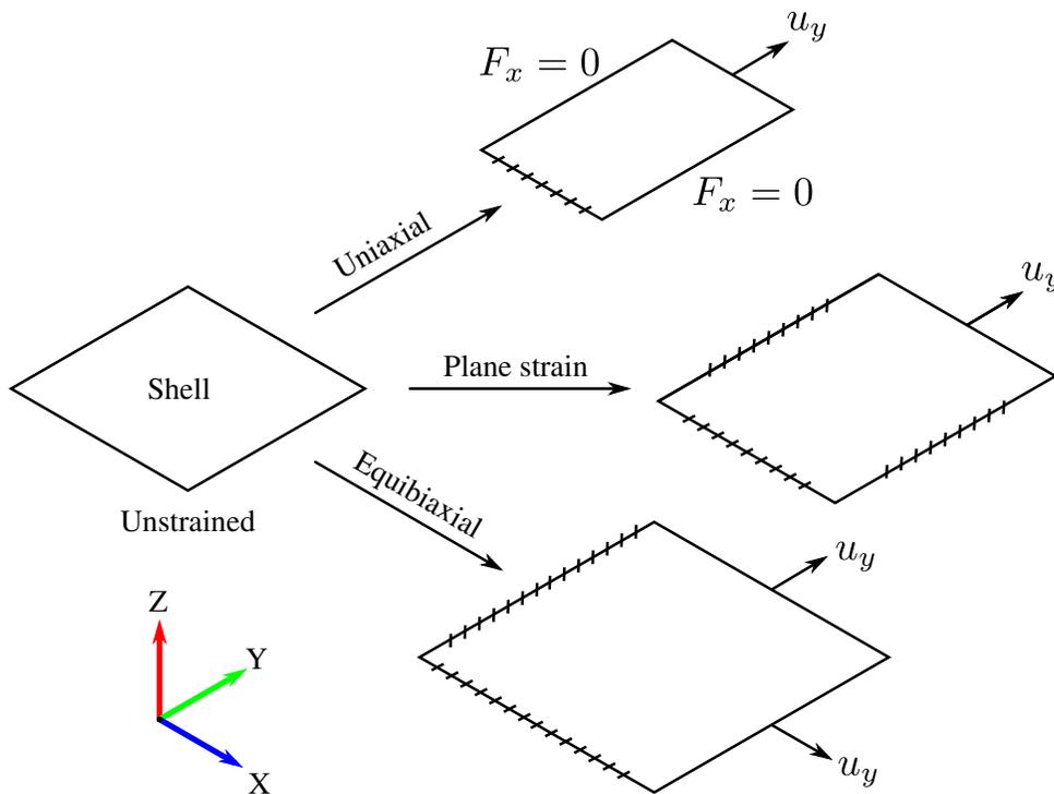
Figure 15-13. A single shell strained in three different strain paths
