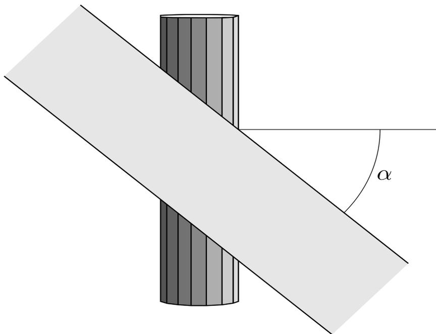
Figure 18-22. Top view shows orientation of belt relative to axis.
