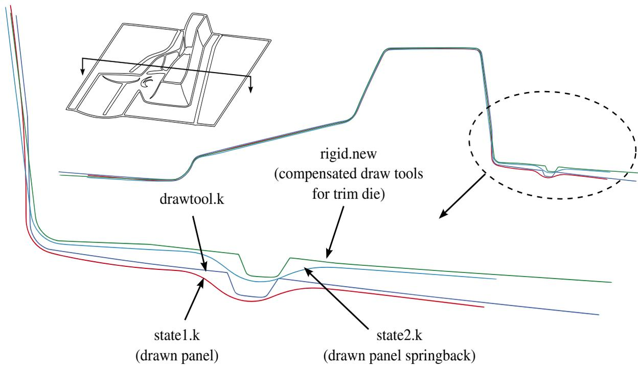
Figure 25-33. Trim die compensation with drawn panel springback shape.
