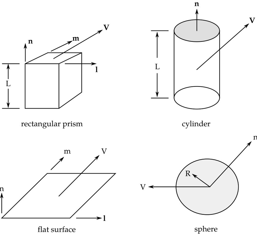
**Figure 34-1.** Vector  $\mathbf{n}$  determines the orientation of the generalized rigidwalls. For the prescribed motion options the wall can be moved in the direction  $\mathbf{V}$  as shown.
