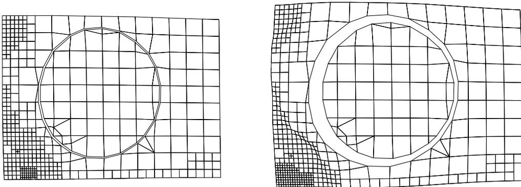
**Figure 18-8.** Instant lancing – closed-loop hole. The left mesh is immediately after AT while the right one is at punch home.
