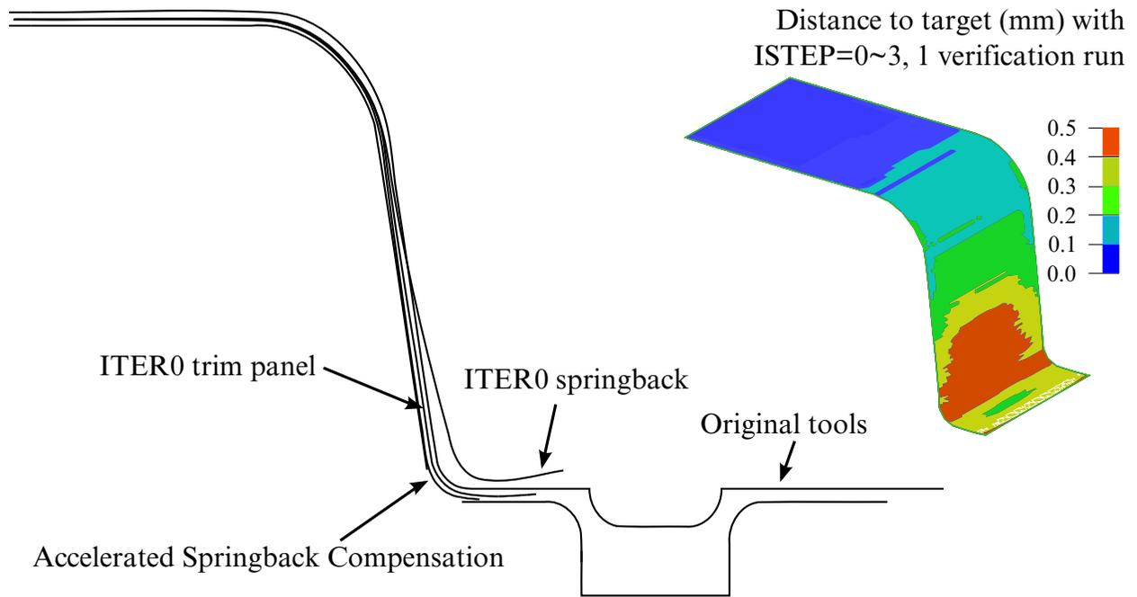
Figure 25-32. Accelerated Springback Compensation.
