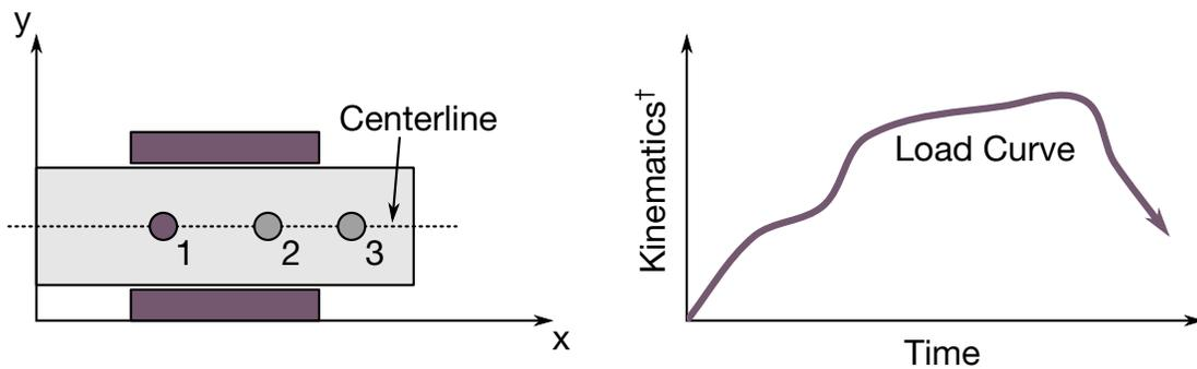
**Figure 10-20. Translational motor joint.** This joint is usually used in combination with the translational or the cylindrical joint. The first node must belong to one rigid body, and nodes 2 and 3 to the other. The value of the load curve may specify any of several kinematic measures see TYPE.
