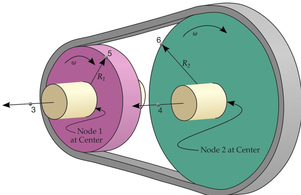
**Figure 10-25.** Pulley joint. Nodal pairs (1, 3) and (2, 4) define axes that are orthogonal to the pulleys. Nodal pairs (1, 5) and (2, 6) define vectors in the plane of the pulleys. The ratio  $R_2/R_1$  is specified.
