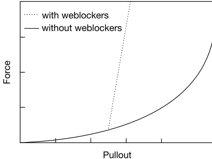
**Figure 18-18.** Retractor force pull characteristics.
