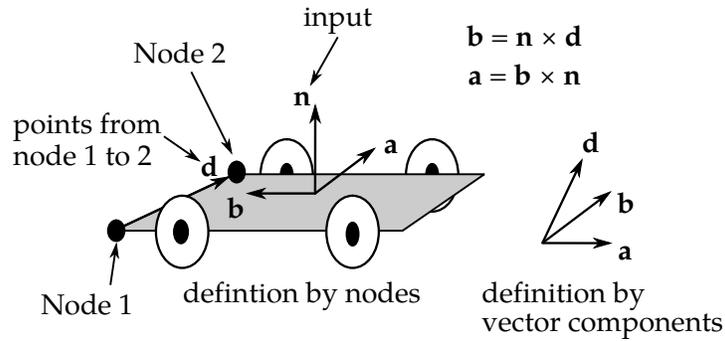
**Figure 34-3.** Definition of orthotropic friction vectors. The two methods of defining the vector,  $\mathbf{d}$ , are shown. If vector  $\mathbf{d}$  is defined by nodes 1 and 2, the local coordinate system may rotate with the body which contains the nodes; otherwise,  $\mathbf{d}$  is fixed in space, thus on the rigid wall, and the local system is stationary.
