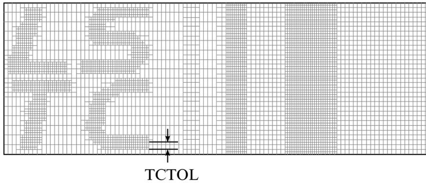
**Figure 15-24.** Define the variable TCTOL to limit the mesh adaptivity area.
