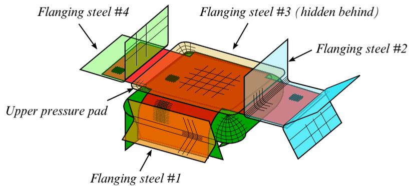
**Figure 12-25.** An example of multiple flanging process.
