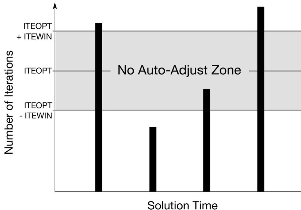
**Figure 12-50.** Iteration Window as defined by ITEOPT and ITEWIN.
