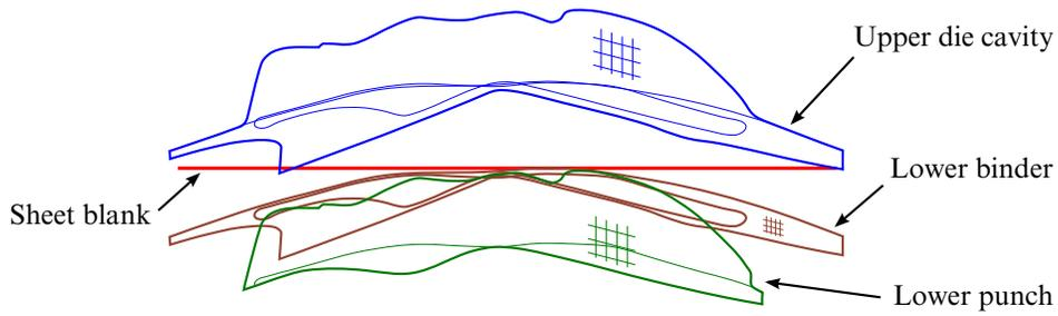
**Figure 11-18.** Initial parts auto-positioned at  $t = 0.0$ .
