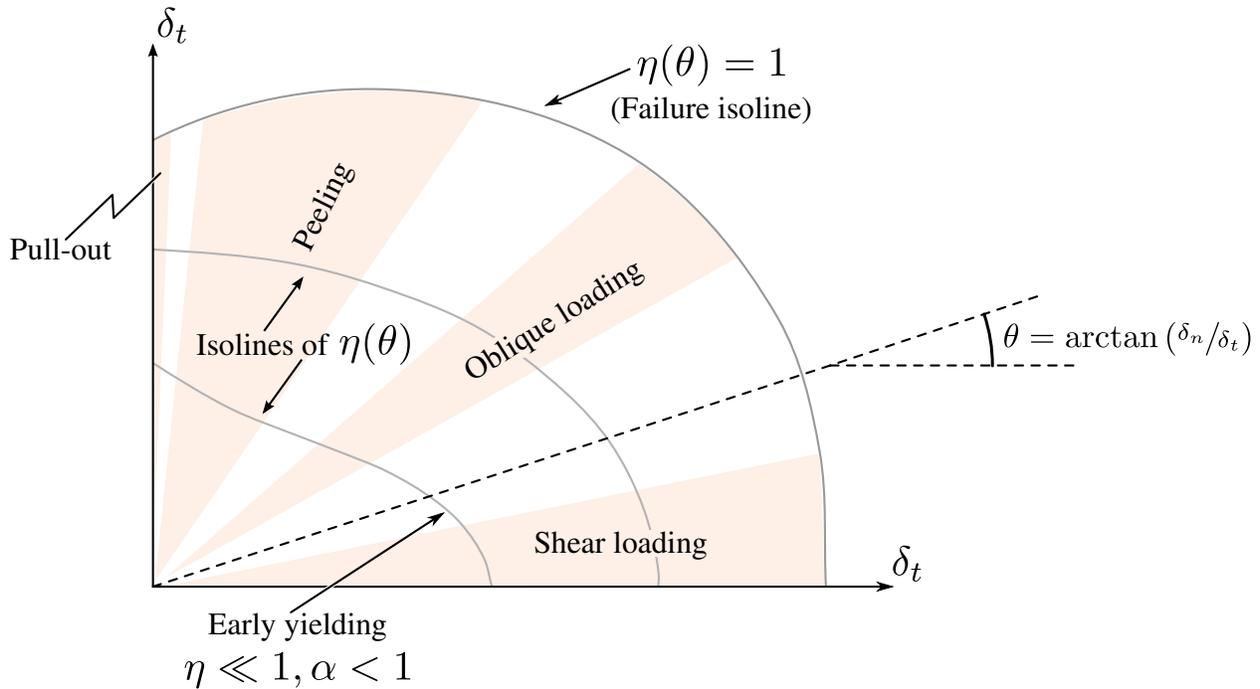
**Figure 10-43.** Isosurfaces of  $\eta(\theta)$
