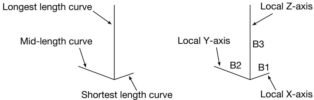
Figure 15-4. Input curves (left). The generated local coordinate system is written to the d3plot file as a part consisting of three beams (right).
