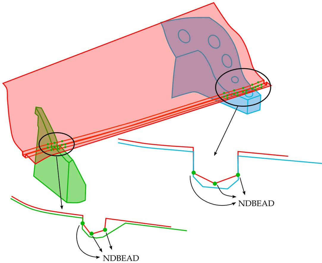
**Figure 12-35.** Definition of NDBEAD in the scrap trimming method. *Model courtesy of the Ford Motor Company.*
