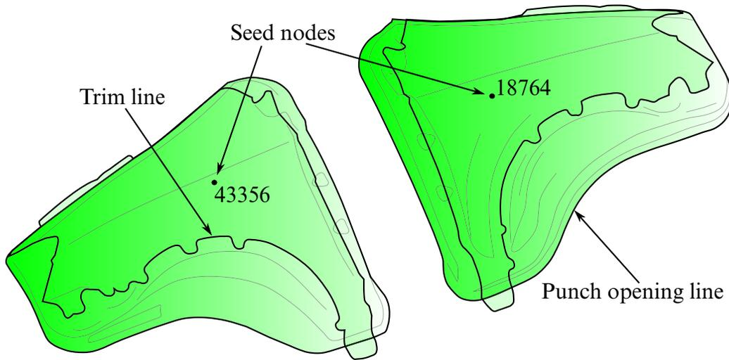
**Figure 15-18.** Trimming of a double-attached part (NUMISHEET2002 Fender Outer).
