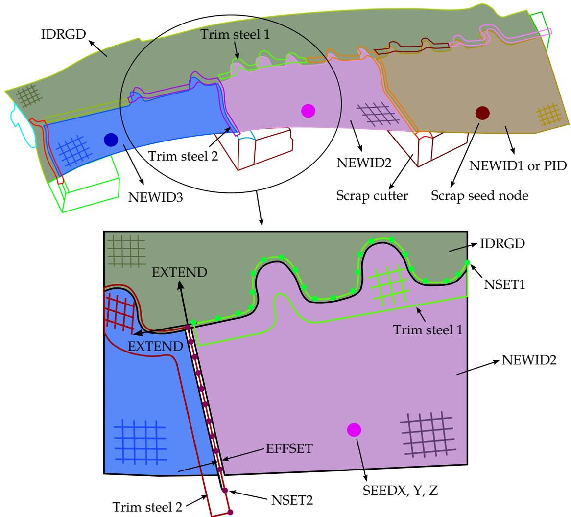
**Figure 12-34.** Trimming of multiple scraps and parameter definitions in the scrap trimming method. *Model courtesy of the Ford Motor Company.*
