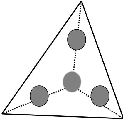
Example of discrete element sphere nodes for a tetrahedron element with  $NQ = 2$
