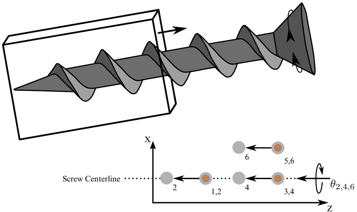
**Figure 10-26.** Screw joint. The second body translates in response to the spin of the first body. Nodal pairs (1, 3) and (2, 4) lie along the same axis and nodal pairs (1, 5) and (2, 6) are orthogonal vectors. The helix ratio,  $\dot{x}/\omega$ , is specified.
