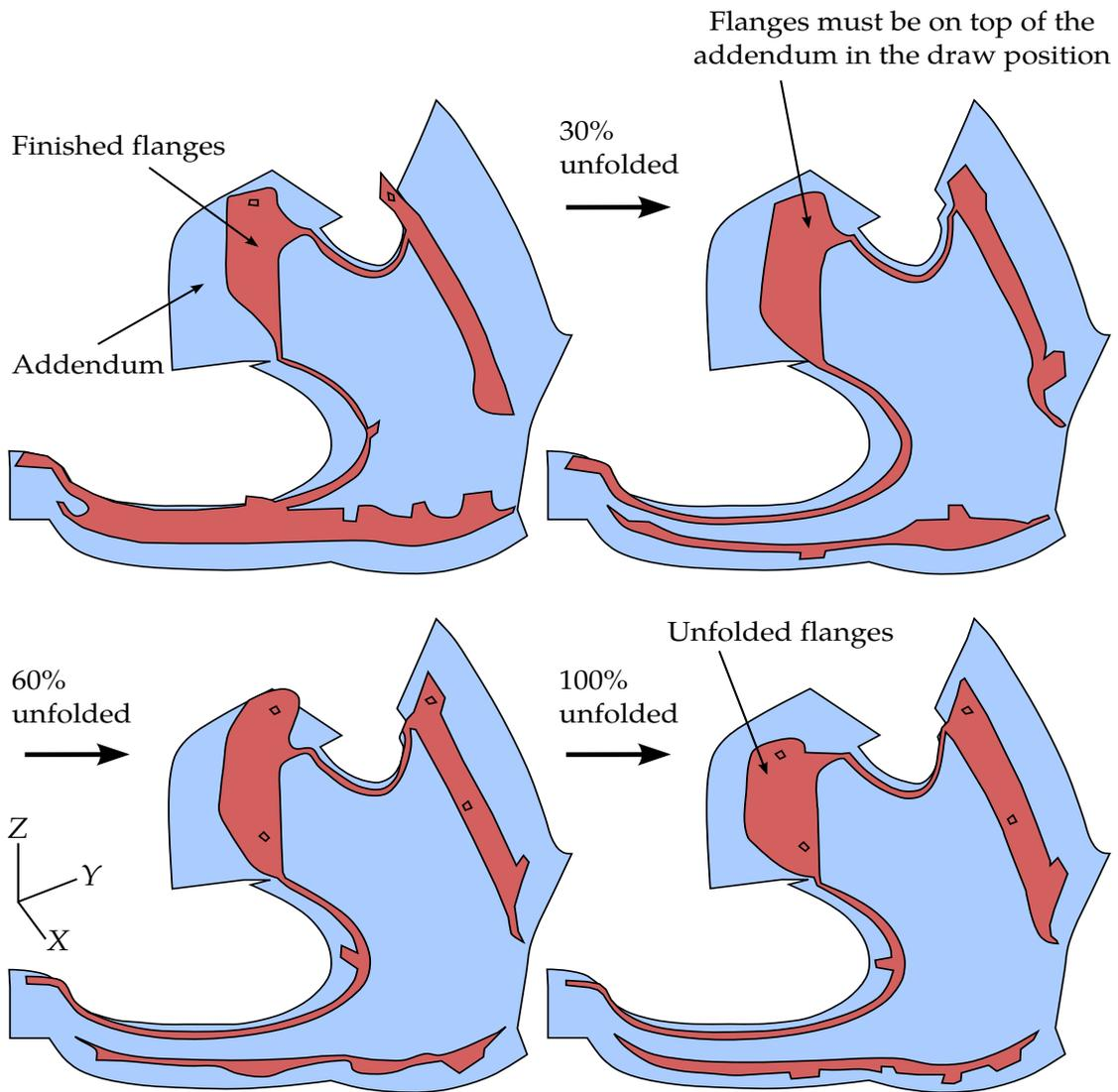
**Figure 12-47.** Flange unfolding progression of a fender outer (*original model courtesy of NCAC at George Washington University*).
