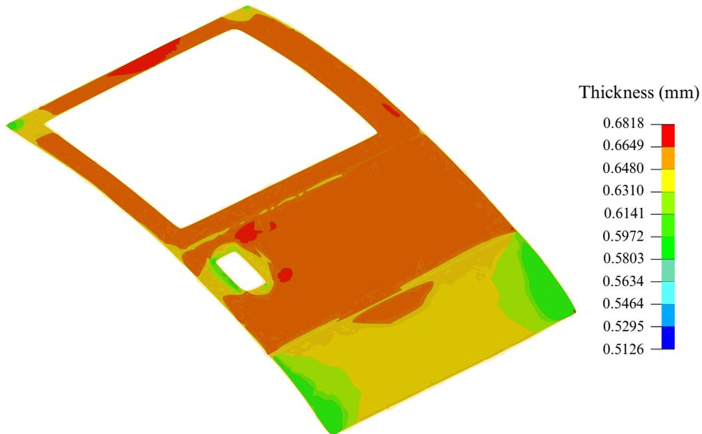
Figure 12-38. Thickness contour of the panel after trimming.
