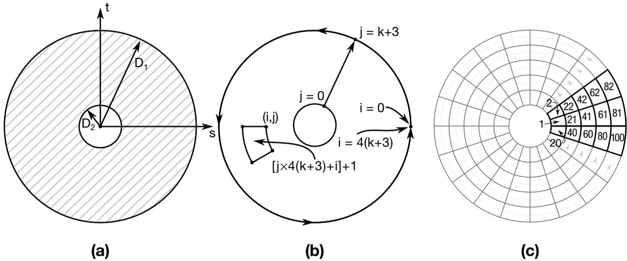
**Figure 24-11.** Type 9: Tubular. (a) Cross section geometry. (b) Integration point numbering. (c) Example for  $k = 2$ .
