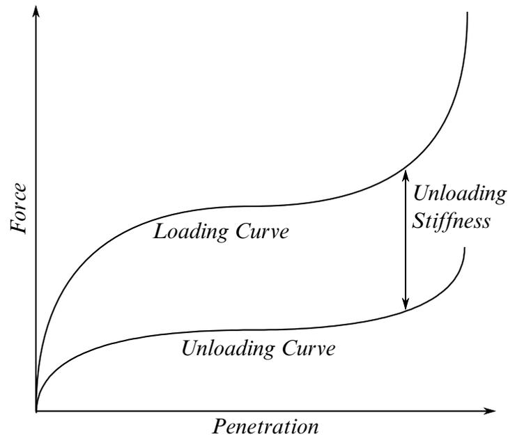
**Figure 11-10.** Behavior if an unloading curve is defined
