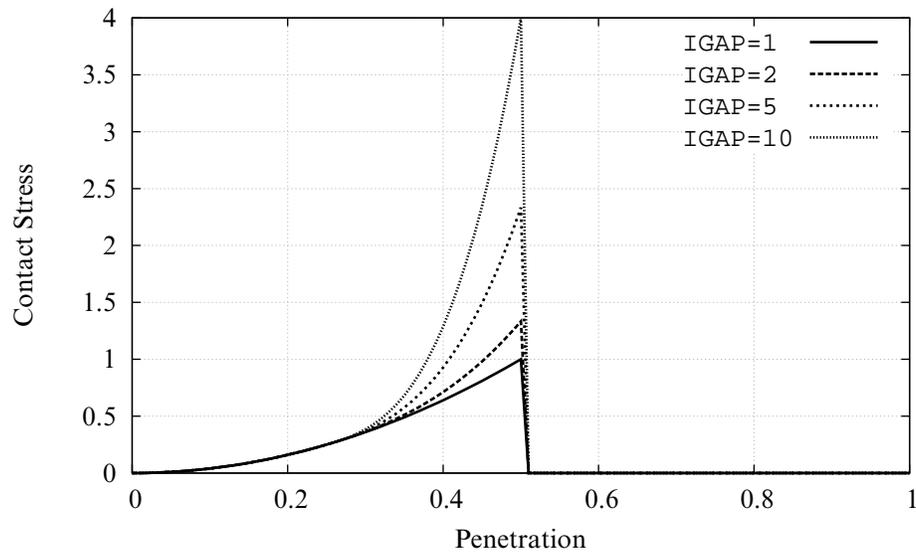
**Figure 11-15.** Mortar contact stress as function of penetration
