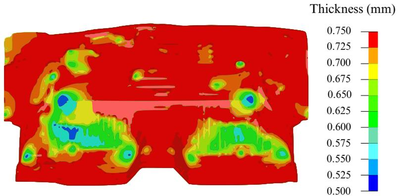
**Figure 12-15.** Shell thickness prediction ( $t_0 = 0.75\text{mm}$ ).
