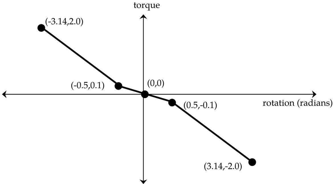
Figure 56-4 Characteristic torque curve shape used by all joints.
