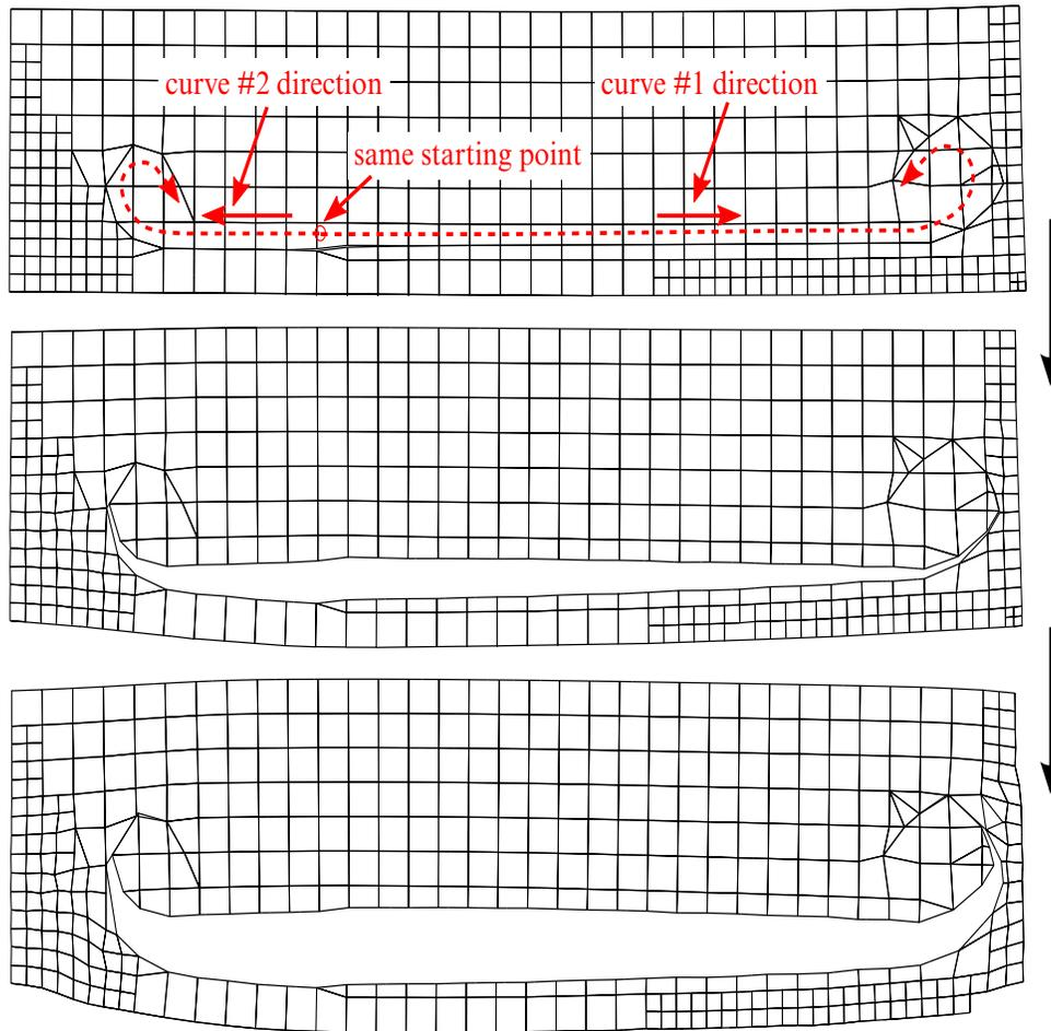
**Figure 18-12.** Progressive lancing – multiple lancing starting from the same coordinates.
