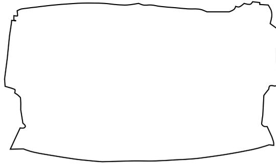
Figure 12-17. Initial blank size prediction (flat, not to scale).
