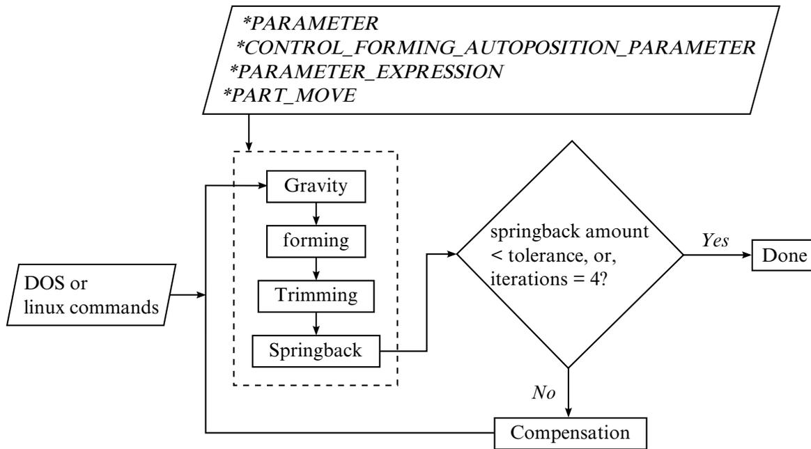
**Figure 25-25.** Iterative compensation flow chart
