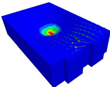
Thereby exploiting the Randles-circuit approach to describe the charging and discharging process as well as the accompanying heat production.
