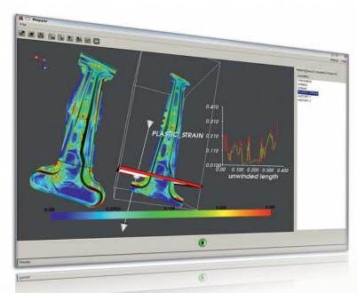
Typical B-Pillar Geometry — transfer of stamping results into a crash model
