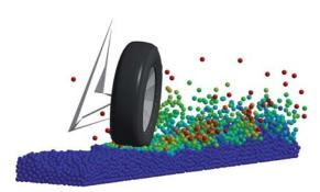
particles. Herein, the required mechanical behavior of the bonds is automatically computed by LS-DYNA using the parameters given in the material card. With the definition of a fracture energy release rate of the bonds, fracture mechanics of brittle materials can be studied.
