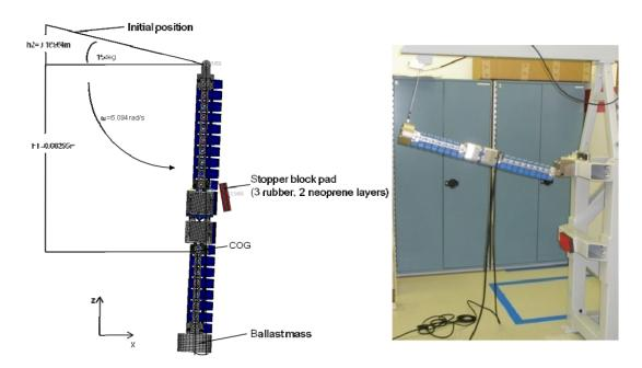
Figure 7: Assembly dynamic calibration setup
