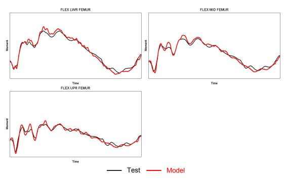
Figure 8: Assembly dynamic calibration femur moment results
