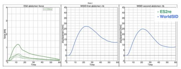
Figure 7: 3.0 m/s abdomen test; ES2re abdomen forces [kN] and WorldSID upper and lower abdomen rib deflection [mm] vs. Time [ms]
