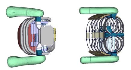
Below the clavicle/shoulder rib, both dummies consist of three thorax ribs. On the ES2re ribs a CONFOR® pink foam is tied on each single rib. The WorldSID ribs are covered with an ensolite foam pad which is only connected by a hook-and-loop fastener.
