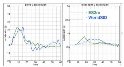
Figure 11: 4.0 m/s pelvis test; pelvis and lower spine acceleration [g] vs. Time [ms].
