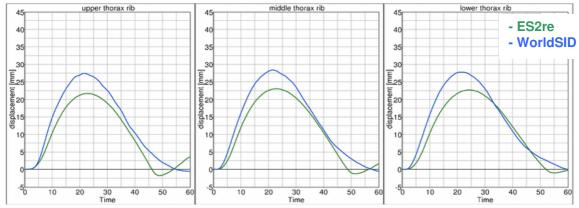
Figure 2: 3.0 m/s thorax test; upper, middle and lower thorax rib deflection [mm] vs. time [ms].
