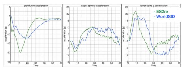
Figure 8: 4.3 m/s abdomen test; Pendulum, lower spine and upper spine acceleration [g] vs. Time [ms].
