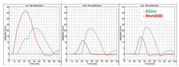
Figure 18: flat barrier 4 m/s; Upper, middle and lower thorax rib deflections [mm] vs. Time [ms].
