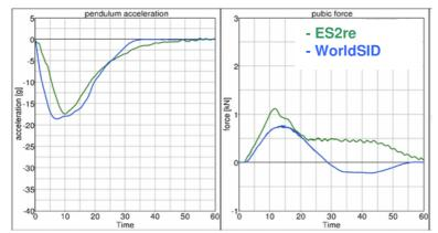
Figure 12: 4.0 m/s pelvis test; Pendulum acceleration [g] and pubic force [kN] vs. Time [ms].
