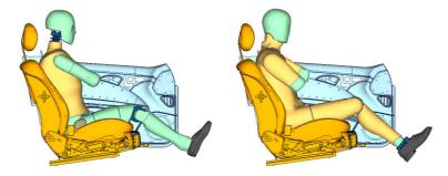
Figure 23: ES2re (left hand side) and WorldSID (right hand side) in vehicle with door trim and seat side view.
