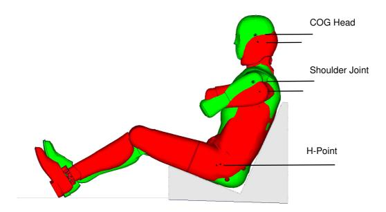
Figure 1: ES2re (green) and WorldSID (red) on WorldSID calibration bench.
