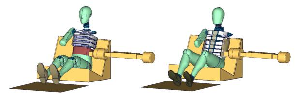
Figure 5: ES2re abdomen pendulum test (left hand side) and WorldSID abdomen pendulum test (right hand side)
