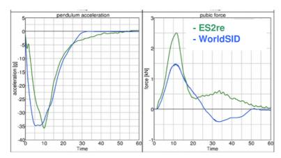
Figure 14: 6.7 m/s pelvis test; Pendulum acceleration [g] and pubic force [kN] vs. Time [ms].
