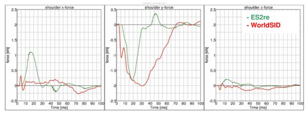
Figure 20: flat barrier 4 m/s; Shoulder force [kN] in x-, y- and z-direction vs. Time [ms].
