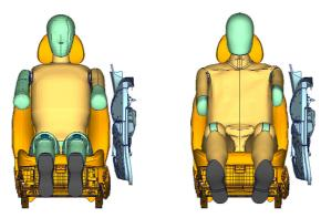
Figure 22: ES2re (left hand side) and WorldSID (right hand side) in vehicle with door trim and seat front view.
