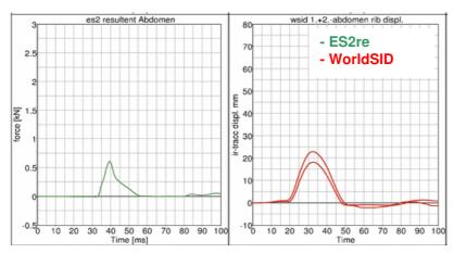
Figure 19: flat barrier 4 m/s; ES2re resultant abdomen force [kN] and WorldSID abdomen rib defections [mm] vs. Time [ms].
