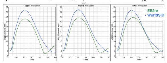
Figure 4: 4.3 m/s thorax test; upper, middle and lower thorax rib deflection [mm] vs. time [ms].
