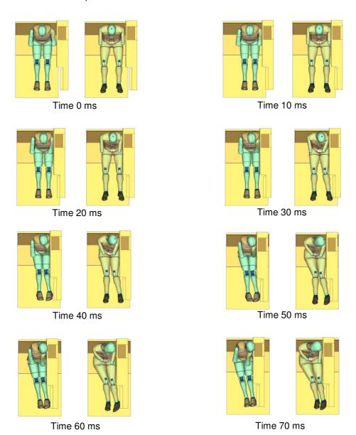
Figure 21: flat barrier 4 m/s; left hand side ES2re, right hand side WorldSID for times 0 - 70 ms
