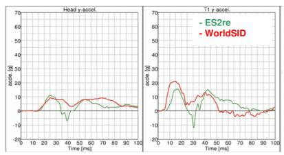
Figure 16: flat barrier 4 m/s; Head and T1 y-acceleration [g] vs. Time [ms].
