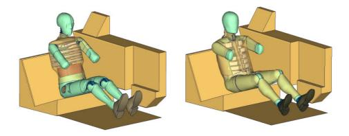
Figure 15: ES2re (left hand side) and WorldSID (right hand side) sled test with flat barrier and 4 m/s.
