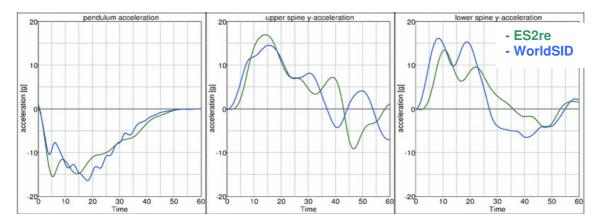
Figure 3: 4.3 m/s thorax test; pendulum, upper spine and lower spine accelerations [g] vs. time [ms].
