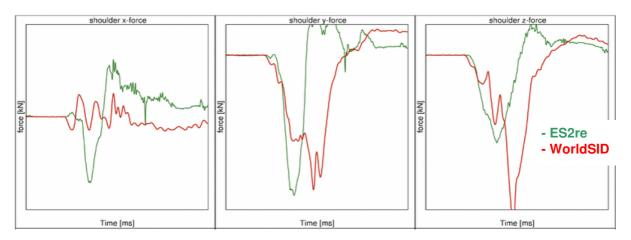
Figure 25: vehicle oblique pole; Shoulder force [kN] in x-, y- and z-direction vs. Time [ms].
