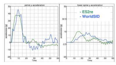
Figure 13: 6.7 m/s pelvis test; Pelvis and lower spine acceleration [g] vs. Time [ms].
