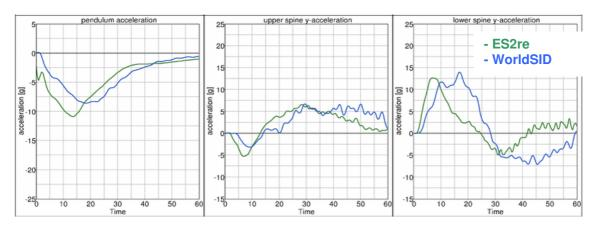
Figure 6: 3.0 m/s abdomen test; Pendulum, lower spine and upper spine acceleration [g] vs. Time [ms].
