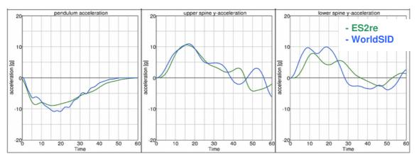
Figure 1: 3.0 m/s thorax test; pendulum, upper spine and lower spine accelerations [g] vs. time [ms].
