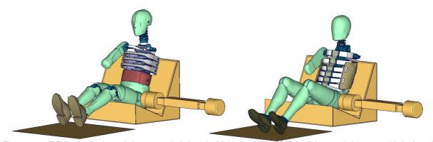
Figure 10: ES2re pelvis pendulum test (left hand side) and WorldSID pelvis pendulum test (right hand side)
