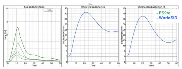
Figure 9: 4.3 m/s abdomen test; ES2re abdomen forces [kN] and WorldSID upper and lower abdomen rib deflection [mm] vs. Time [ms]
