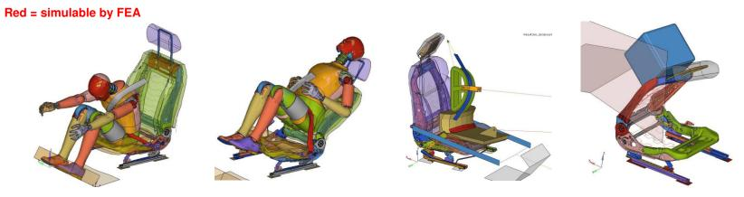
Different materials behaviors : Steels / Foams / Plastics Different modeling scales : seat frame / seat mechanisms Integration of restraint systems Integration of dummies
