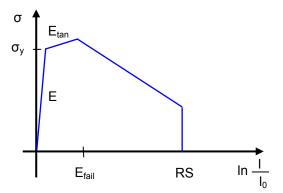
Fig. 13: Stress-Strain relationship for bolt material
