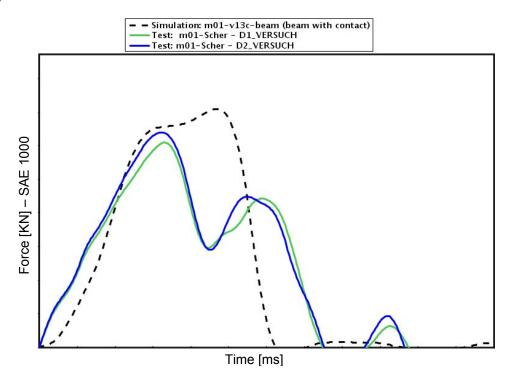
Fig. 16: Reaction force for dynamic test with bolt failure
