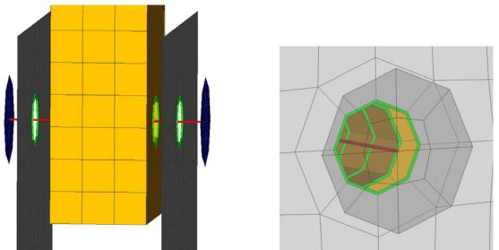
Fig. 4: Modelling of bolt with spotweld-beams and contact beams on hole edge
