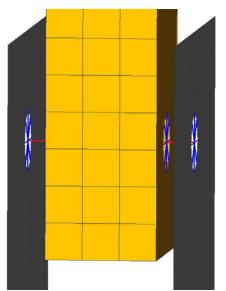
Fig. 1: Modelling of bolt with beams (elform=1) and connection through spider mesh
