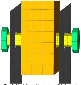
Fig. 2: Modelling of bolt with solid elements
