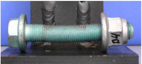
Fig. 15: Bolt after dynamic load without failure
