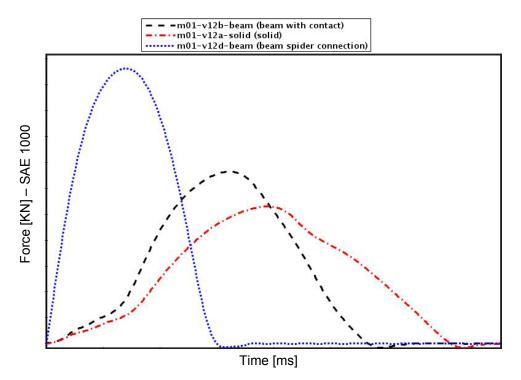
Fig. 9: Comparison of the reaction force for three modeling types
