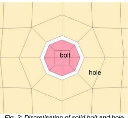
Fig. 3: Discretisation of solid bolt and hole
