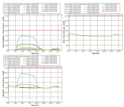
Fig. 7: Example for postprocessing of a bolt which is modelled with beam pieces
