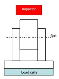
Fig. 11: Test configuration
