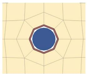
Fig. 5: Discretisation of beam bolt (3d-illustration) and contact beams around the hole
