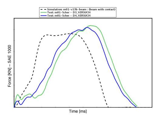
Fig. 14: Reaction force for dynamic test without bolt failure
