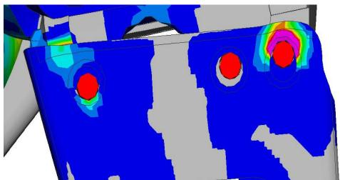
Fig. 6: Bearing stress with spotweld-beams for bolt-shank and contact beams around the hole
