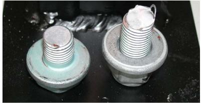
Fig. 17: Bolt after dynamic load with failure
