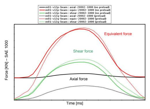
Fig. 10: Influence of preload in double shear model
