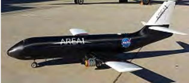
NASA is developing and validating a system that will allow part of an aircraft's wing to fold in flight to increase efficiency through wing adaptation.
