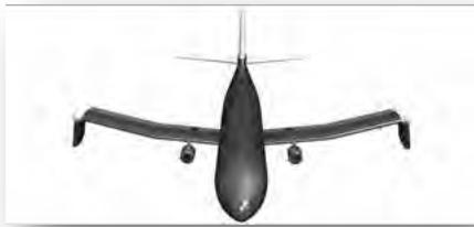
The Spanwise Adaptive Wing concept seeks to enhance aircraft performance through allowing the outboard portions of wings to adapt, or fold, according to different flight condition demands. NASA engineers believe this could create lateral-directional stability and reduce drag.
