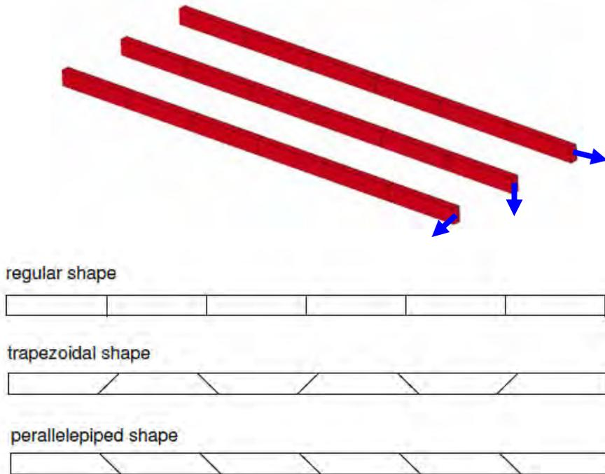
**Figure 2 Straight cantilever beam test. Loading: unit forces at free end**
