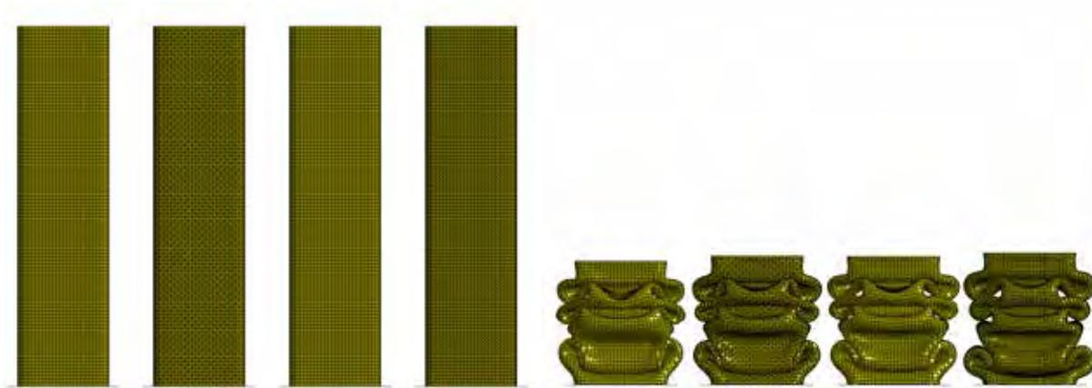
Figure 12 Initial and deformed model for hex, tet and penta element
