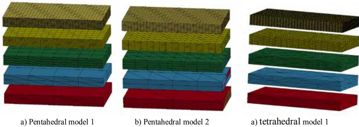
**Figure 8 Clamped plate subjected torque, pentahedral and tetrahedral model**
