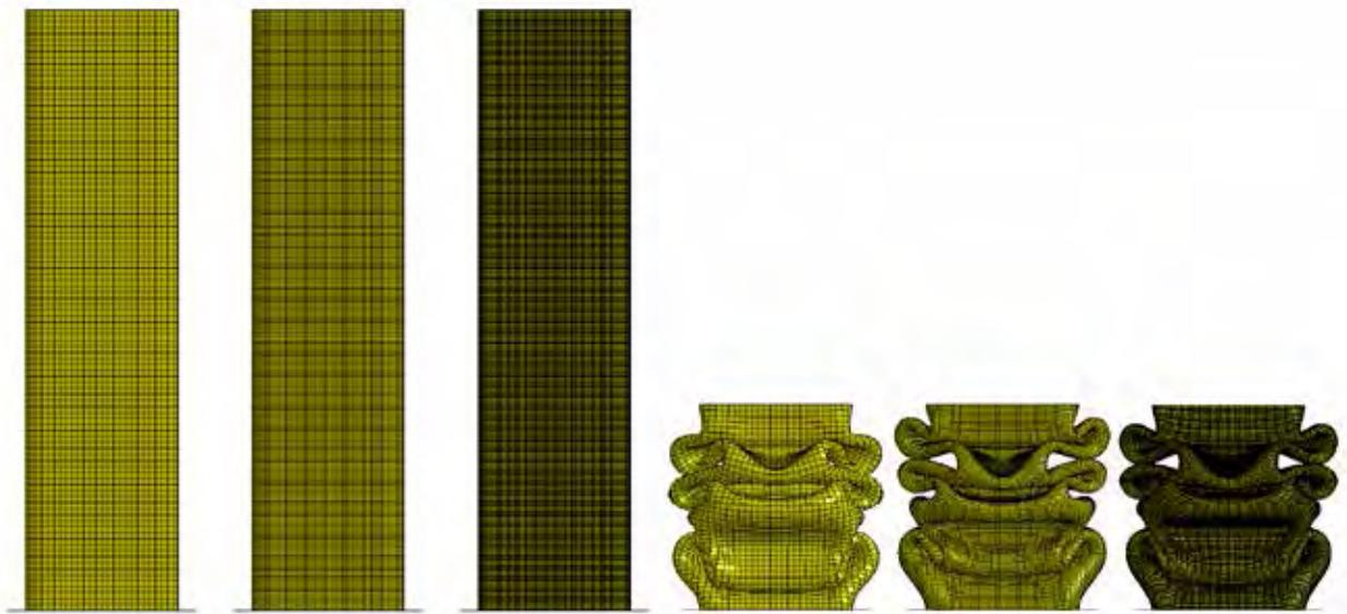
Figure 10 Initial and deformed model with 4mm, 2mm, and 1mm mesh
