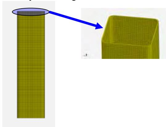
**Figure 9 Model set up for crush box, one layer of mesh over thickness**
