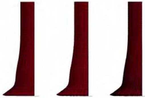
**Figure 5 Deformed model for bar impact problem using a) 972 Elform2 element b) 972 Elform24 Element c) 7776 Elform2 element**
