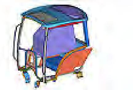
Fig. 2 CAD model of the tractor showing the protective structure FOPS
