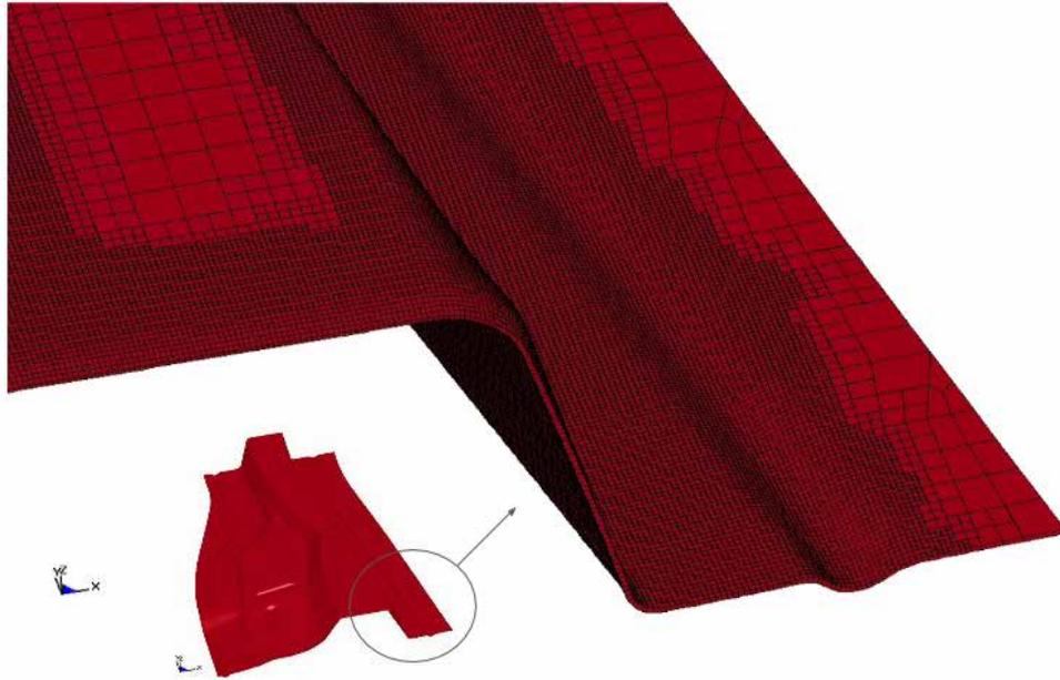
Figure 3. Adaptive mesh refinement of laminates (2005 NUMISHEET Crossmember).
