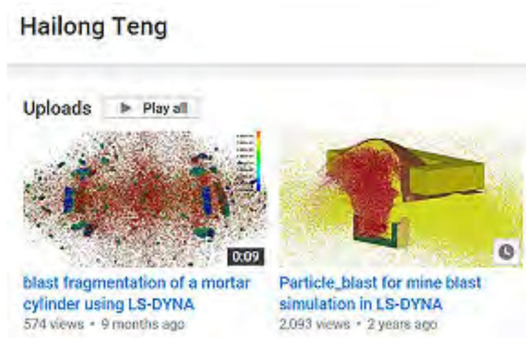
The Particle Blast Method (PBM) was employed to model the behavior of the detonation the bonded DEM was used to model the mortar cylinder , for more information, please refer to [http://www.fragblast11.org/Media/Fragblast11/presentations/SESSION\\_10A\\_1150.pdf](http://www.fragblast11.org/Media/Fragblast11/presentations/SESSION_10A_1150.pdf)
