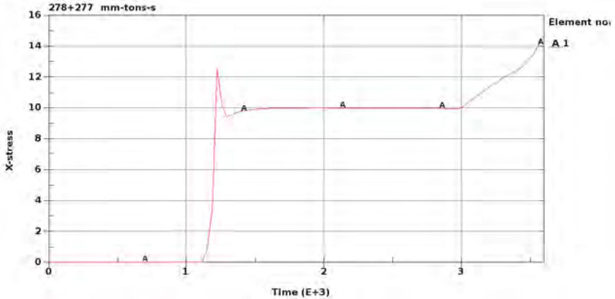
Figure 8 Stress in XX direction during tension and curing test
