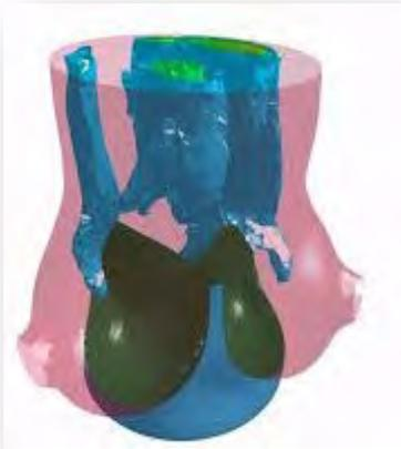
**The LS-DYNA® ICFD solver can be used to solve complex multi-physic problems that include behavior of a heart valve.**
