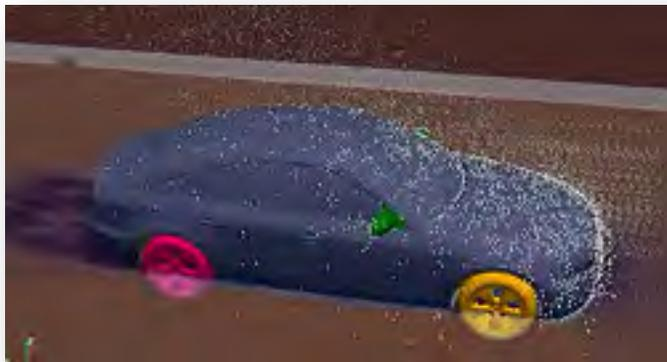
**Snow accumulation on vehicle using ICFD solver and DEM coupling (LS-DYNA R9)**
