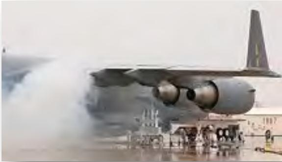
Oil smoke billows from the right inboard engine of the C-17, while a probe collects emissions data, during engine health monitoring tests that resume this week when ash will be fed into an engine.
