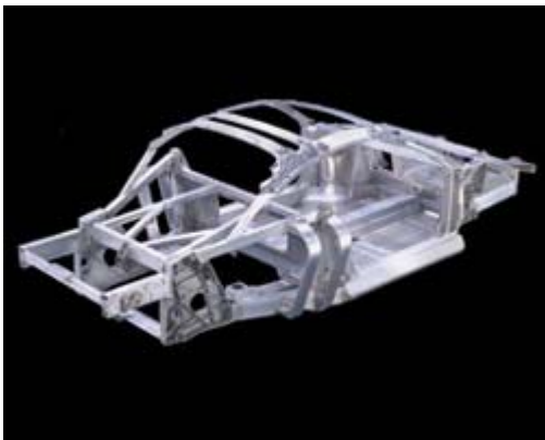
Figure 2: Aluminum spaceframe for the Ferrari 360 Modena.
