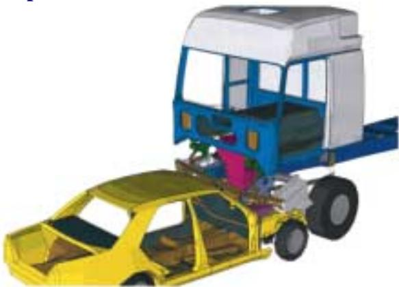
Impact of a passenger car (W124) with 60 km/h relative velocity.
