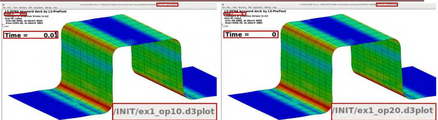
Fig.6: Von Mises Stress distribution: end of stage 1 (op10 - left) and beginning of stage 2 (op20 -right)
