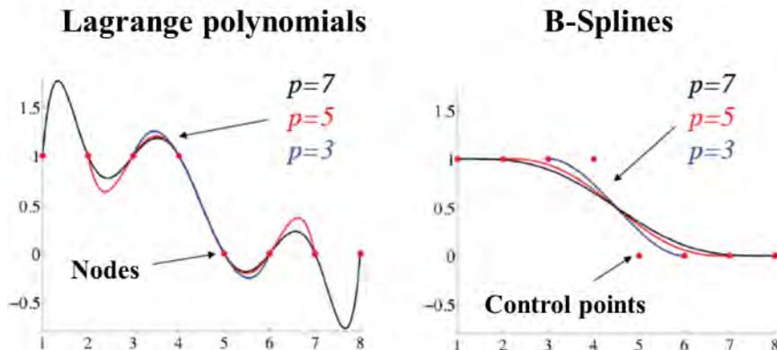
Fig.2: Comparison of Curves represented by Lagrange polynomials (left) and B-spline basis functions(right)given the same set of nodes and control points, respectively [3]
