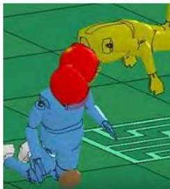
In this case, using a sample helmet mesh, Dilip Bhalsod of LSTC used that helmet mesh with some standard LSTC automotive dummy models to create [\*\*a proof-of-concept collision between two football players.\*\*](#)
