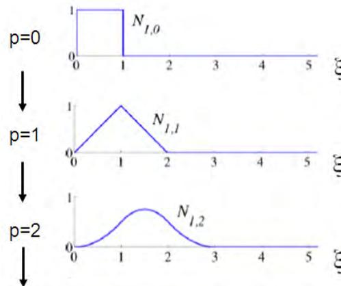
Fig.1: B-spline basis functions of order 0, 1 and 2 for uniform knot vector [3]
