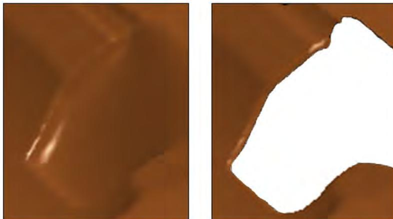
Fig.7: A deformed shell NURBS patch before (left) and after trimming (right)
