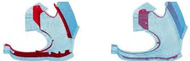
Accurate un-flanging simulation for trimming curve development
