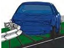
**Numerical simulation of a TB32 crash.** Impact conditions as prescribed by the norm EN1317 ( 110 Km/h - 20°) using LS-DYNA. Performed at GDTech SA, Liège Belgium.
