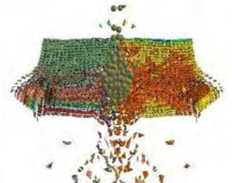
Bird striking CFRP laminate (SPH-Peridynamics)
