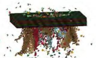
Ball impact on CFRP (Peridynamics)
