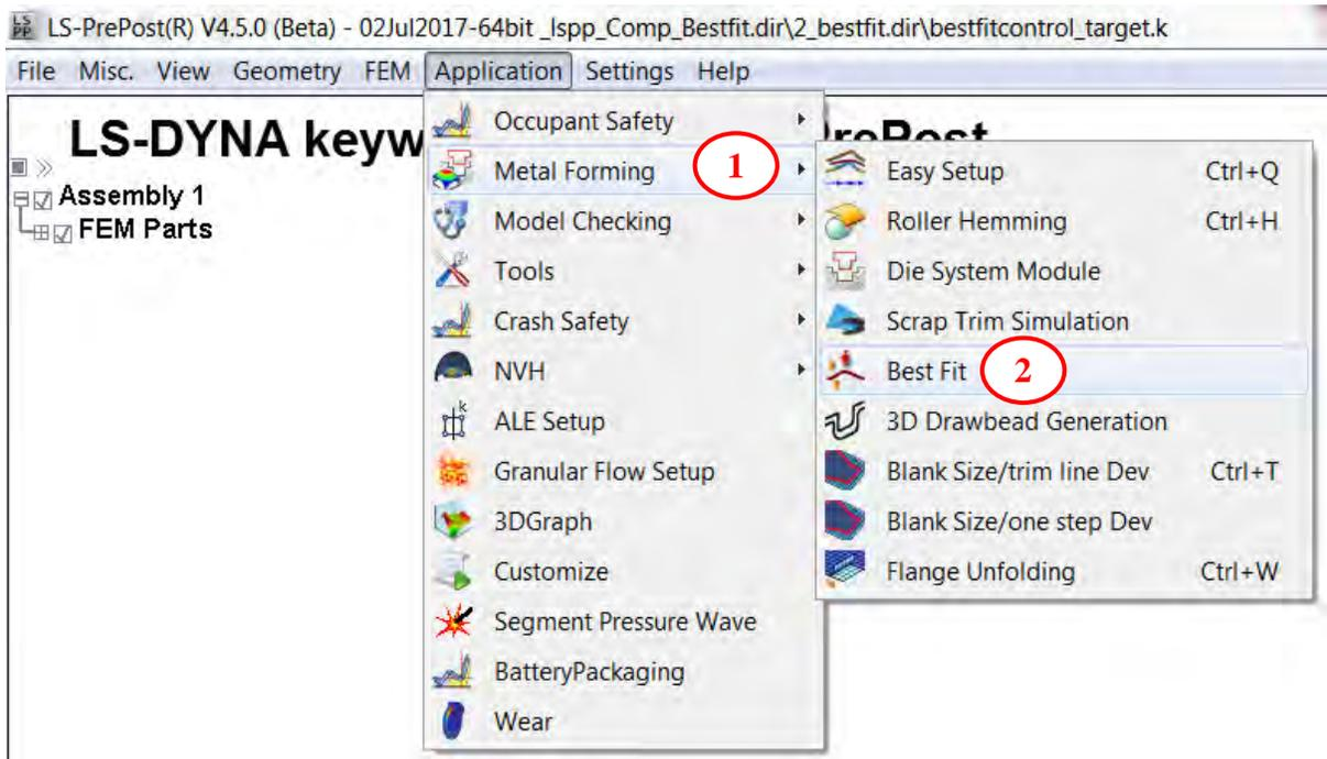
Figure 1. Activating the Best Fit GUI in LS-PrePost 4.5
