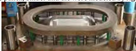
Fig. 7. Experimental setup for the double dome test.
