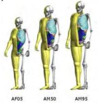
The internal organs were modeled based on high resolution CT-scans.
