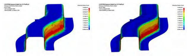
(a) No Fission (b) With Fission Figure 3. Effective plastic strains of the solid at the end of the forming processes, with and without adaptive fission. The solid is discretized into one layer of hexahedral elements.
