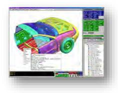
The Oasys PRIMER pre-processor is designed to make preparation and modification of LS-DYNA models as fast and as simple as possible, improving user productivity and efficiency and reducing the time spent manipulating and developing models suitable for LS-DYNA.
