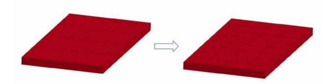
Figure 1. Mesh Fission for Sandwich Structure Part: 32 hexahedral elements are refined to 128 of the same type, as a sweeping of the top and bottom adaptive shell elements through the thickness. The number of layers of the solids always remains the same.
