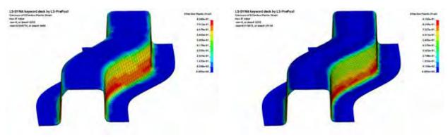
(a) No Fission (b) With Fission Figure 4. Effective plastic strains of the solid at the end of the forming processes, with and without adaptive fission. The solid is discretized into three layers of hexahedral elements.
