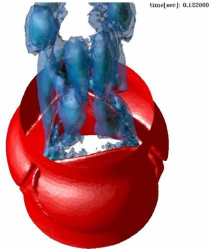
The above is an FSI problem of a opening valve and the flow is shown and maximum aperture when the flow rate peaks. In both cases the turbulence was modeled using a LES approach.
