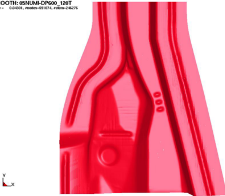
Figure 7 Numisheet'05 Automotive Underbody Cross Member
