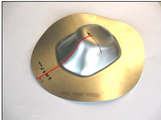
Figure 14. The end-cap drawn to 47 mm with the thickness distribution measurement line.
