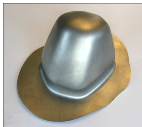
Figure 13. A fully formed exhaust end-cap.
