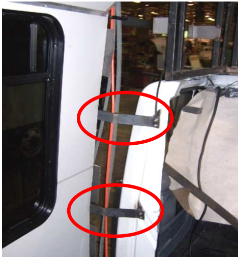
Figure 5: Connection of bus body to driver's cabin road side
