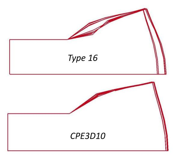
Overlays of the different meshes for 50% compression
