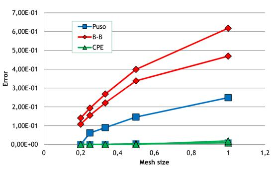
Cosserat Point Element is much less mesh sensitive than Belytschko-Bindeman and Puso elements
