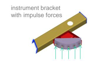
transient explicit: 220 min (single precision) transient non-linear implicit: 265 min transient modal dynamics: 4 min
