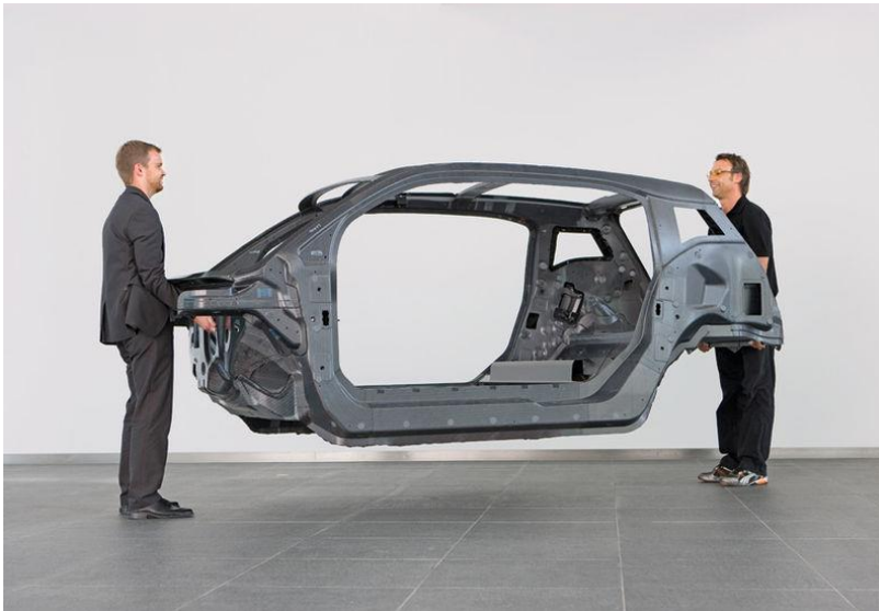
BMW's i3 carbon fiber composite passenger cell (Image courtesy of auto-motor-und-sport.de)
