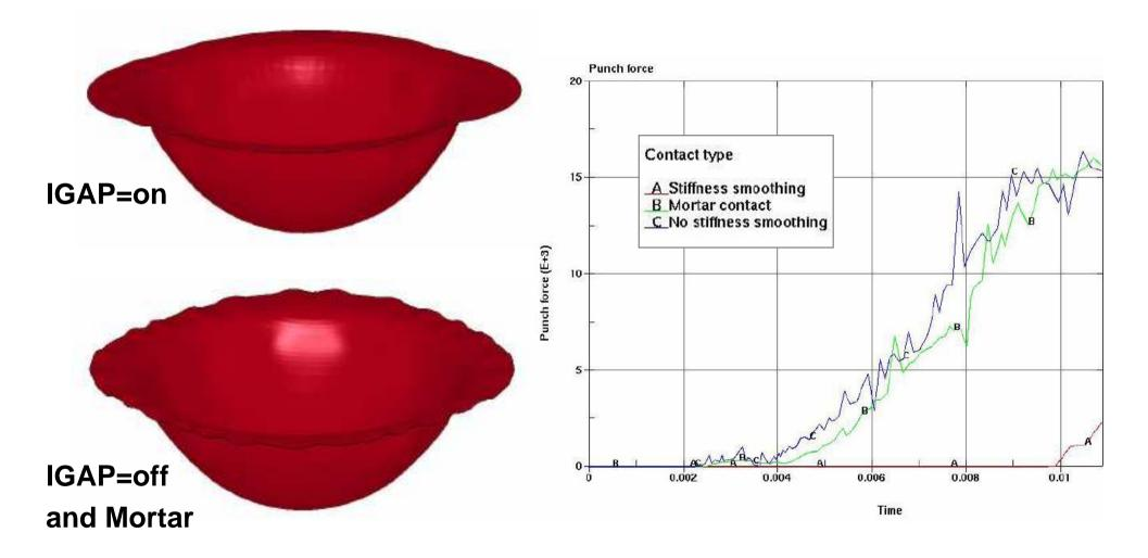
Normalized CPU times: IGAP=on: 1.0, IGAP=off: 3.1, Mortar: 2.2
