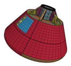
Free fall impact / Strong FSI coupling Proof of feasibility using ICFD solver May be applied to similar Slamming problems
