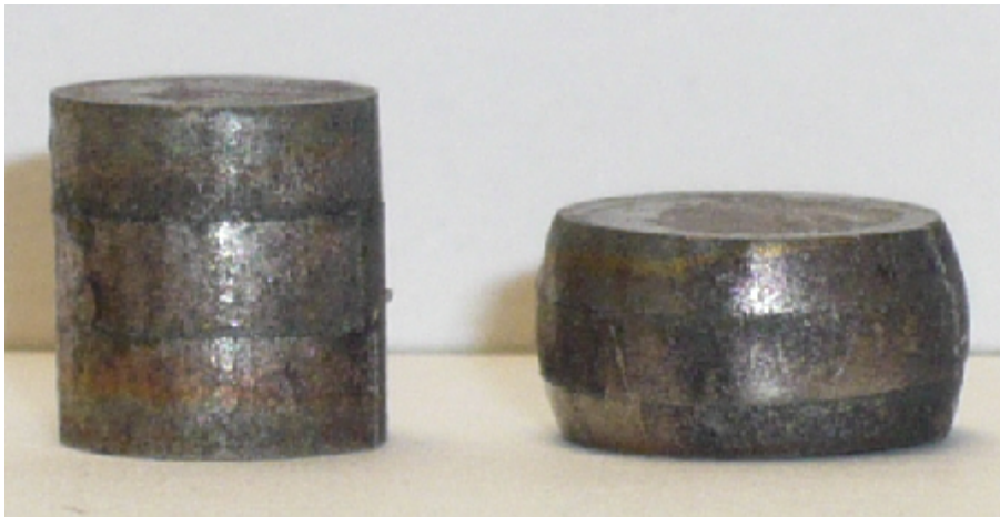
Figure 6: Undeformed and deformed specimen.
