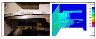
Figure 19 Buckling of gusset plate
