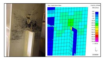
Figure 11 Column Stiffener Plate Yielding
