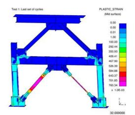
Figure 9 Plastic Strain at end of fourth set of cycles
