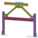
Figure 15 Intermediate Stage: Frame with braces removed
