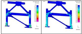
Figure 18 Initial Stresses and Plastic Strains for Test 2
