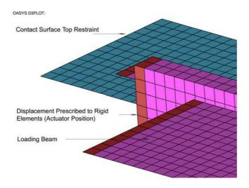
Figure 2 Contact Surface/Loading Beam Detail
