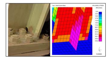
Figure 6 Column Stiffener Plate Yielding
