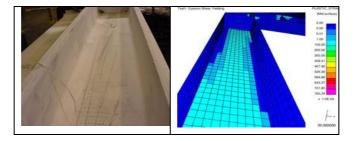
Figure 10 Column Shear Yielding
