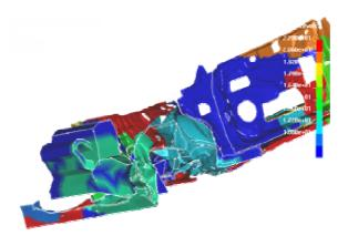
**Figure 8**: The SIMCluster functional shows areas of similar scatter on the body of the Neon model. All nodes of such an area share the same source of instability.
