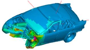
**Figure 3:** PD3MX as color coding on the BMW test case showing differences of more than 10 cm between several runs.
