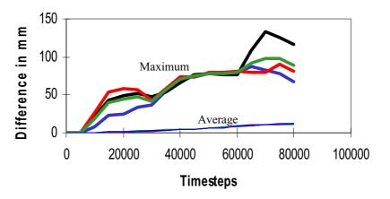
**Figure 1** Difference between several simulation runs of a BMW model after a 40% offset crash using PAM-CRASH on a 32 node IBM SP2 using the same input deck
