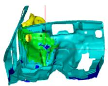
Figure 10: SIMCluster function for the BMW model at 80 ms identifies two clusters, each of which has the same reason for instability.
