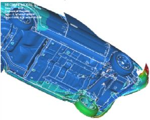
**Figure 4:** PD3MX as color coding on the Neon testcase showing differences of up to 10 cm in node positions between different simulation runs.
