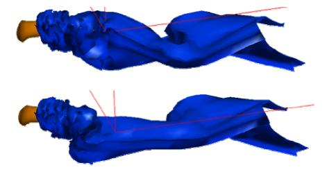
Figure 12: Two different modes of the crash behaviour of the longitudinal rail.
