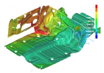
**Figure 7**: PD3MX as color coding on the footarea of the Neon Model showing scatter of simulation results of more than 3 cm at 114 ms.
