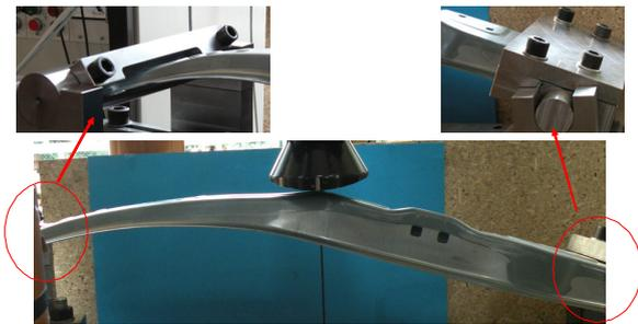
Fig. 12: Test set up for bending test with superimposed tension on a component
