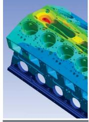
Deformation contours on an engine block, courtesy of ANSYS, Inc.
