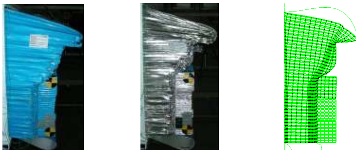
Figure 11: Deformed barriers test 1, 2 and simulation;
