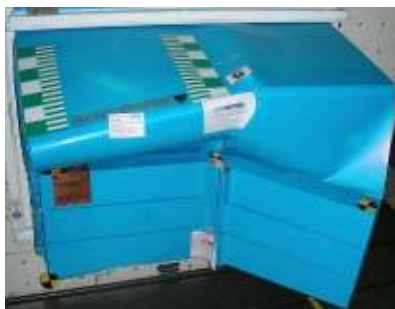
Figure 14: Deformed barriers test 5 and simulation;
