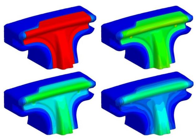
Fig.11: fringe plot of temperature in tool and blank during one cycle
