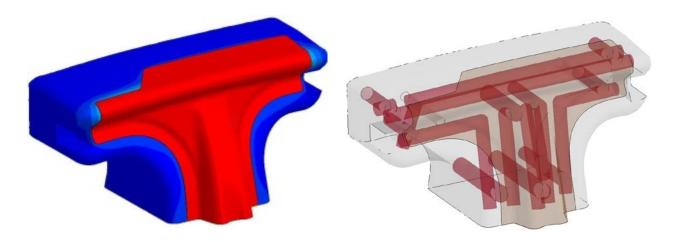
Fig.7: punch segment 4 with blank (red); left image shows a fringe plot of temperature at time t=0; right image shows the geometry of tool and blank in transparent mode
