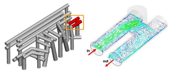
Fig.3: u-bend section of punch segment 1 (left) and vector plot of velocity (right)
