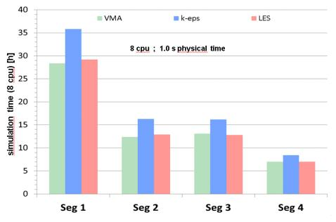
Fig.6: simulations with different turbulence models; comparison of runtimes (same mesh size
