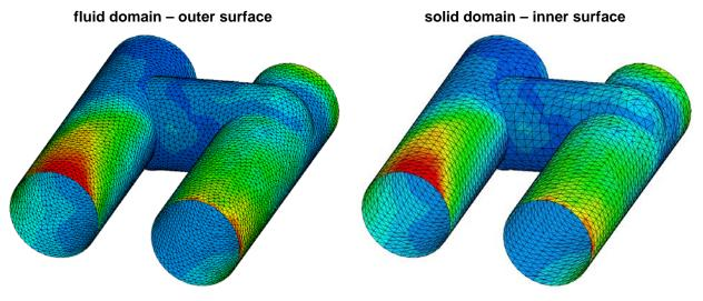
Fig.8: coupling: mesh and temperature distribution on the common boundary
