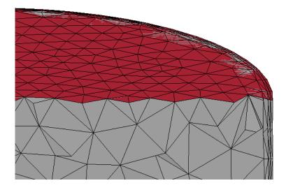
Fig.9: section of the automatically generated volume mesh of the fluid with boundary layer resolution
