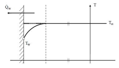
Fig.10: temperature distribution in the fluid near a solid wall
